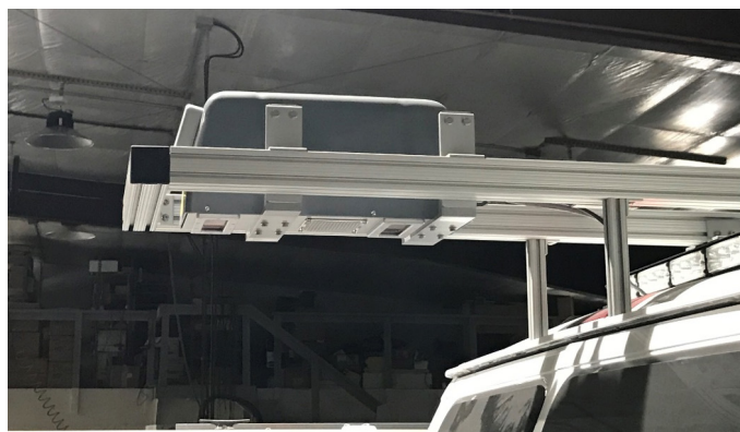
Figure 2. Photograph. Close-up view of an ATPMS.
