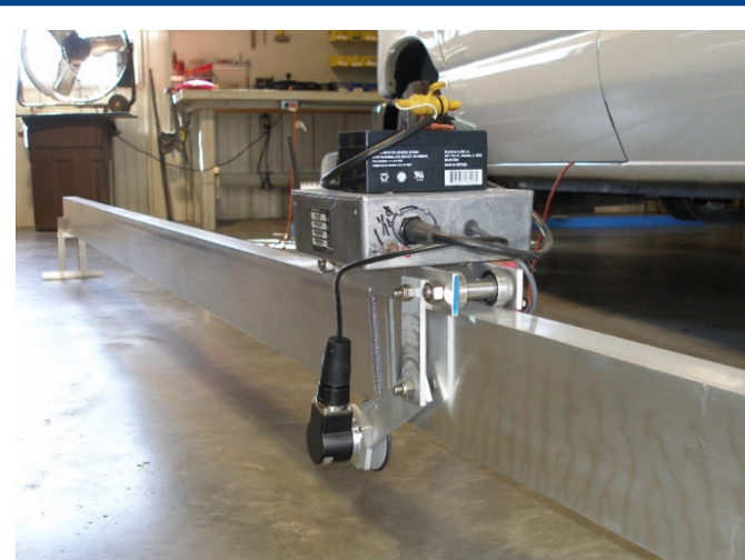
Figure 4. Photograph. Reference device that collected reference transverse profile data.
