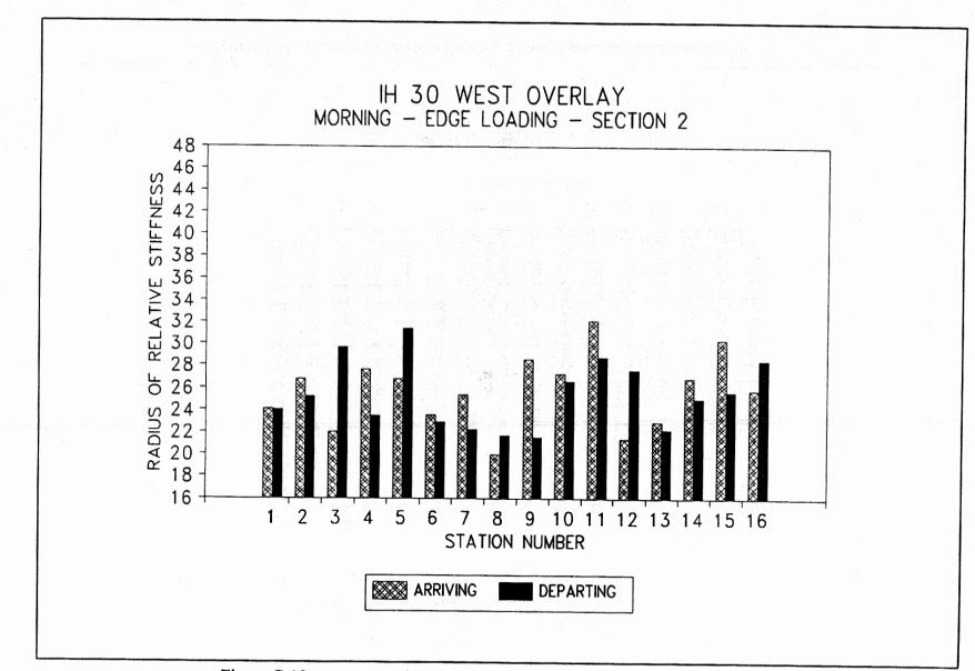
Figure C-10. *l* versus station (I-30W, overlay, morning, edge, section 2).
