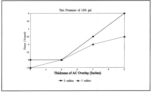
Figure 50. Time for AC overlay to rut 7.6 mm (0.3 in).
