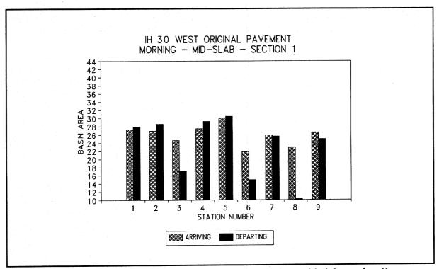
Figure 33. Basin area versus station (I-30W, morning, mid-slab, section 1).
