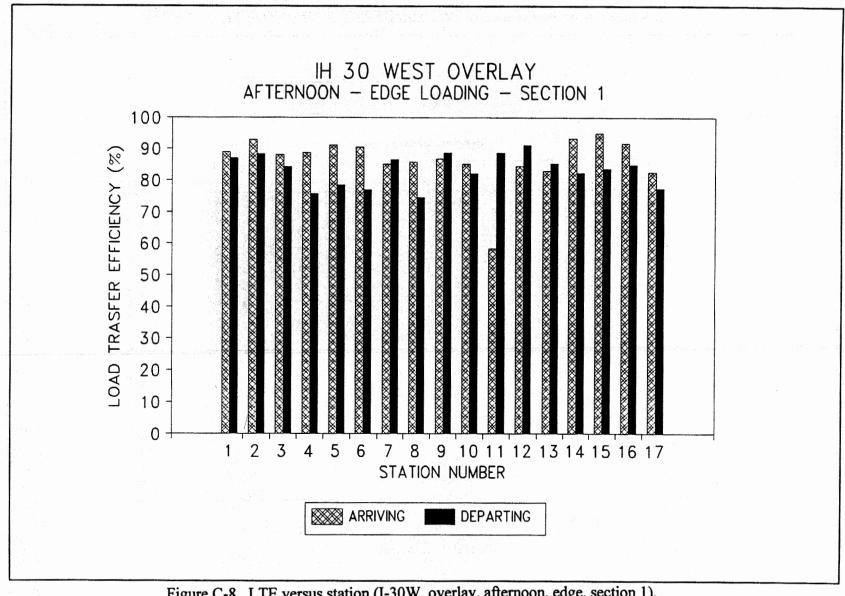
Figure C-8. LTE versus station (I-30W, overlay, afternoon, edge, section 1).
