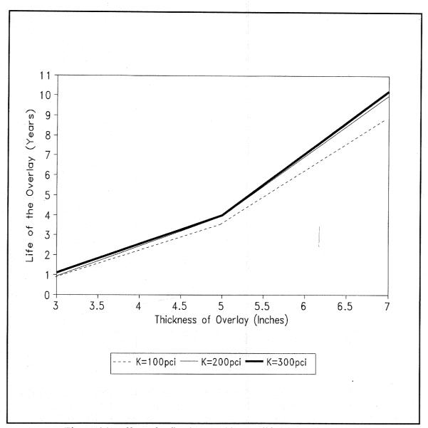
Figure 46. Effect of reflective cracking on life of the AC overlay as a function of different subgrade moduli.
