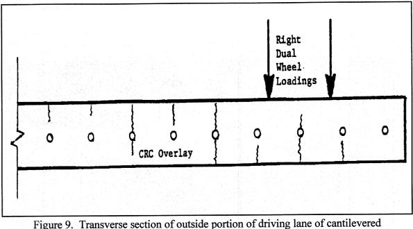
CRC overlay illustrating formation of longitudinal cracks along planes of rebars in tension zones of the concrete.<sup>(37)</sup>
