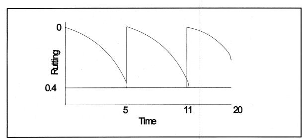
Figure 51. Rutting life of an AC overlay.
