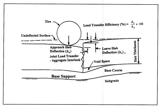
Figure 17. Load transfer efficiency.<sup>(51)</sup>
