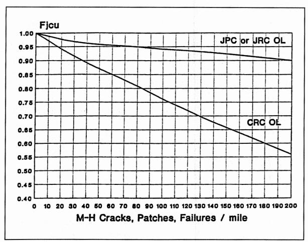
1 mi = 1.7 kmFigure 14. Adjustment factor for the design of jointed and CRC unbonded overlays.<sup>(53)</sup>
