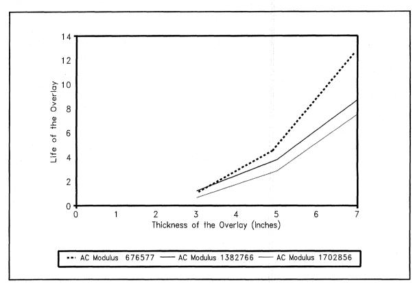
Figure 45. Effect of reflective cracking on life of AC overlay as a function of different moduli of AC.
