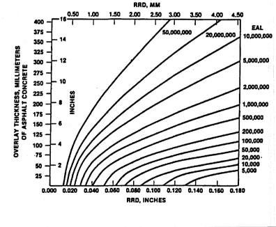
Figure 5. AC overlay thickness required to reduce pavement deflection value (rebound test).<sup>(18)</sup>
