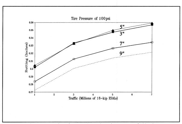
Figure 49. Rutting of AC overlay under a tire pressure of 100 psi.
