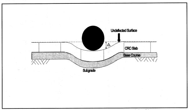
Figure 16. Shape of the deflection basin under a slab of low stiffness and strong subgrade support.
