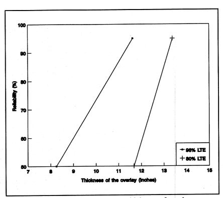
Figure 34. Reliability versus thickness of overlay.
