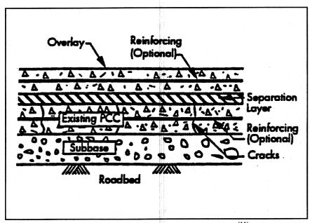
Figure 1. Unbonded concrete overlay.<sup>(11)</sup>
