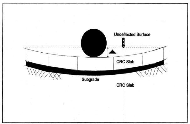
Figure 15. Shape of the deflection basin under a slab of high stiffness and weak subgrade support.
