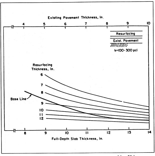
1 in = 25.4 mm Figure A-5. PCC overlay design chart for case 2 condition of existing pavement.<sup>(48)</sup>
