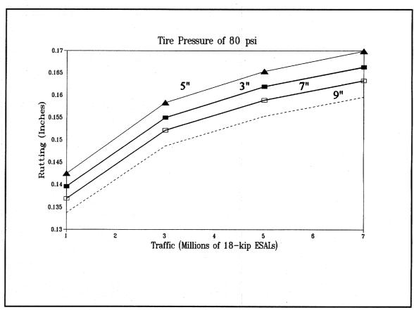
Figure 48. Rutting of AC overlay under a tire pressure of 80 psi.
