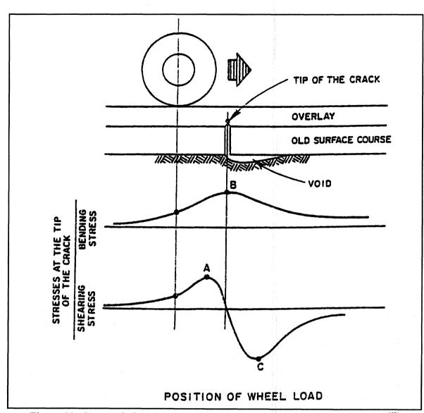
Figure 44. Stresses induced at the cracked section due to a moving wheel load.<sup>(62)</sup>
