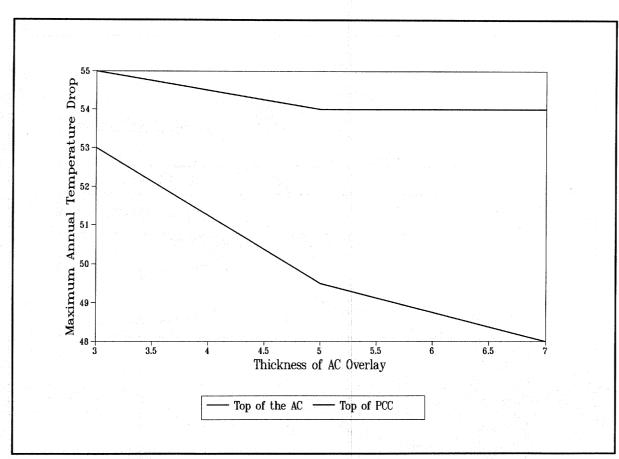
Figure 43. Temperature variations at the surface of AC overlay and PCC surface.
