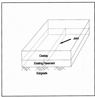
Figure 21. Section of the existing slab.
