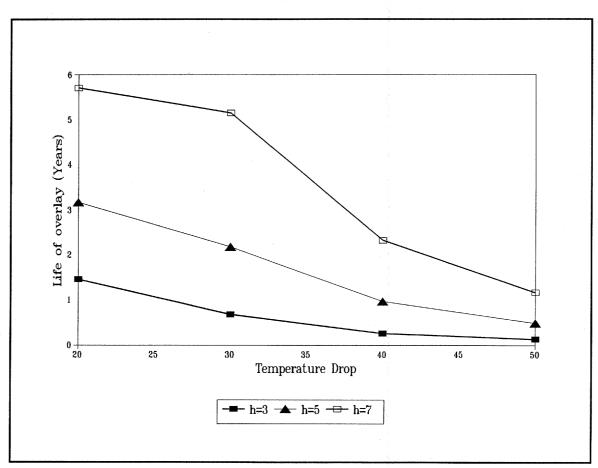
Figure 47. Effect of reflective cracking on life of the overlay as a function of different daily drops in temperature.
