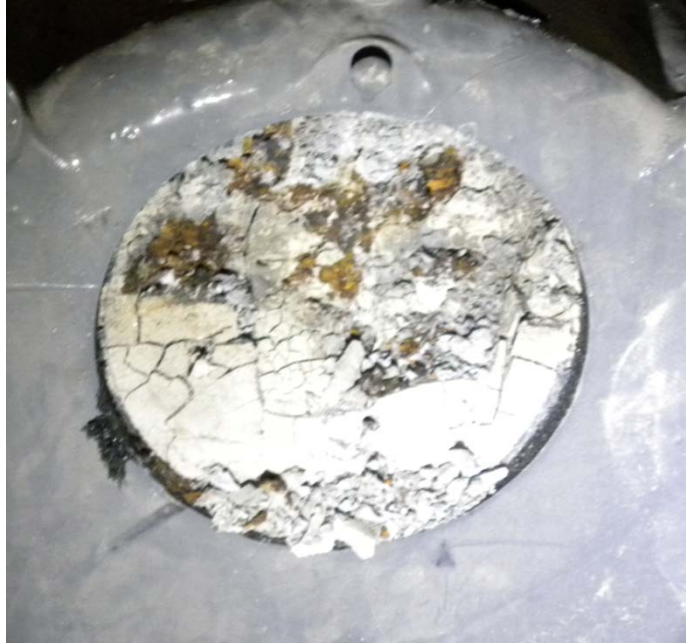
Figure 30. Photo. Opened tendon end showing predominantly type 3 grout and strand corrosion products.
