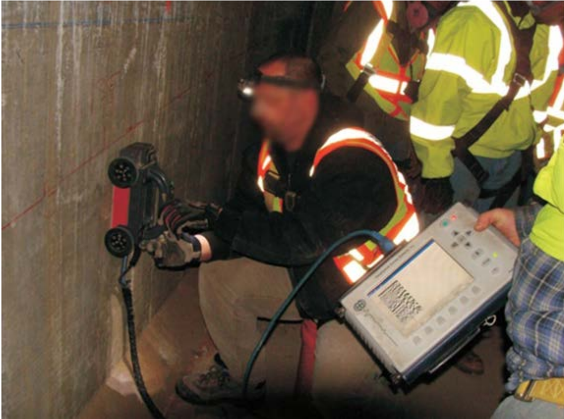
Figure 64. Photo. Locating internal tendons in the web wall using GPR.
