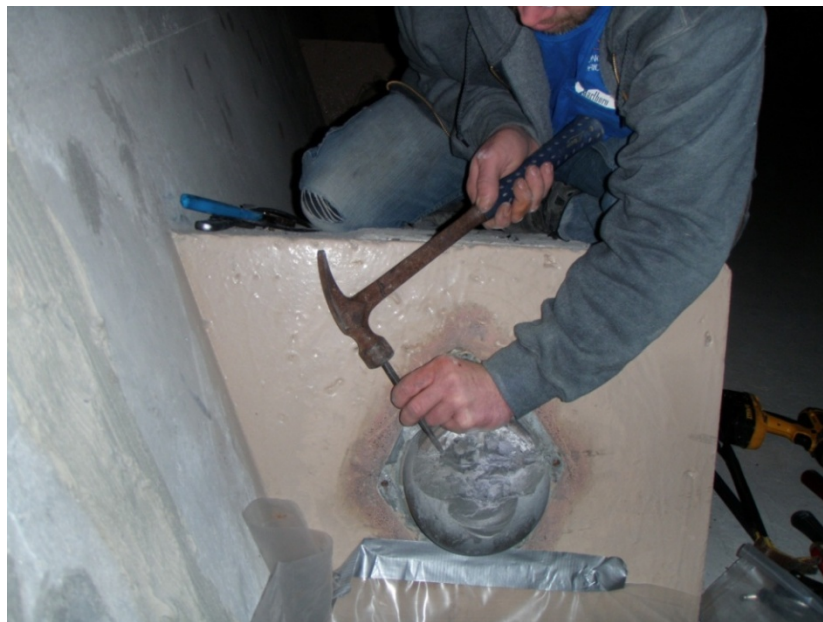
Figure 54. Photo. Grout sample acquisition at an opened internal tendon end cap by light chipping.
