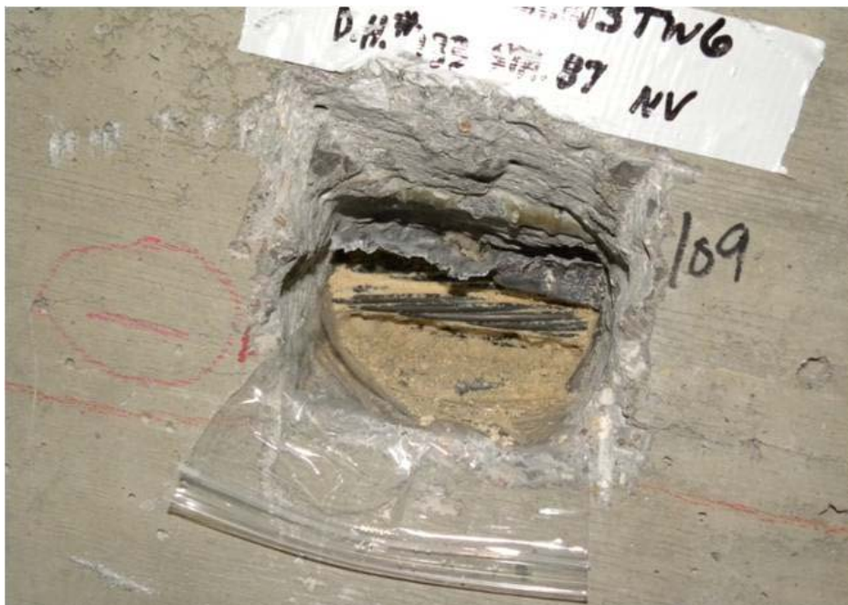
Figure 57. Photo. Access hole in an internal tendon at an intermediate location revealing strand and grout.
