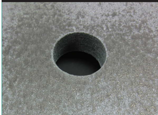
Figure 5. Typical post-test faying surface of sealed TSC.
