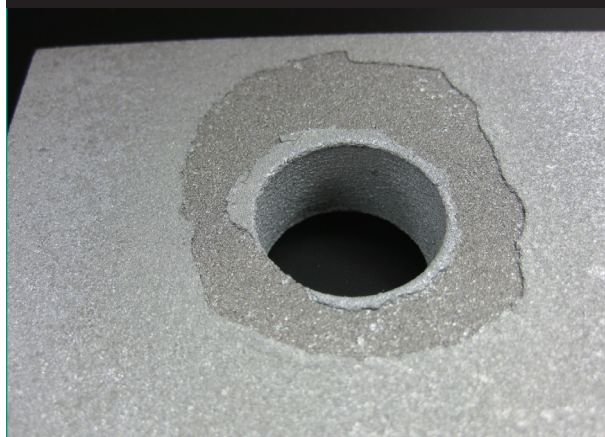
Figure 4. Typical post-test faying surface of unsealed TSC.
