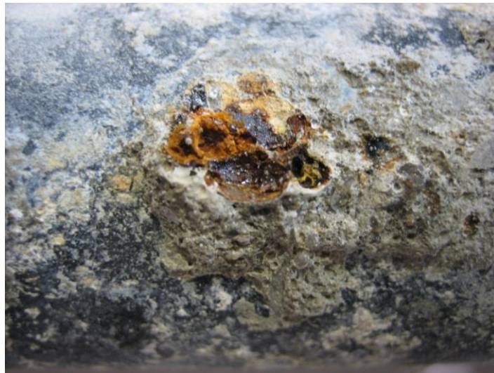
Figure 73. Photo. Close-up of another HDG bar (GL2).
