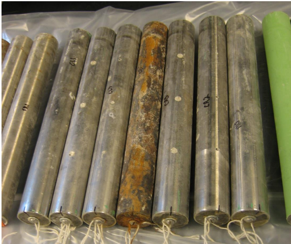
Figure 97. Photo. Condition of the as-extracted bars from the SCC bar slab.
