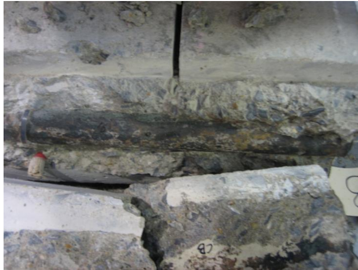
Figure 98. Photo. Condition of the exposed black bar (CB).
