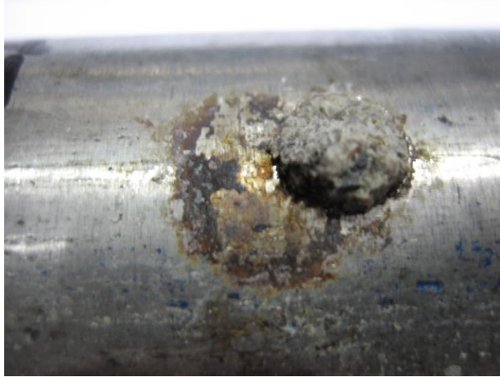
Figure 91. Photo. Close-up of a corroding artificial defect on the bar shown in figure 90.
