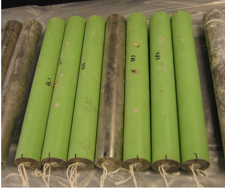
Figure 59. Photo. Condition of as-extracted bars from EC bar slab.
