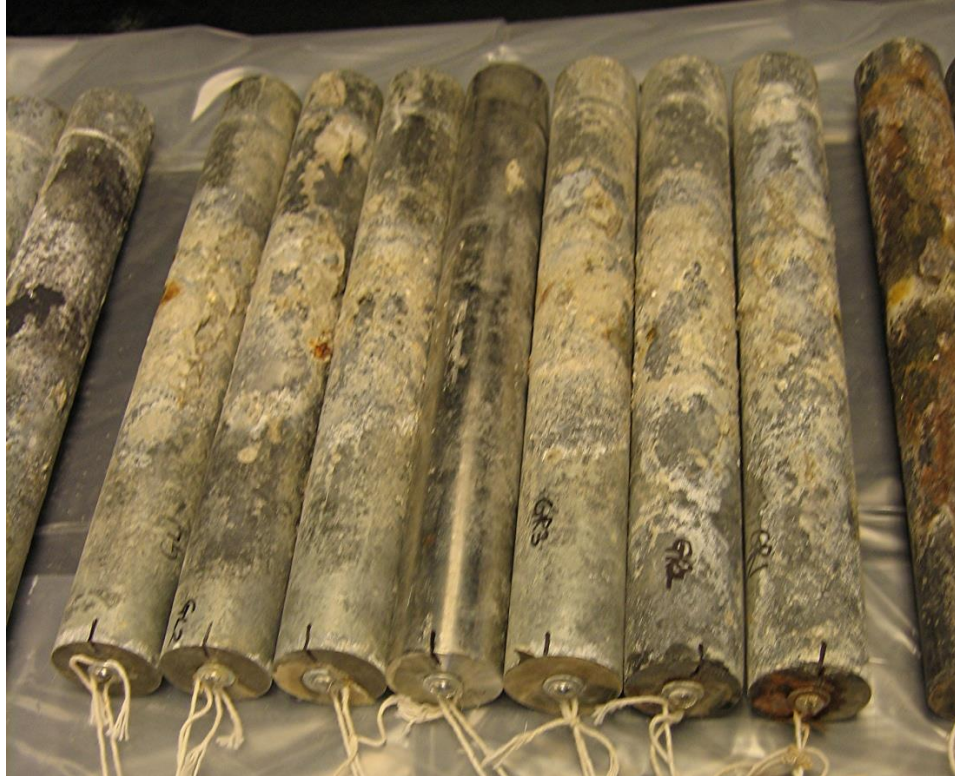
Figure 68. Photo. Condition of as-extracted bars from HDG bar slab.
