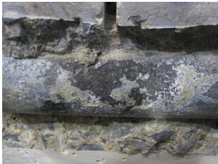
Figure 82. Photo. Condition of another exposed ZC bar (ZL1).
