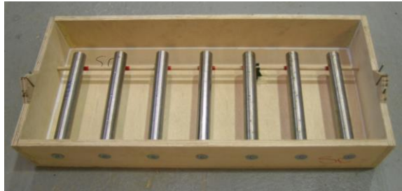
Figure 12. Photo. SCA and SCB bars and a type 316L solid SS bar in the center (SCA and SCB bar slab).
