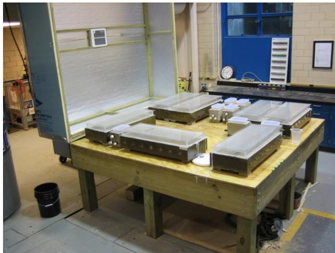
Figure 18. Photo. Exposure test setup in a heat tent.
