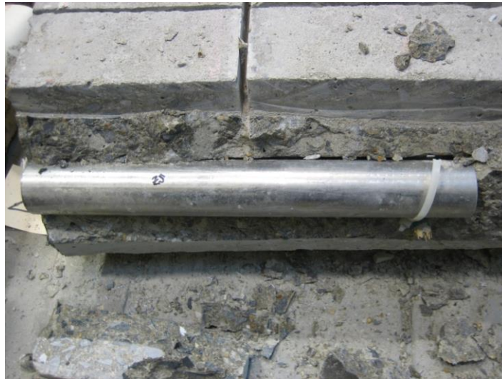
Figure 106. Photo. Clean condition of an exposed type 316L solid SS bar.
