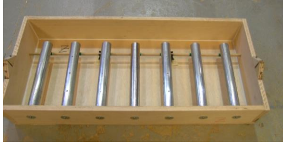
Figure 11. Photo. ZC bars and a type 316L solid SS bar in the center (ZC bar slab).
