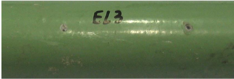
Figure 64. Photo. As-extracted condition of the bar shown in figure 63.
