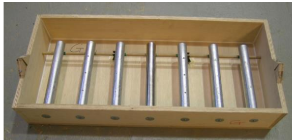
Figure 10. Photo. HDG bars and a type 316L solid SS bar in the center (HDG bar slab).
