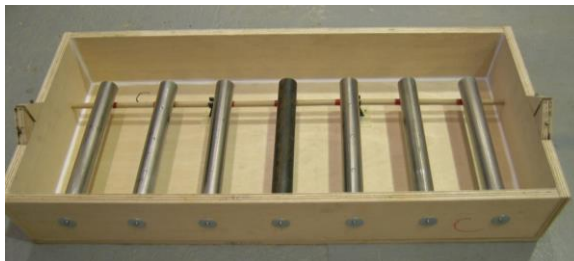
Figure 12. Photo. SCA and SCB bars and a type 316L solid SS bar in the center (SCA and SCB bar slab).
