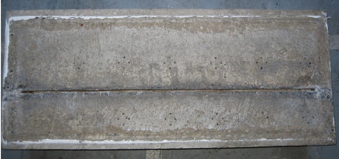
Figure 67. Photo. Top surface condition of HDG bar slab before autopsy.
