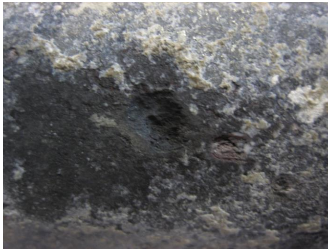
Figure 86. Photo. Close-up of a deep pit.
