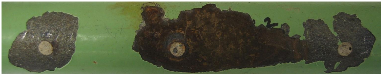
Figure 62. Photo. Autopsied condition of the bar shown in figure 61.
