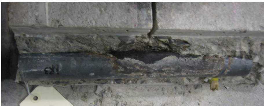
Figure 53. Photo. Condition of an exposed black bar (BL3).
