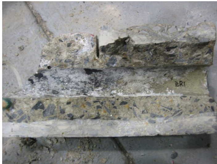
Figure 79. Photo. Bar/concrete interface for the bar shown in figure 78.
