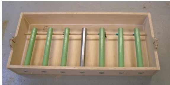
Figure 9. Photo. EC bars and a type 316L solid SS bar in the center (EC bar slab).
