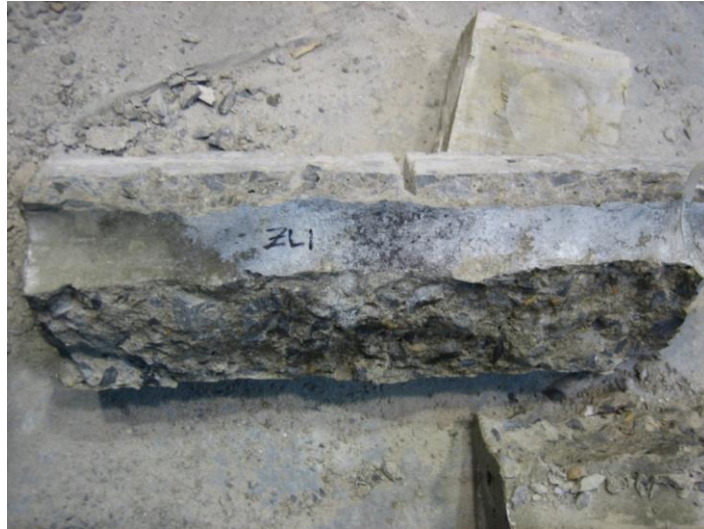
Figure 83. Photo. Bar/concrete interface for the bar shown in figure 82.
