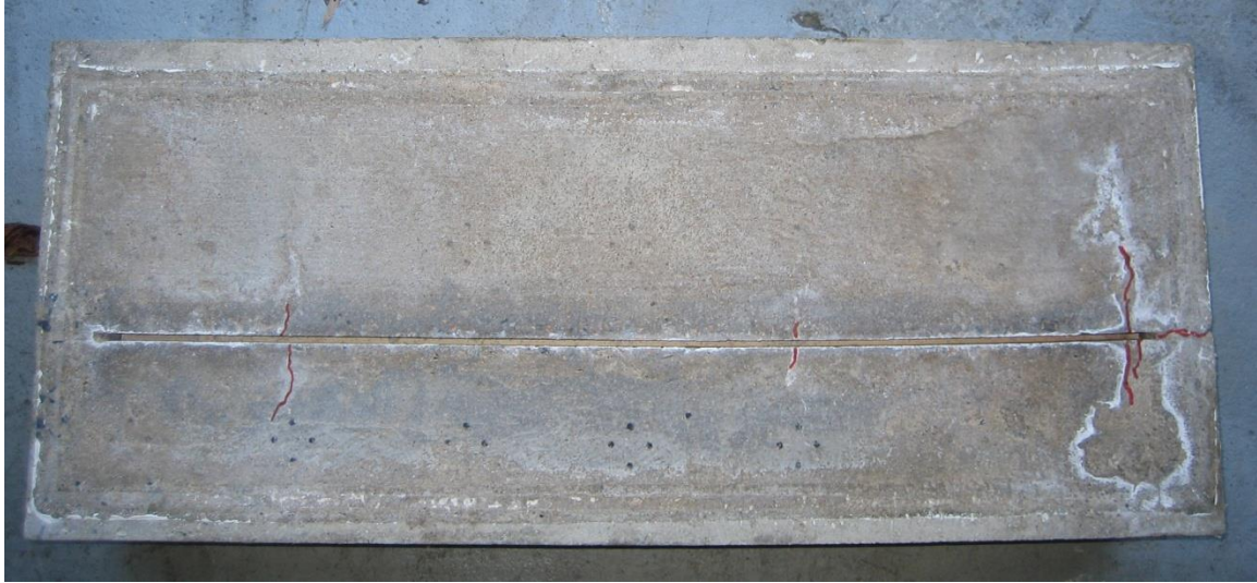
Figure 103. Photo. Top surface condition of the assorted bar slab before autopsy.
