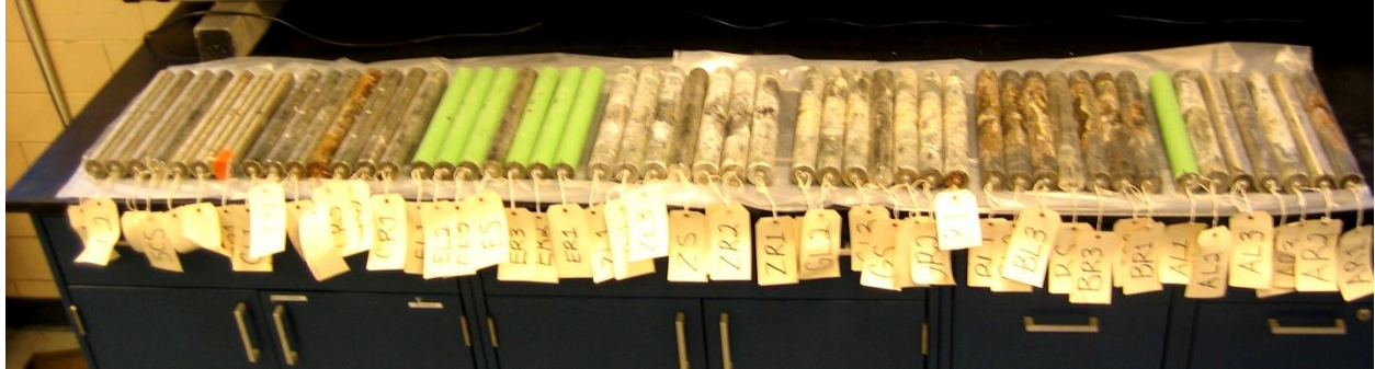
Figure 50. Photo. Overview of the entire extracted dowel bars.
