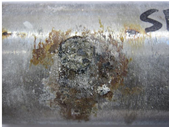
Figure 95. Photo. Close-up of a corroding artificial defect on the bar shown in figure 94.
