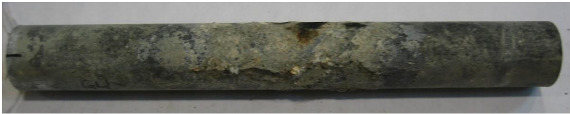
Figure 69. Photo. Condition of an exposed HDG bar (GL1).
