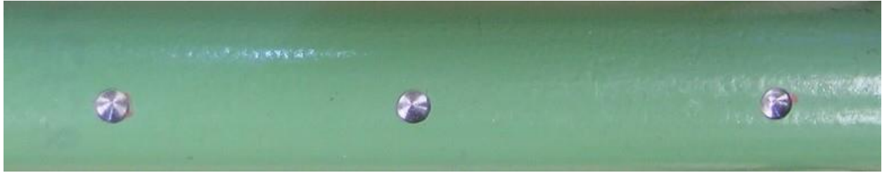
Figure 60. Photo. Initial condition of an EC bar (EL2).
