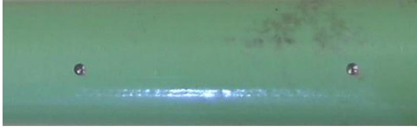
Figure 63. Photo. Initial condition of another EC bar (EL3).
