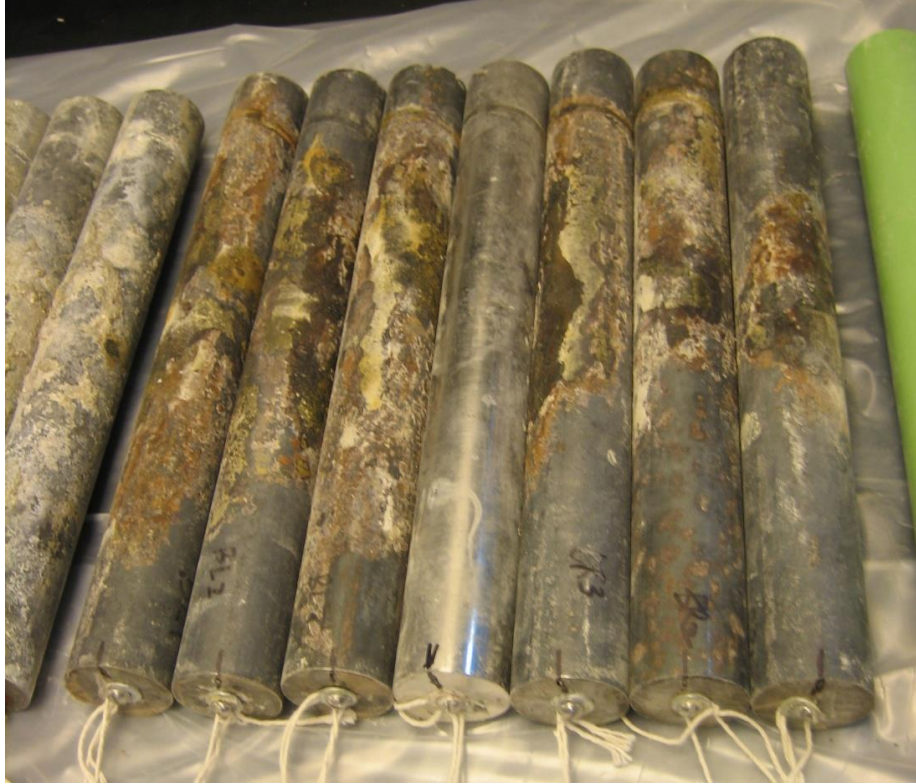
Figure 52. Photo. Condition of as-extracted bars from black bar slab.
