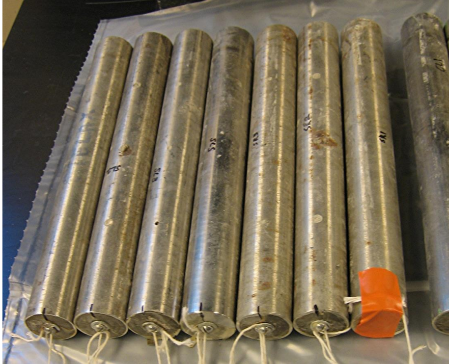
Figure 89. Photo. Condition of as-extracted bars from SCA/SCB bar slab.
