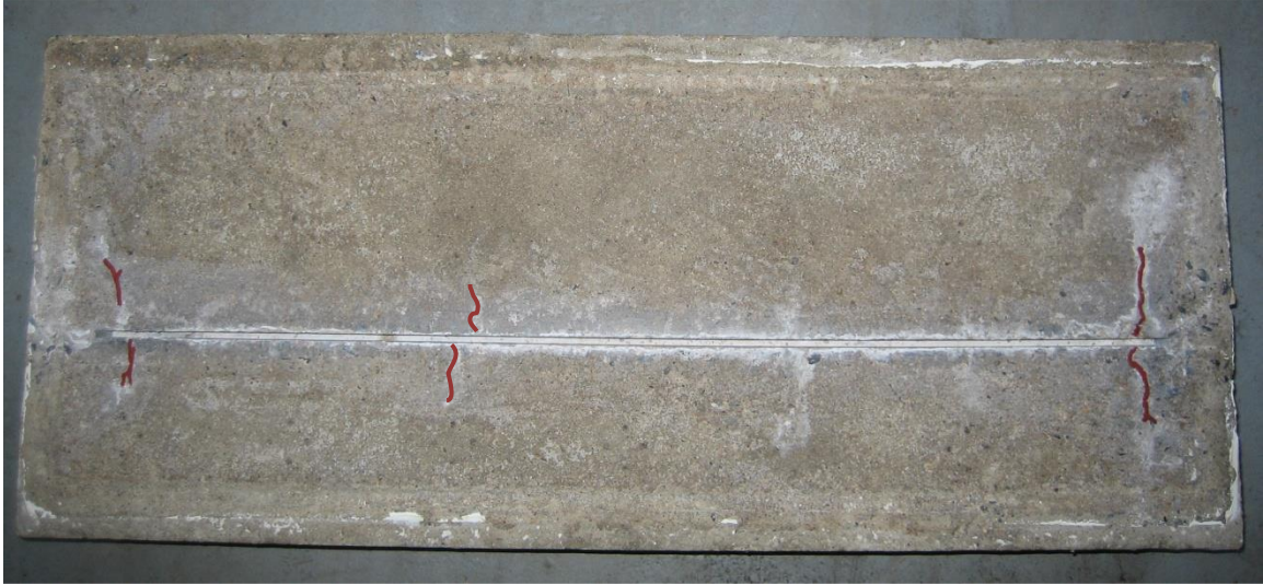
Figure 76. Photo. Top surface condition of ZC bar slab before autopsy.
