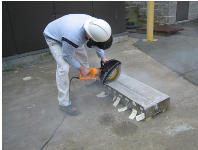
Figure 23. Photo. Saw cutting of a test slab.
