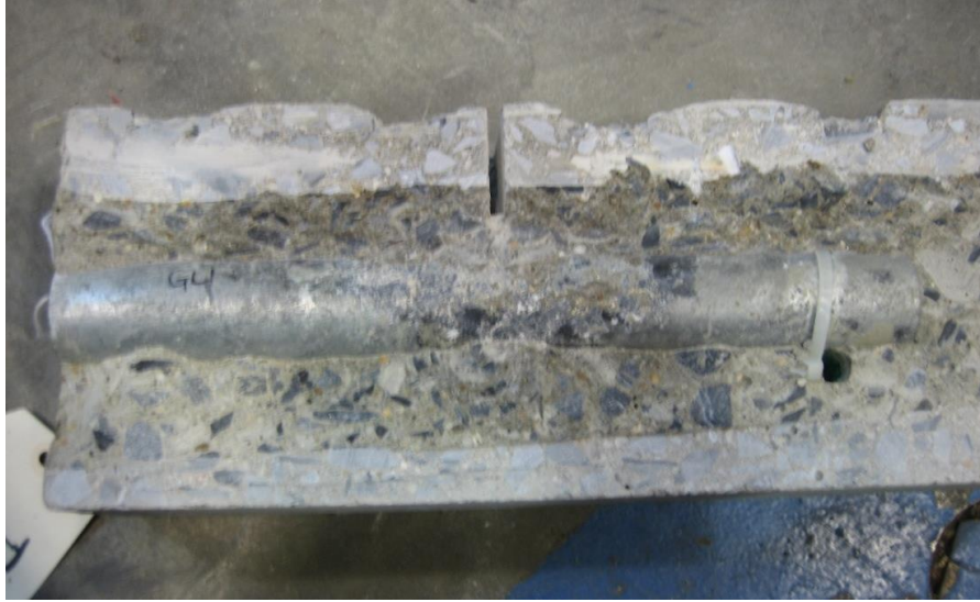
Figure 69. Photo. Condition of an exposed HDG bar (GL1).
