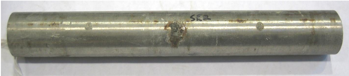
Figure 94. Photo. Top side of an extracted SCB bar (SR2).
