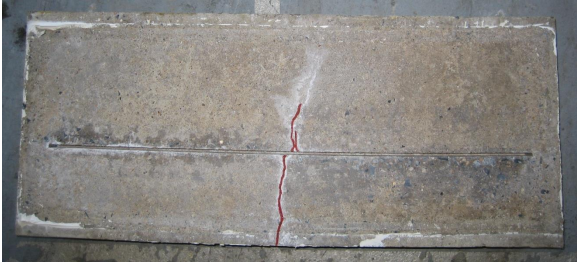
Figure 96. Photo. Top surface condition of the SCC bar slab before autopsy.
