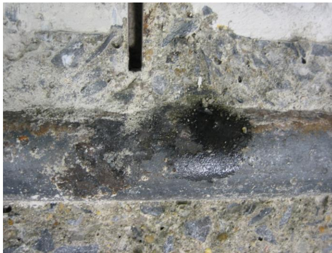
Figure 55. Photo. Bottom side of the bar shown in figure 53.
