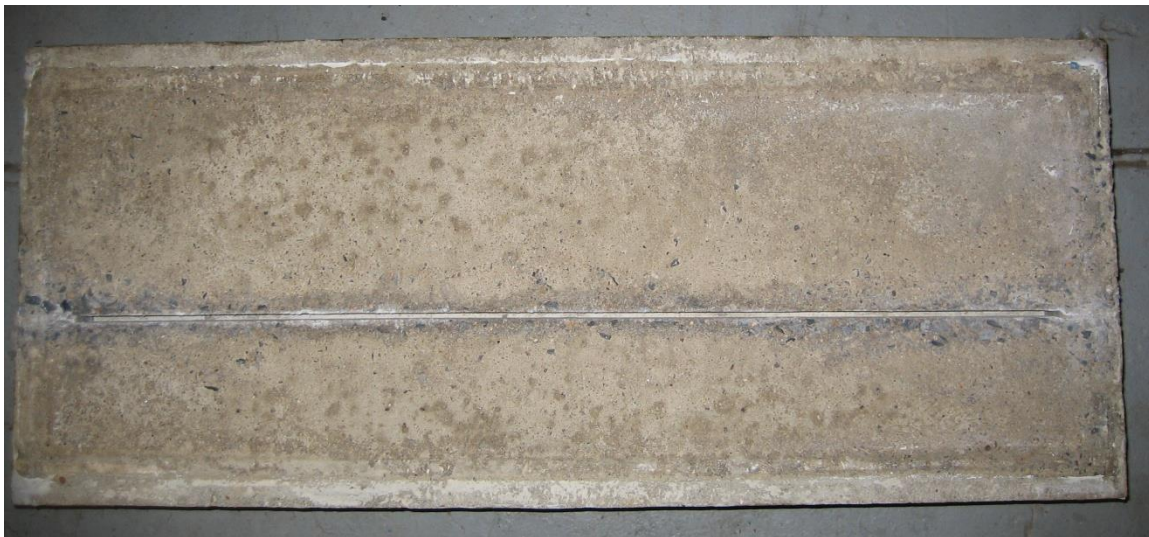
Figure 58. Photo. Top surface condition of EC bar slab before autopsy.
