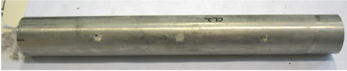
Figure 101. Photo. Top side of an extracted SCC bar (CL2).
