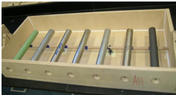
Figure 13. Photo. SCC bars and a black bar in the center (SCC bar slab).
