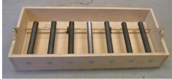
Figure 8. Photo. Black bars and a type 316L solid SS bar in the center (black bar slab).
