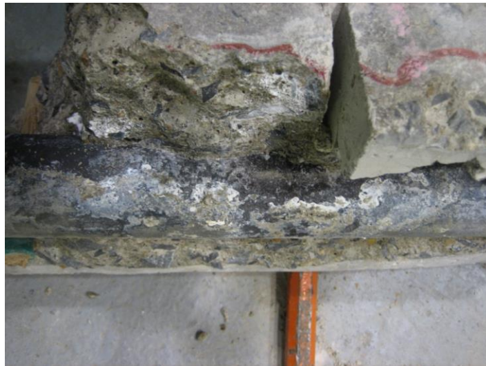
Figure 78. Photo. Condition of an exposed ZC bar (ZR1).
