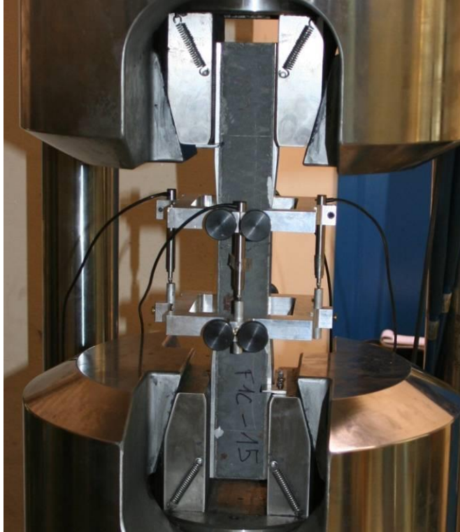
Figure 13. Photo. Testing of a longer 431.8-mm (17-inch)-long specimen.
