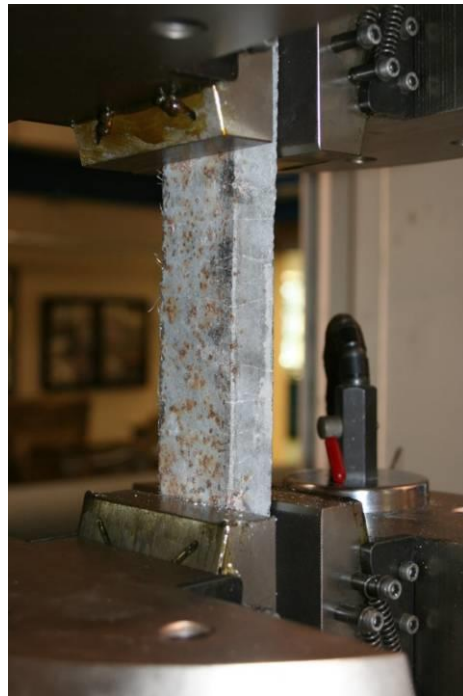
Figure 1. Photo. Extraction of a prismatic specimen from a beam tensile face.
