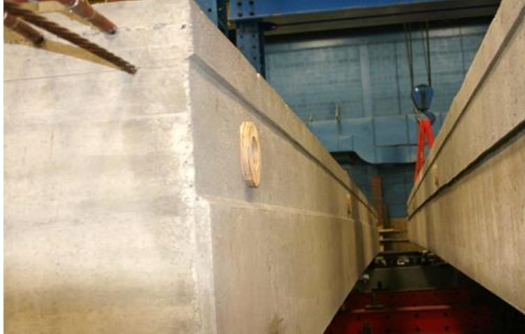
Figure 3. Photo. Alignment of the partial-depth conventional grout connection.
