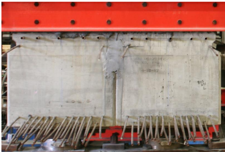
Figure 13. Photo. Partial-depth beams aligned for connection with the conventional grout shear key connection.
