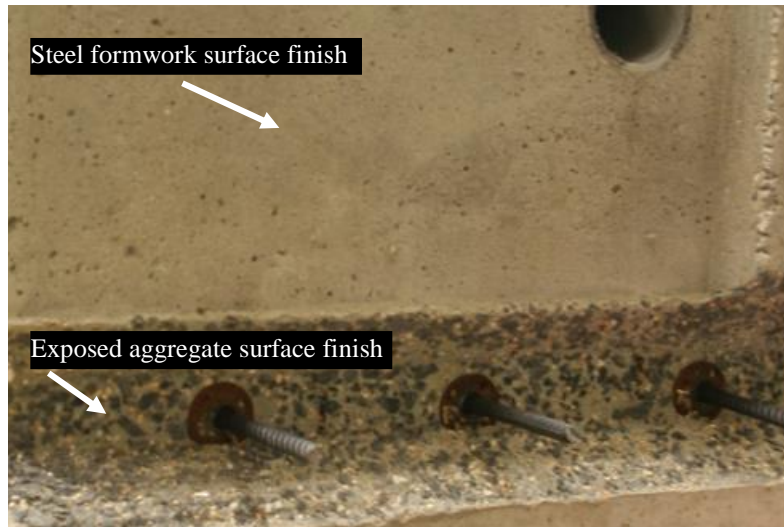
Figure 8. Photo. EA surface finish utilized in the UHPC connection.
