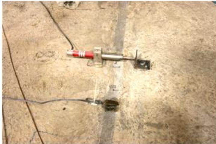
Figure 30. Photo. Five LVDTs (four vertical and one transverse) at the mid-span used to measure vertical deflection of the beams and the transverse connection opening.
