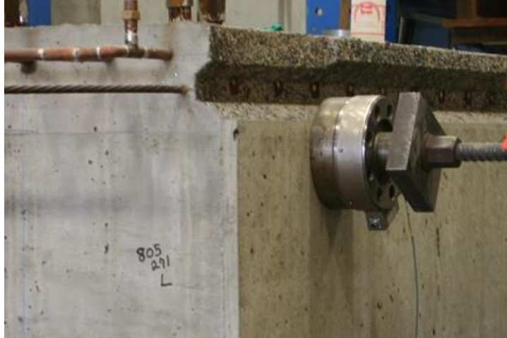
Figure 21. Photo. Transverse PT monitored with a load cell.
