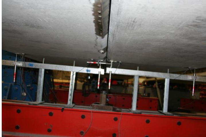
Figure 30. Photo. Five LVDTs (four vertical and one transverse) at the mid-span used to measure vertical deflection of the beams and the transverse connection opening.
