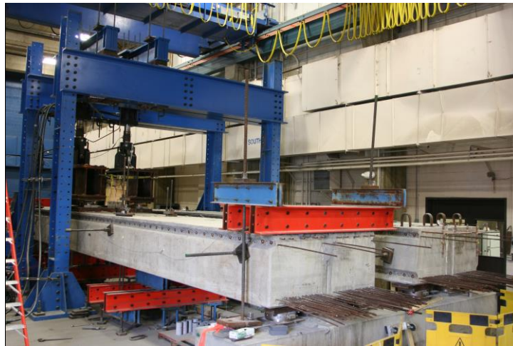
Figure 23. Photo. Cyclic structural loading test setup.
