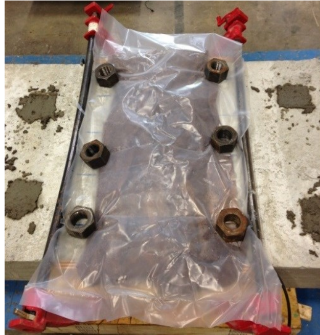
Figure 26. Photo. Curing of UHPC in deck-level connection specimen.
