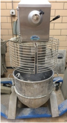
Figure 18. Photo. Planetary bowl and paddle mixer for UHPC batches up to 0.75 ft 3 (0.02 m 3 ).
