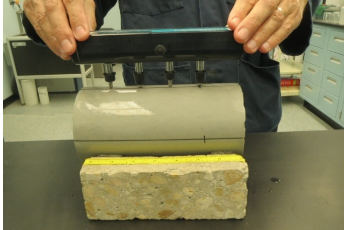
Figure 129. Photo. Setup for surface resistivity test.
