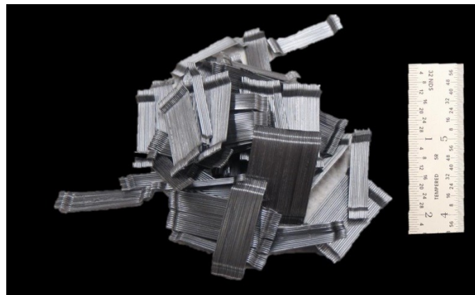
Figure 12. Photo. Photo of the steel fiber reinforcement used in U-A.
