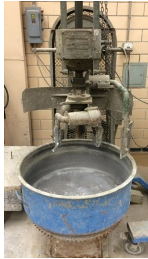
Figure 19. Photo. Small pan-style mixer for UHPC batches up to 1.0 ft 3 (0.028 m 3 ).
