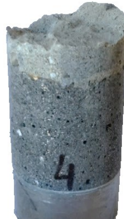
Figure 109. Photo. Substrate failure mode in direct tension pull-off tests.
