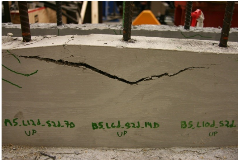
Figure 144. Photo. Bond test failure due to cone-shaped block fracture mode.
