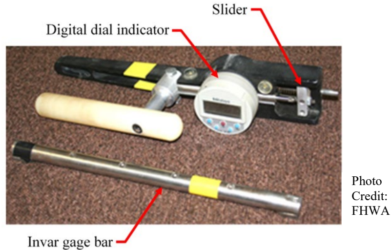
Figure 8. Photo. DEMEC Instrument and Gauge Bar.
