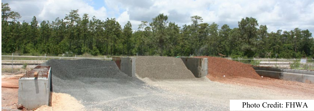
Figure 5. Photo. Lightweight Aggregate Stockpiles at Precaster’s Facility with Continuous Sprinklers.
