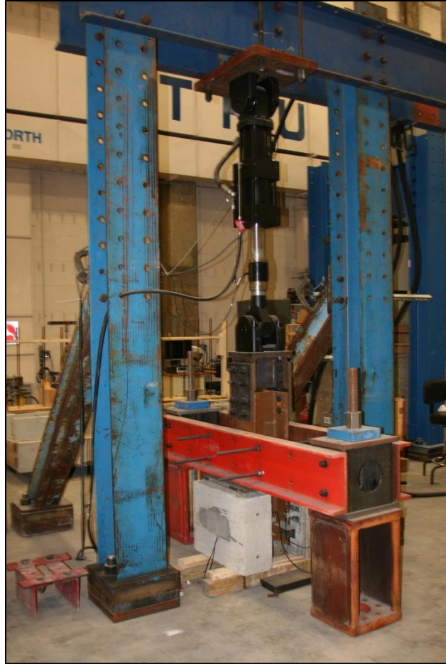
Figure 35. Photo. Small-scale fatigue test setup.
