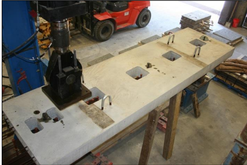
Figure 13. Photo. Before grouting large-scale beam specimen 4F1.
