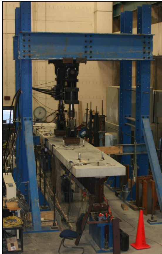
Figure 18. Photo. Southwest view of large-scale fatigue test setup.
