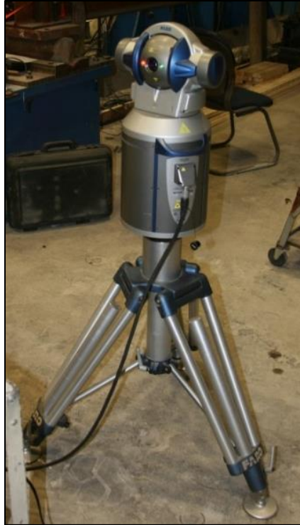
Figure 30. Photo. Laser tracker system head unit.
