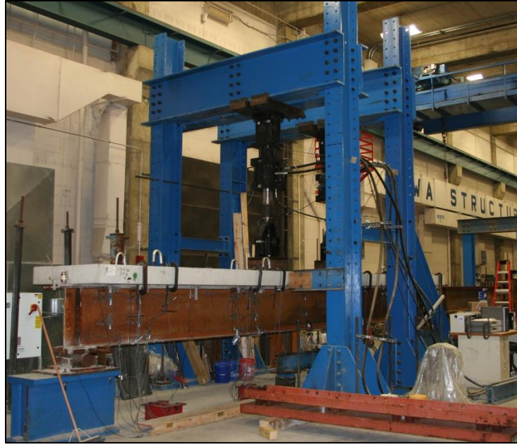
Figure 18. Photo. Southwest view of large-scale fatigue test setup.
