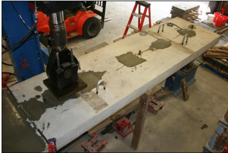
Figure 14. Photo. After grouting large-scale beam specimen 4F1.
