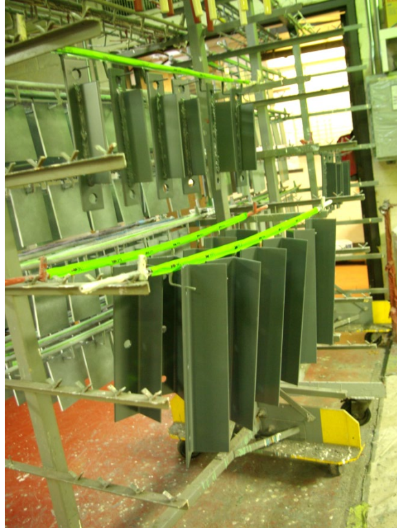
Figure 4. Photo. Coating application for large panel attachments.
