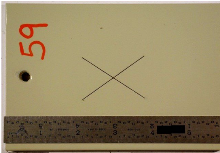
A. Standard size panel with a single-line scribe.
