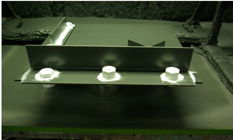
Figure 4. Photo. Coating application for large panel attachments.
