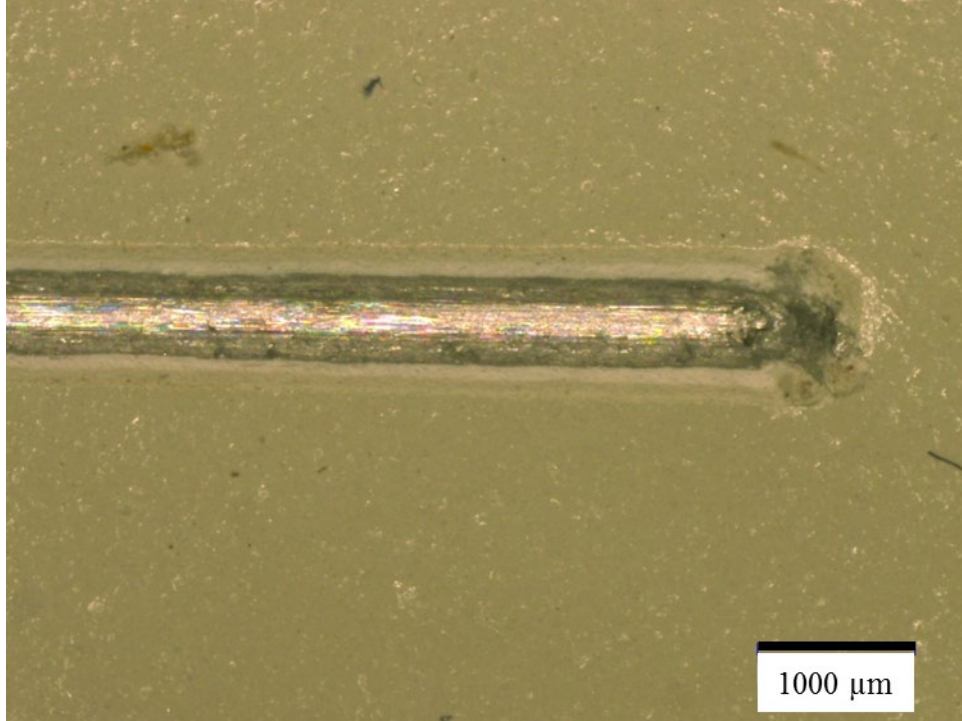
A. Microscopic image of a single-line scribe.
