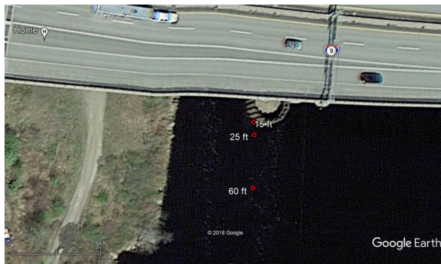
© 2018 Google®. FHWA modifications include red dots and text overlays to identify standoff distance from the bridge structure.
