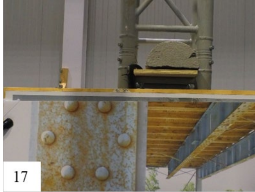
Figure 95. Photo. Image 17, fracture critical member and cracked concrete sample taken at 5 ft.
