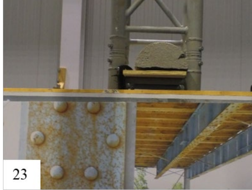
Figure 101. Photo. Image 23, fracture critical member and cracked concrete sample taken at 5 ft.
