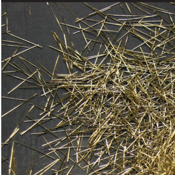
Figure 1. Photo. Commonly used steel fiber reinforcement. (25)
