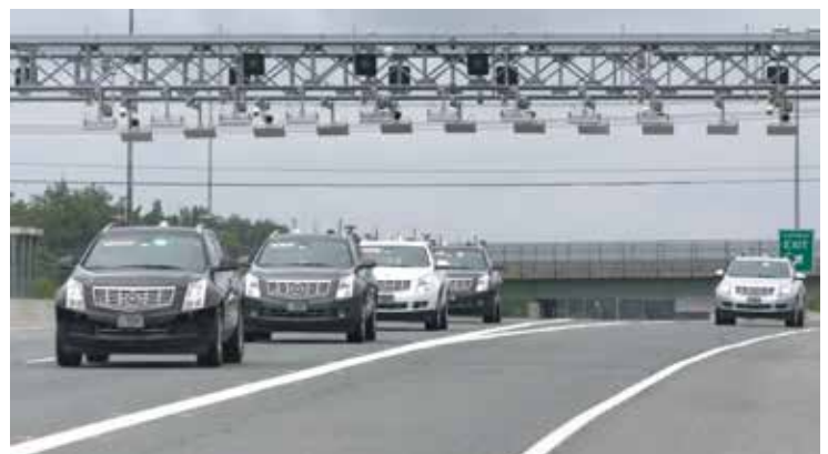
Figure 3. Photo. A car approaches to merge with a 4-car platoon. (Source: FHWA).
