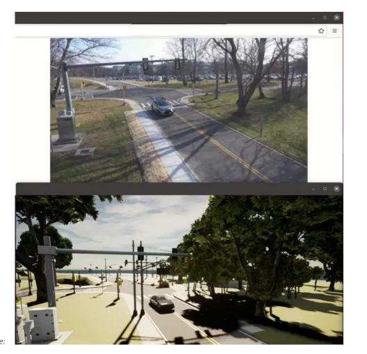
All photos source FHWA. VOICES is demonstrated in this image, which depicts a live vehicle driving along a roadway while its virtual counterpart is displayed in a CARLA simulation running in a computer. This image highlights the possibility of experimenting with live and virtual interactions using a common set of adapters and interfaces.
