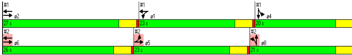
Figure 69. Screen Capture. Timing Plan for Three-Phase Diamond Interchange in High Volumes.
