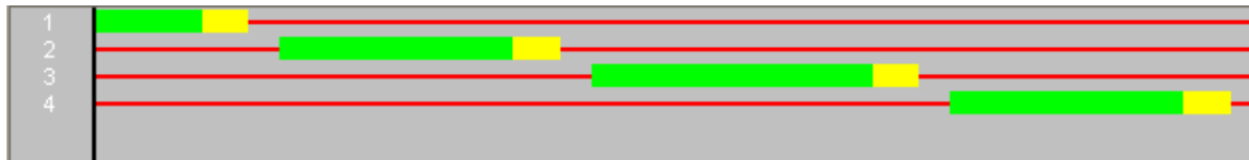
Figure 59. Illustration. Timing Plan for Intersection with Lead Left Turn in High Volumes (Cycle: 75; Split: 11, 20, 23, and 21).
