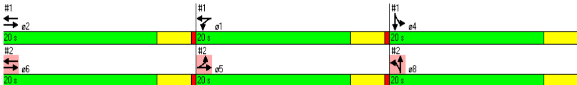
Figure 65. Screen Capture. Timing Plan for Three-Phase Diamond Interchange in Low Volumes.
