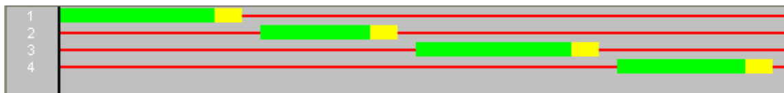
Figure 54. Illustration. Timing Plan for Intersection with Lag Left Turn in Low Volumes (Cycle: 80; Split: 22, 17, 22, and 19).
