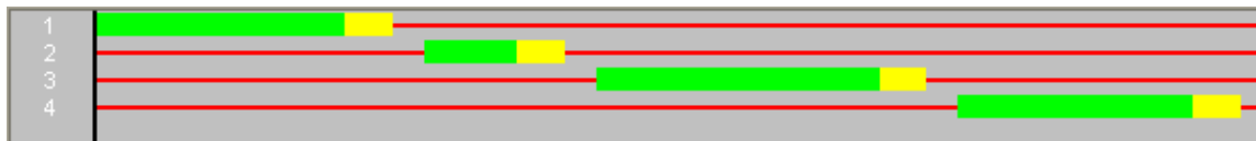
Figure 58. Illustration. Timing Plan for Intersection with Lag Left Turn in High Volumes (Cycle: 75; Split: 20, 11, 23, and 21).
