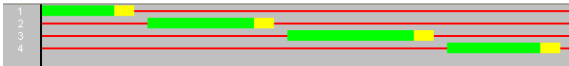
Figure 55. Illustration. Timing Plan for Intersection with Lead Left Turn in Low Volumes (Cycle: 80; Split: 17, 22, 22, and 19).
