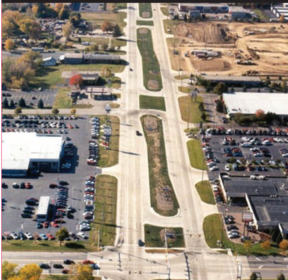
Figure 1. MUT intersection treatment in a corridor in Michigan.
