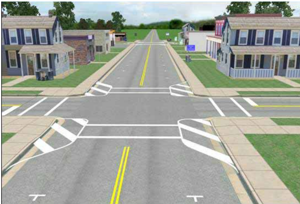
Figure 10. Screenshot. Painted bulb-outs condition.
