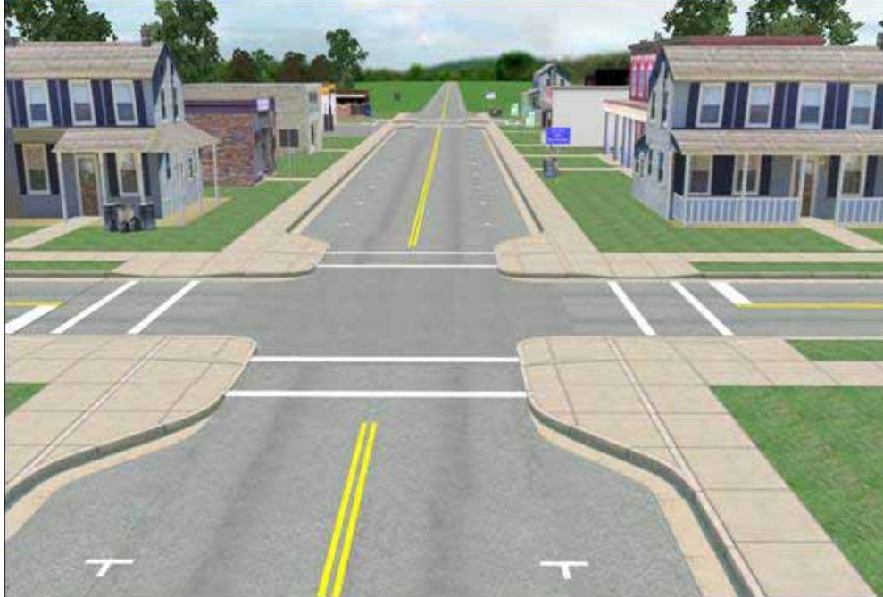
Figure 9. Screenshot. Curb and gutter bulb-outs condition.
