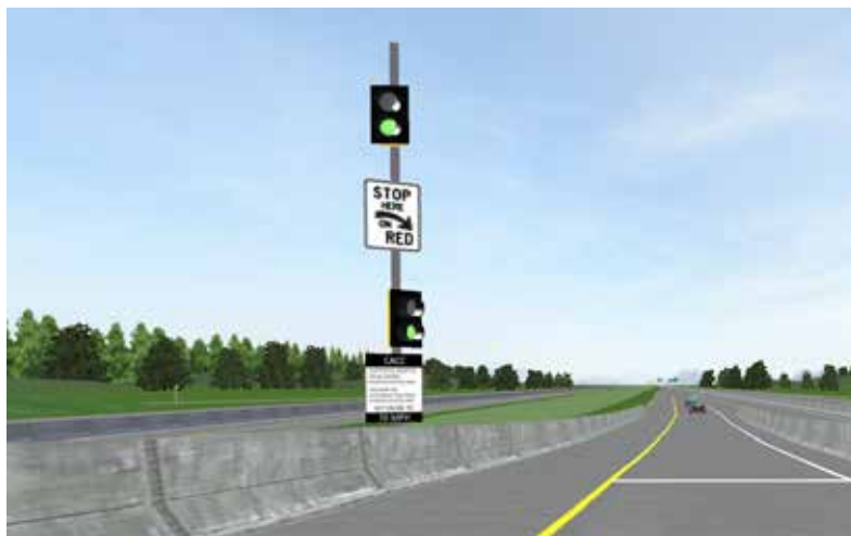
Figure 3. Screen capture. Entrance ramp meter.
