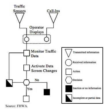
Figure 7. Flowchart. Example OSD for detecting incidents.<sup>(48)</sup>
