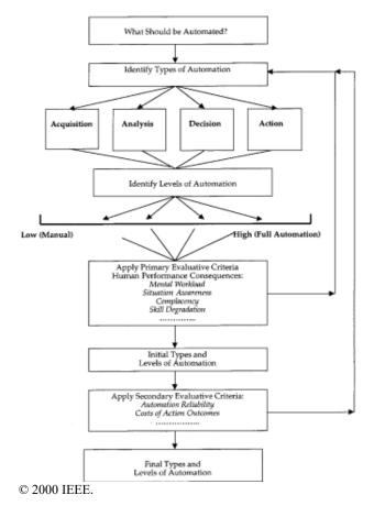
Figure 3. Flowchart. Steps to determine automated task allocation.<sup>(20)</sup>
