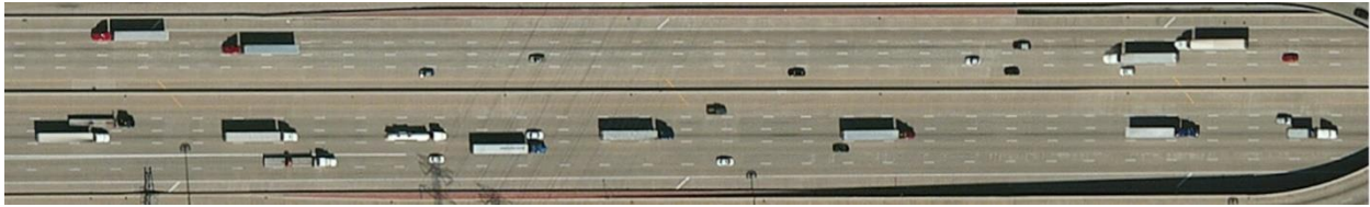
Figure 6. Photo. Multilane entrance ramp with tapered design, I-80 at I-94 eastbound, Lansing, IL. (31)
