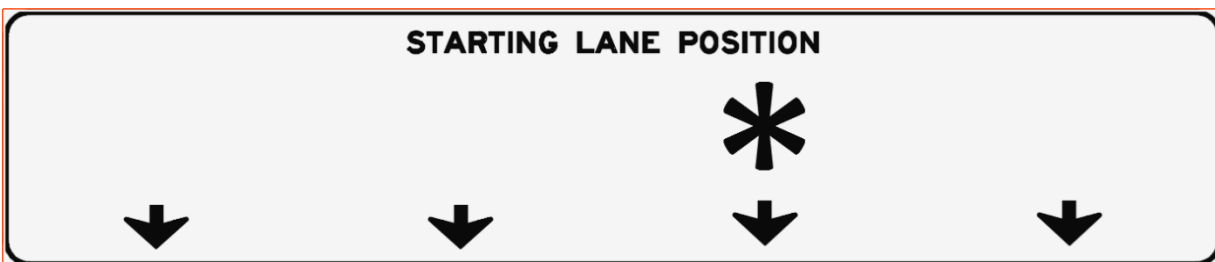
Figure 27. Graphic. Overhead sign that directed participants to a starting lane using the asterisk symbol location in one of four lanes.
