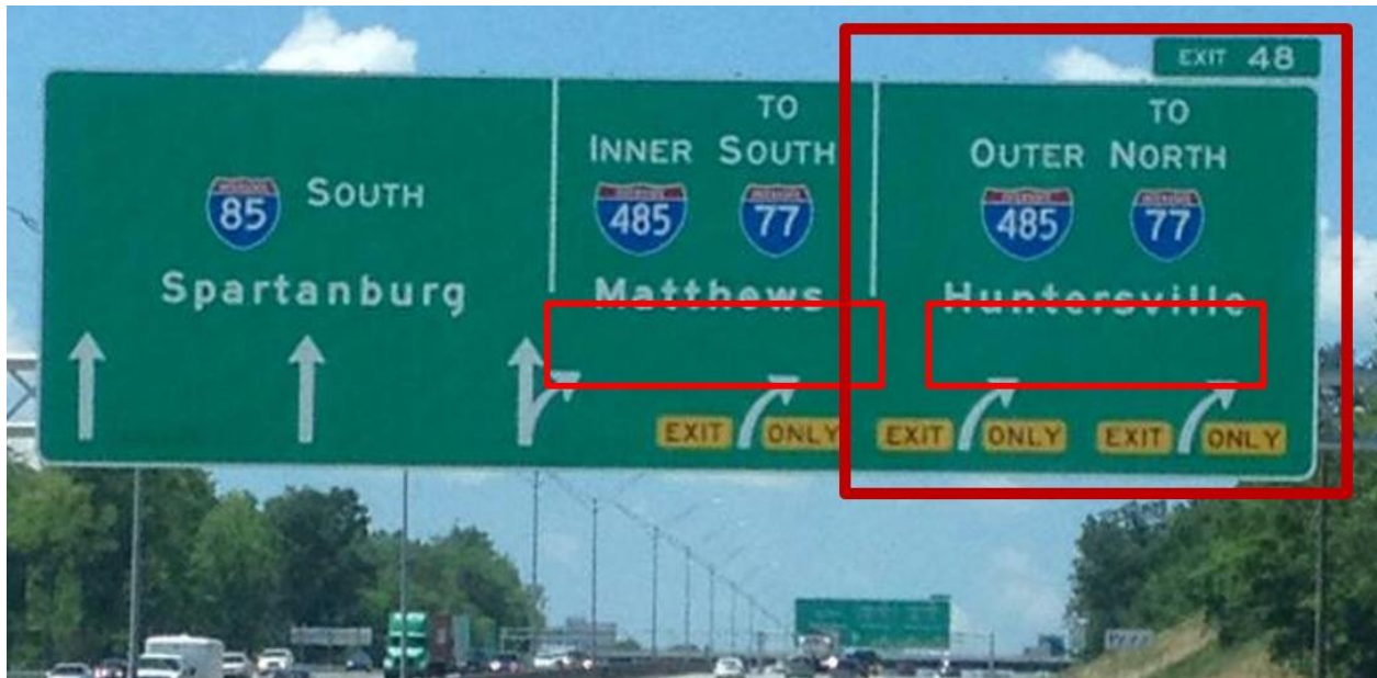
Figure 16. Photo. New installation of blended arrow guide sign in North Carolina.
