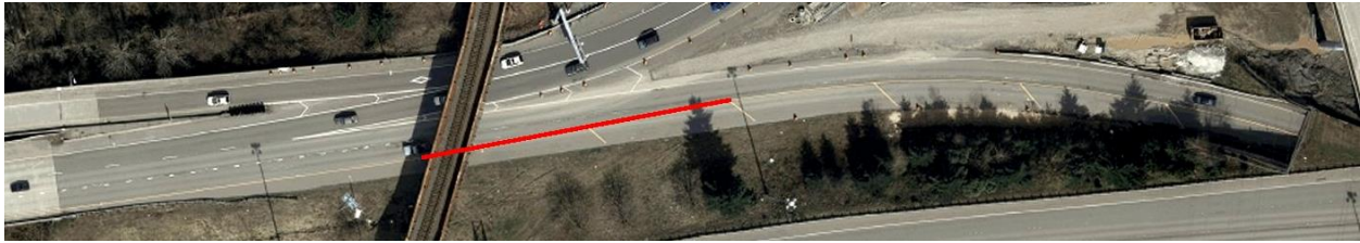
Figure 22. Photo. Location of left edgeline in an asymmetrical widening over and beyond a crest vertical curve. (37)
