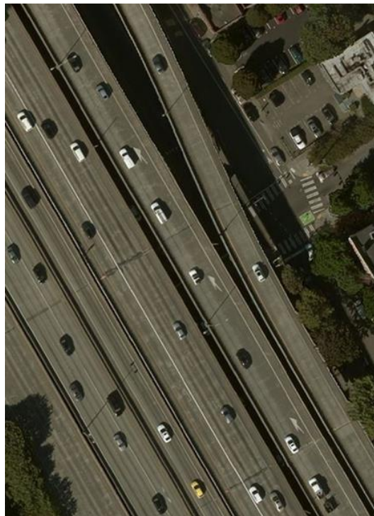
Figure 2. Photo. Satellite imagery of northbound Interstate 5 (I-5) C/D roadway north of I-90 with multiple successive lane-reduction arrows. (28)
