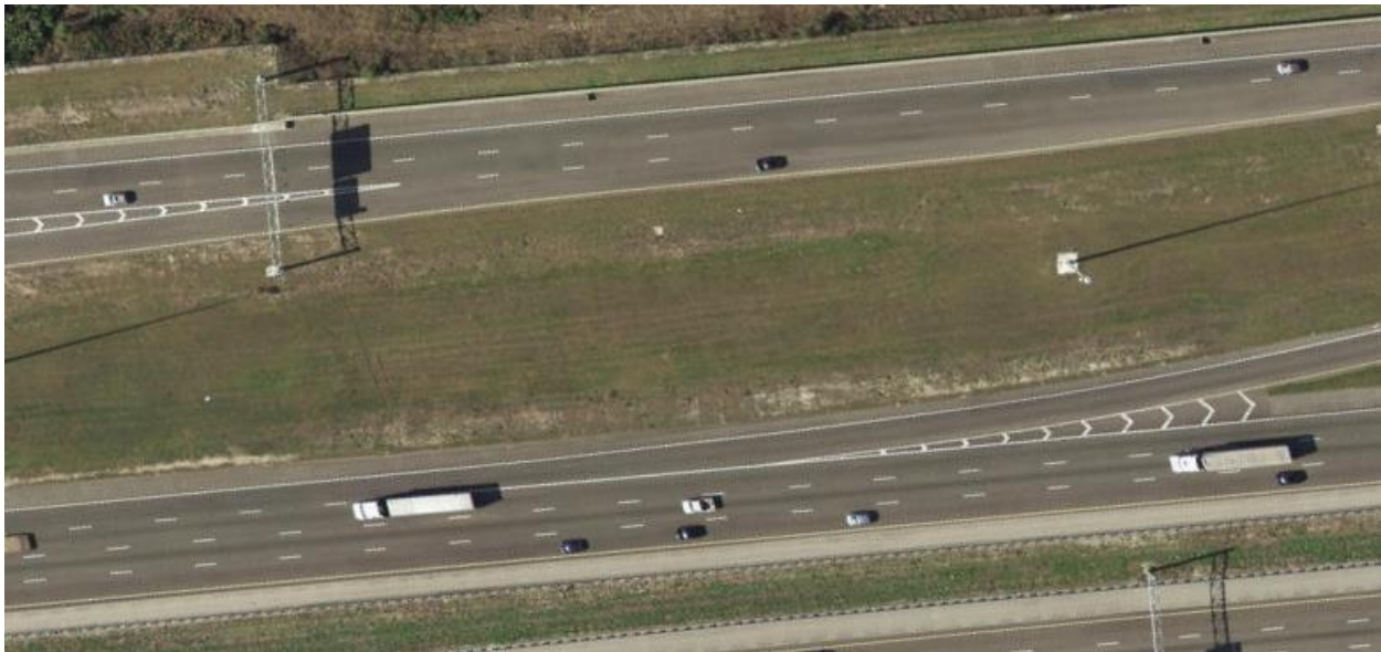
Figure 7. Photo. I-4 distributor roadway upstream of US 192 interchange in Kissimmee, FL, showing left exit from the distributor roadway. (32)
