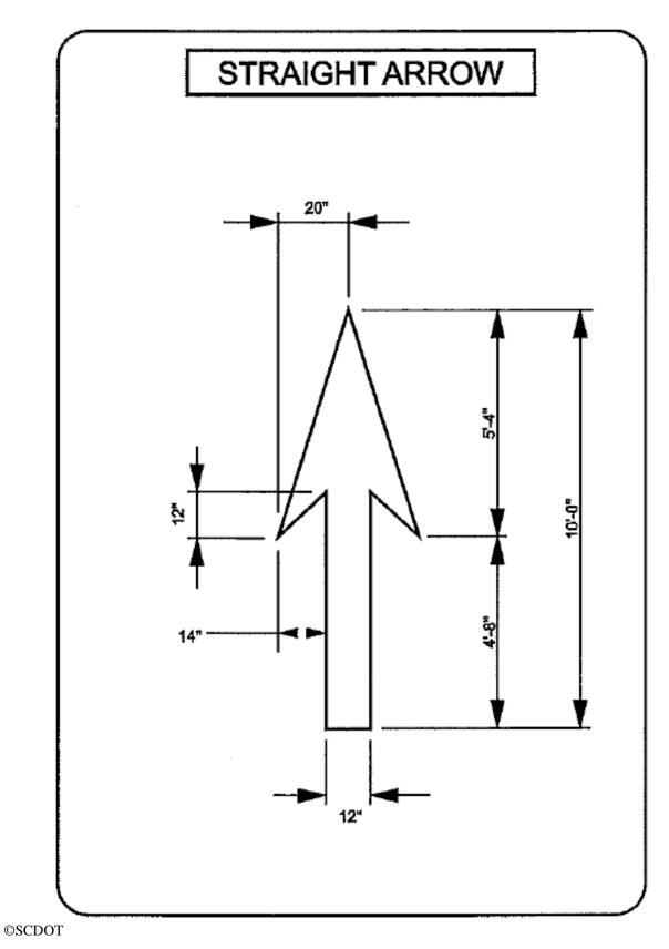
Figure 39. Illustration. SCDOT Standard Drawing 625-410-00 excerpt for straight arrow standard pavement marking.
