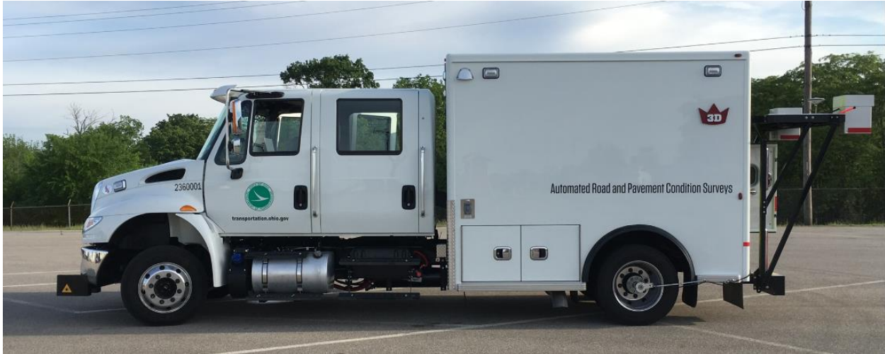
Figure 8. Photo. Ohio DOT van precisely tracks its position relative to the roadway as it gathers data on pavement conditions.
