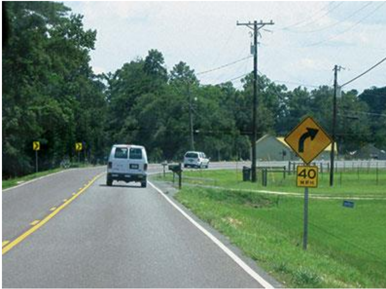
Figure 5. Photo. Arrow signs and chevrons can be used separately or in combination. (25)
