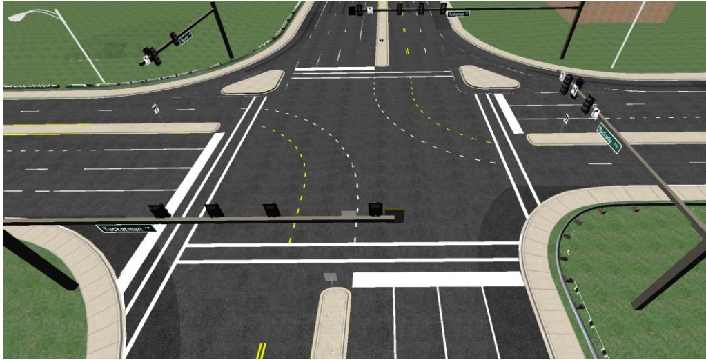
Figure 34. Illustration. Configuration of CLT intersection showing lane markings aligned with geometry.
