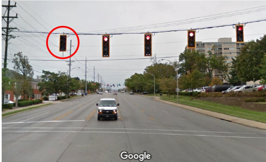
Figure 29. Map. Street view of a blank-out signal used to control a reversible lane on Nicholasville Road, Lexington, KY.
