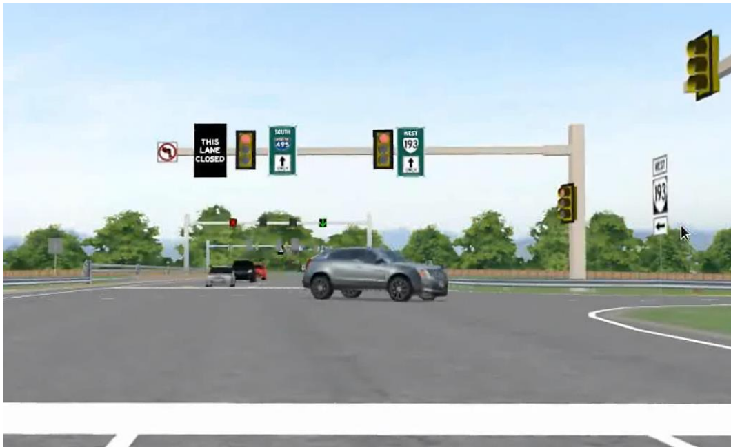
B. Scenario 3—participant’s point of view from the first intersection stop bar: off-peak-period traffic, arrival on red, “This Lane Closed” sign indicating the DRLT lane should not be used.
