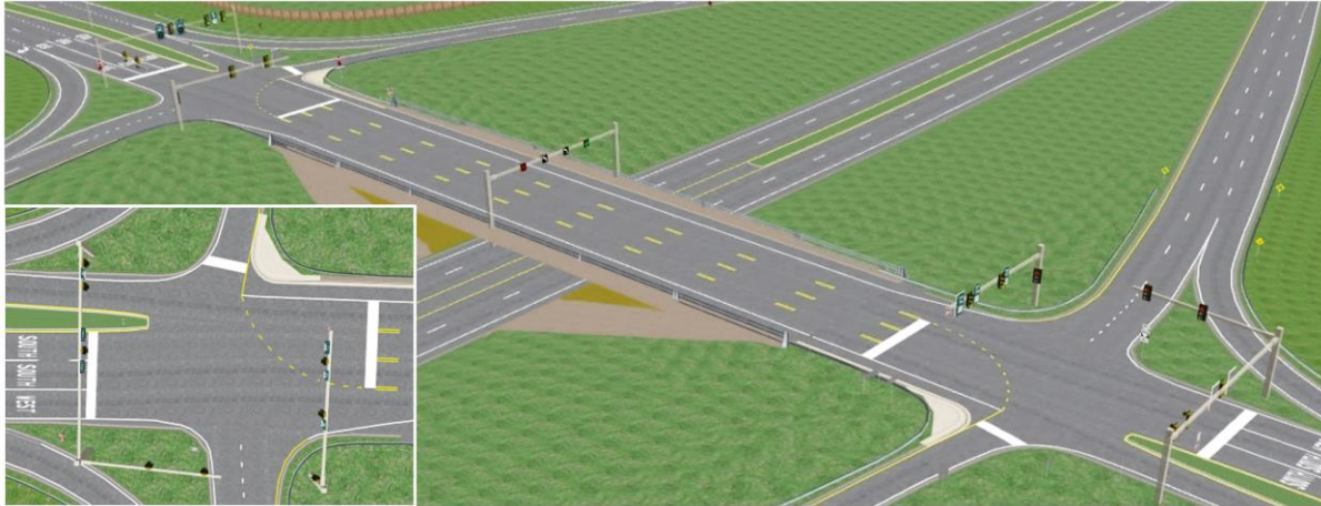
Figure 7. Illustration. DRLT-interchange scenario used in this study with an overhead view of the signalized intersection.
