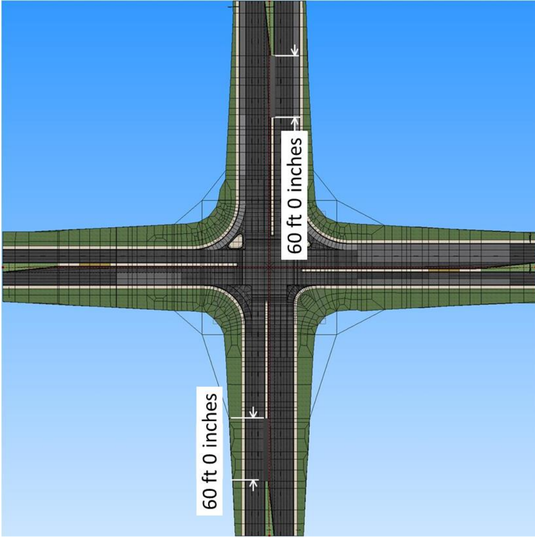
Figure 33. Illustration. Geometric design of a CLT intersection.
