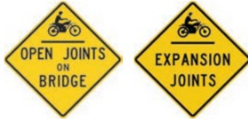
Figure 11. Illustration. Examples of joint signs used in Virginia. (46)
