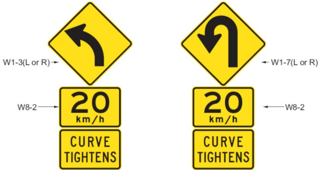
Figure 4. Illustration. Advance curve-warning sign with supplementary Curve Tightens plaque. (29)
