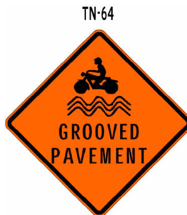
Figure 12. Illustration. Grooved-pavement-warning sign used in work zones in Tennessee. (48)
