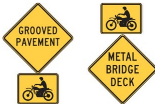
Figure 8. Illustration. Supplemental warning plaques for motorcyclists. (3)
