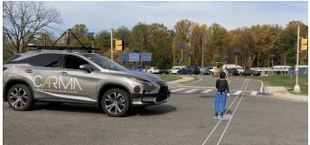
Figure 3. The Human Factors Team testing detection of an articulated child pedestrian dummy.
