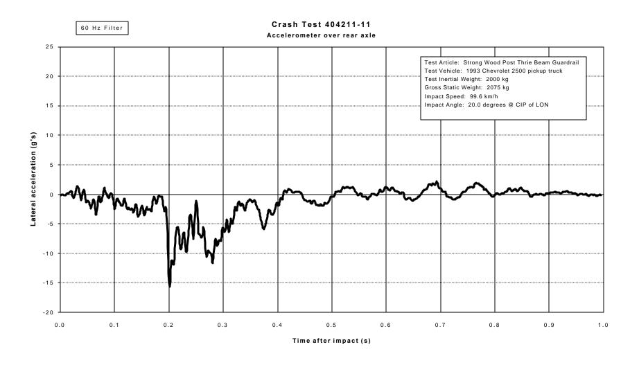
Figure 19. Vehicle lateral accelerometer traces for test 404211-11 (accelerometer located over rear axle).
