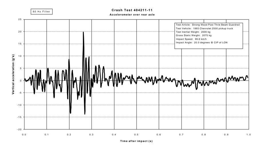
Figure 20. Vehicle vertical accelerometer traces for test 404211-11 (accelerometer located over rear axle).
