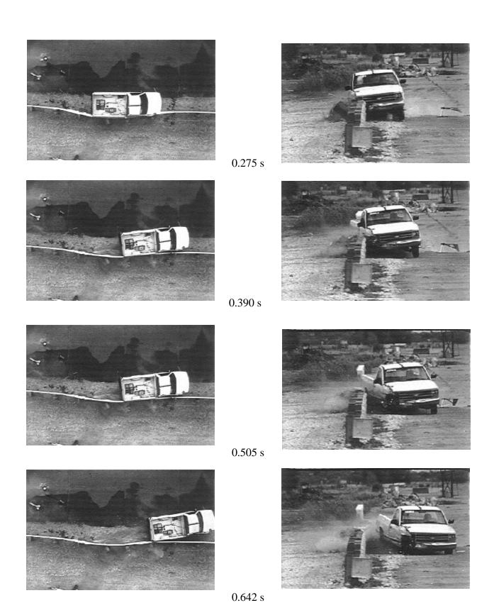
Figure 6. Sequential photographs for test 404211-11 (overhead and frontal views) (continued).
