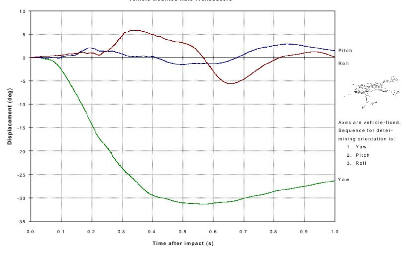
Figure 14. Vehicle angular displacements for test 404211-11.
