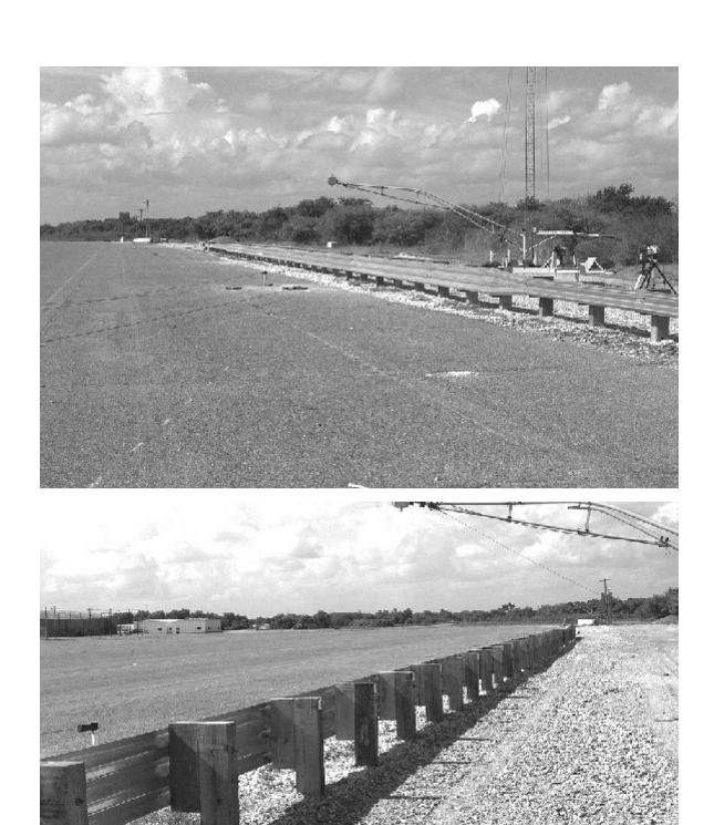
Figure 2. Strong Wood Post Thrie Beam Guardrail installation before test 404211-11.
