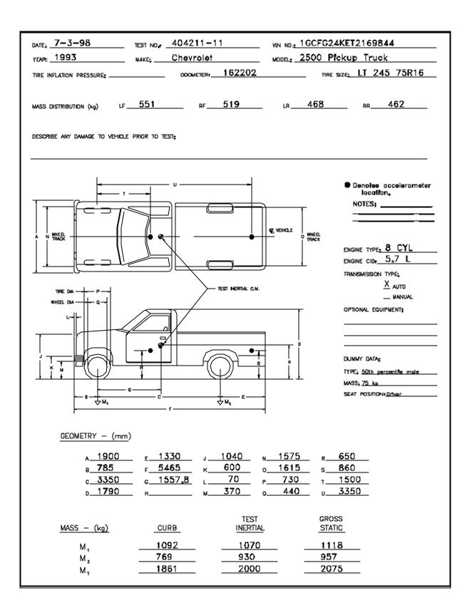
Figure 5. Vehicle properties for test 404211-11.
