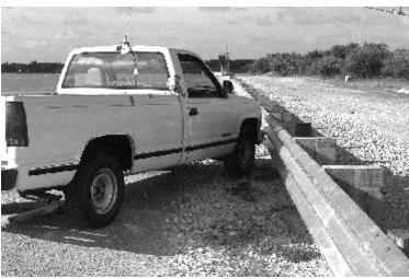
Figure 3. Vehicle/installation geometrics for test 404211-11.
