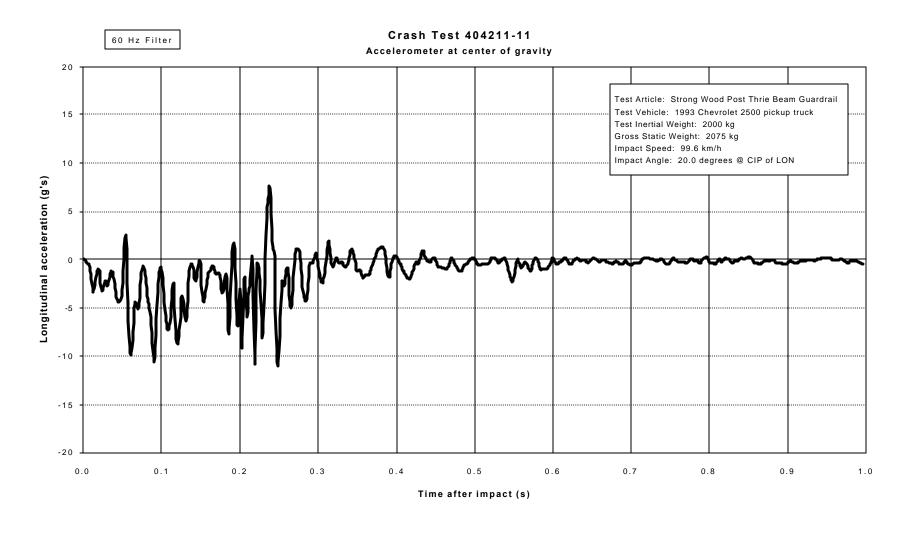
Figure 15. Vehicle longitudinal accelerometer trace for test 404211-11 (accelerometer located at center of gravity).
