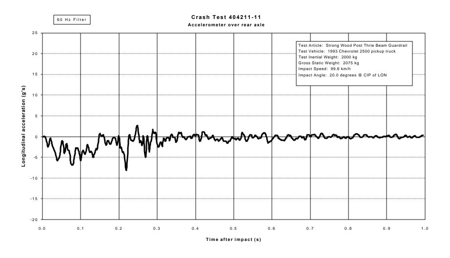
Figure 18. Vehicle longitudinal accelerometer trace for test 404211-11 (accelerometer located over rear axle).
