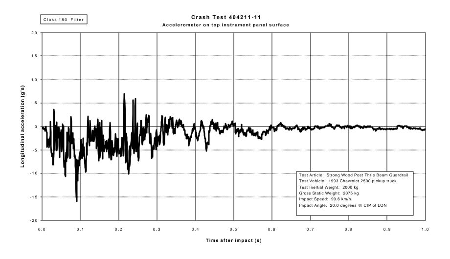
Figure 21. Vehicle longitudinal accelerometer trace for test 404211-11 (accelerometer located on top surface of instrument panel).
