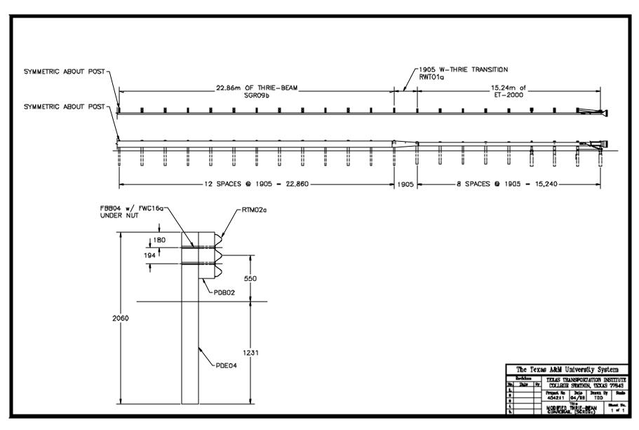
Figure 1. Details of the Strong Wood Post Thrie Beam guardrail installation.
