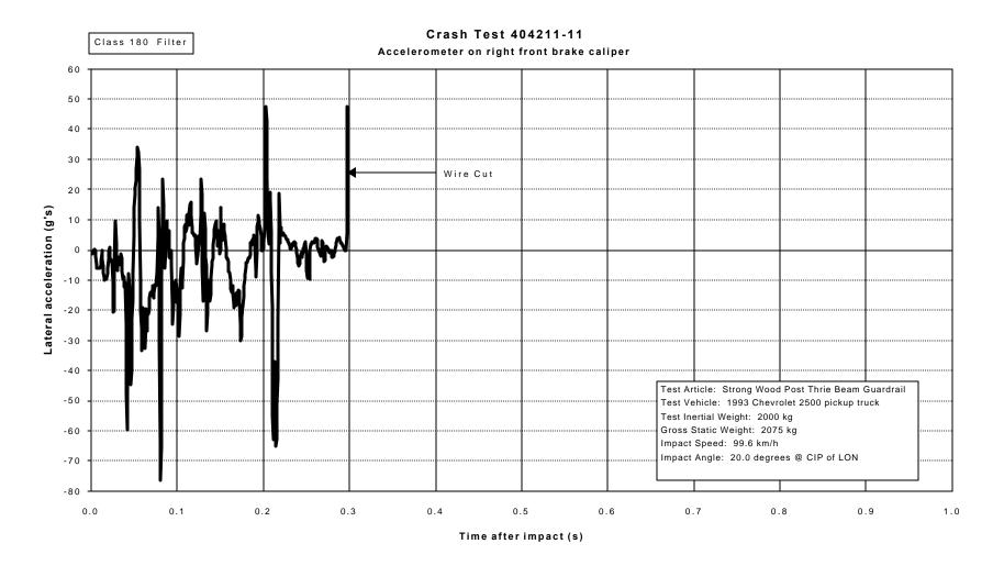
Figure 22. Vehicle lateral accelerometer trace for test 404211-11 (accelerometer located on right front brake caliper).
