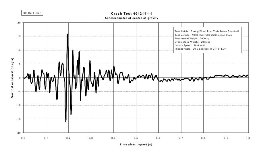
Figure 17. Vehicle vertical accelerometer trace for test 404211-11 (accelerometer located at center of gravity).
