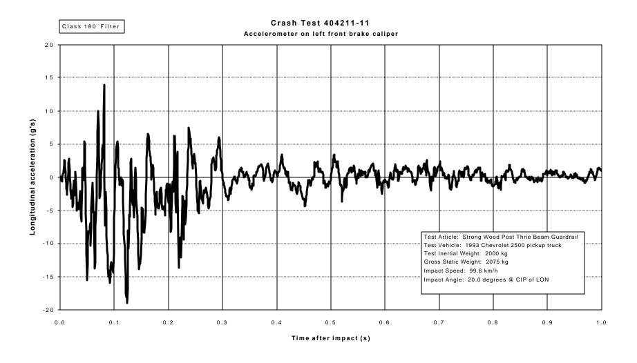
Figure 23. Vehicle longitudinal accelerometer traces for test 404211-11 (accelerometer located on left front brake caliper).
