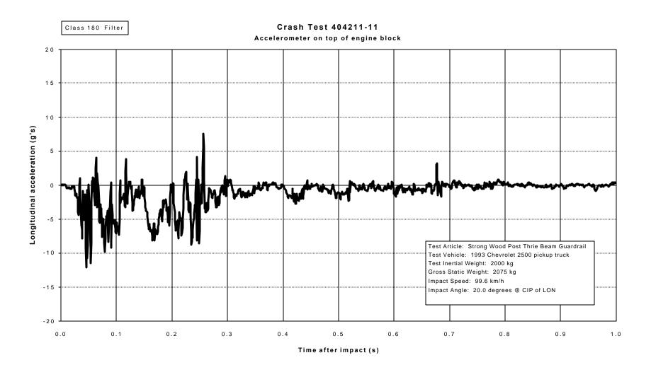
Figure 24. Vehicle longitudinal accelerometer trace for test 404211-11 (accelerometer located on top of engine block).
