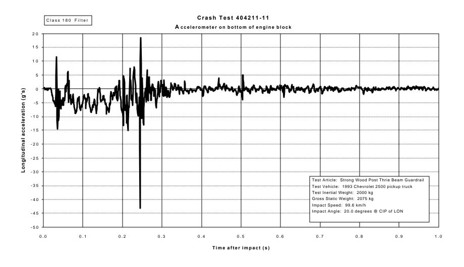
Figure 25. Vehicle longitudinal accelerometer trace for test 404211-11 (accelerometer located on bottom of engine block).
