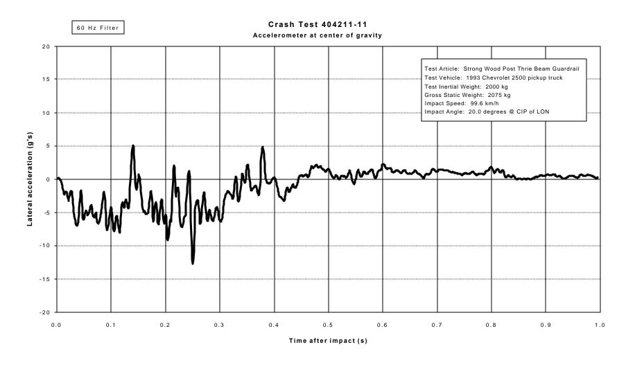
Figure 16. Vehicle lateral accelerometer traces for test 404211-11 (accelerometer located at center of gravity).
