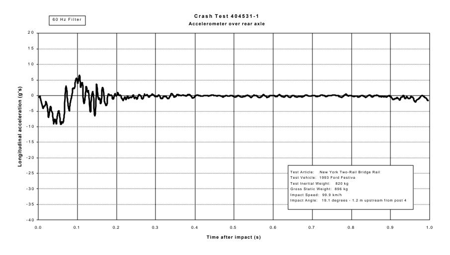
Figure 18. Vehicle longitudinal accelerometer trace for test 404531-1 (accelerometer located over rear axle).
