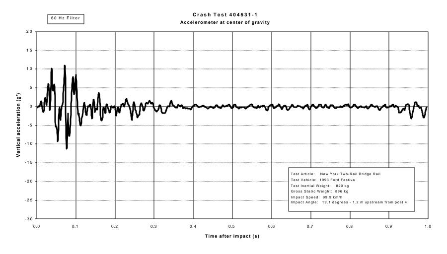
Figure 17. Vehicle vertical accelerometer trace for test 404531-1 (accelerometer located at center of gravity).
