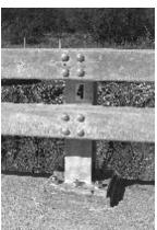
Figure 3. New York Two-Rail Curbless Bridge Railing prior to testing.
