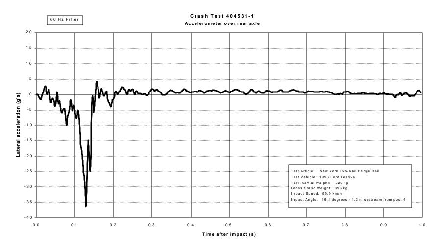
Figure 19. Vehicle lateral accelerometer trace for test 404531-1 (accelerometer located over rear axle).
