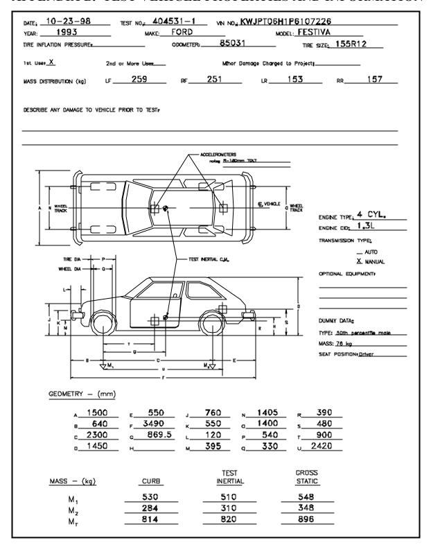
Figure 11. Vehicle properties for test 404531-1.
