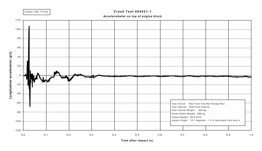
Figure 23. Vehicle longitudinal accelerometer trace for test 404531-1 (accelerometer located on top of engine block).
