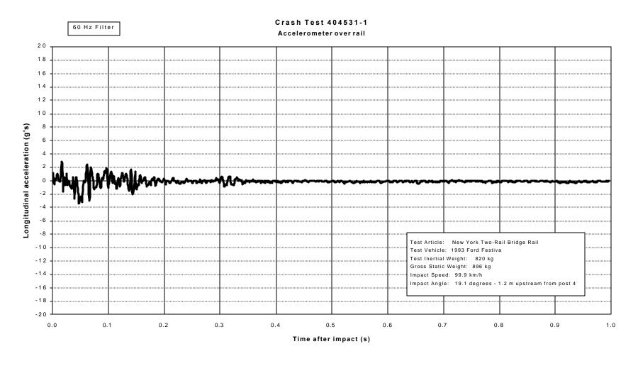
Figure 25. Bridge railing longitudinal accelerometer trace for test 404531-1 (accelerometer located over bridge railing at post 4).
