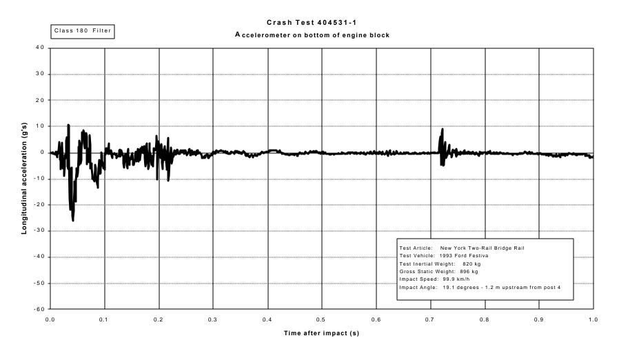
Figure 24. Vehicle longitudinal accelerometer trace for test 404531-1 (accelerometer located on bottom of engine block).
