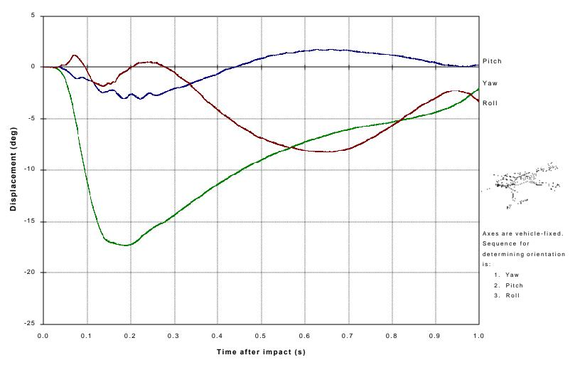
Figure 14. Vehicular angular displacements for test 404531-1.
