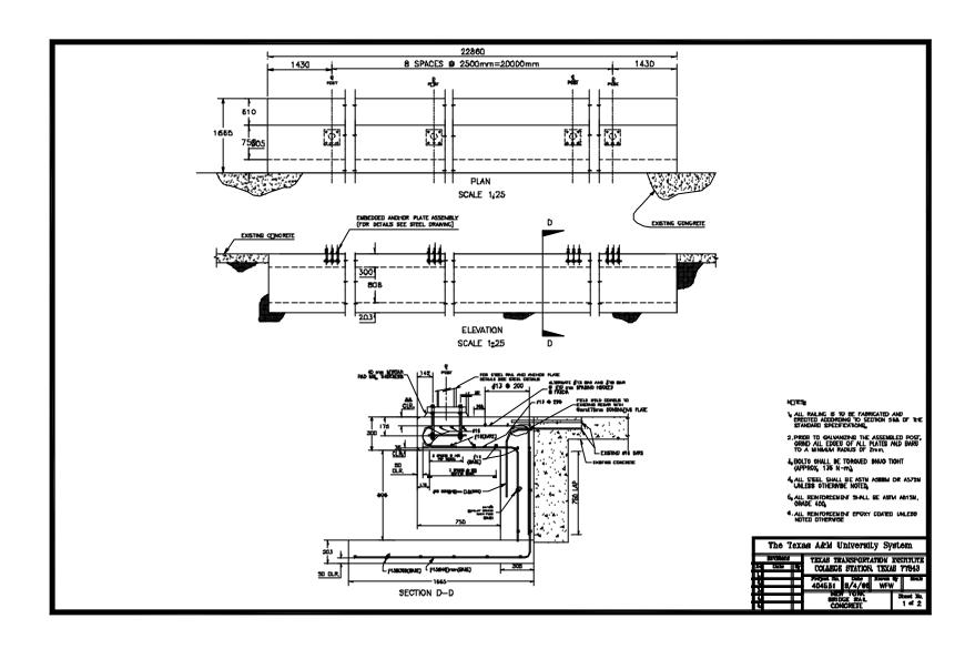
Figure 1. Details of the New York Curbless Two-Rail Bridge Railing for test 404531-1.
