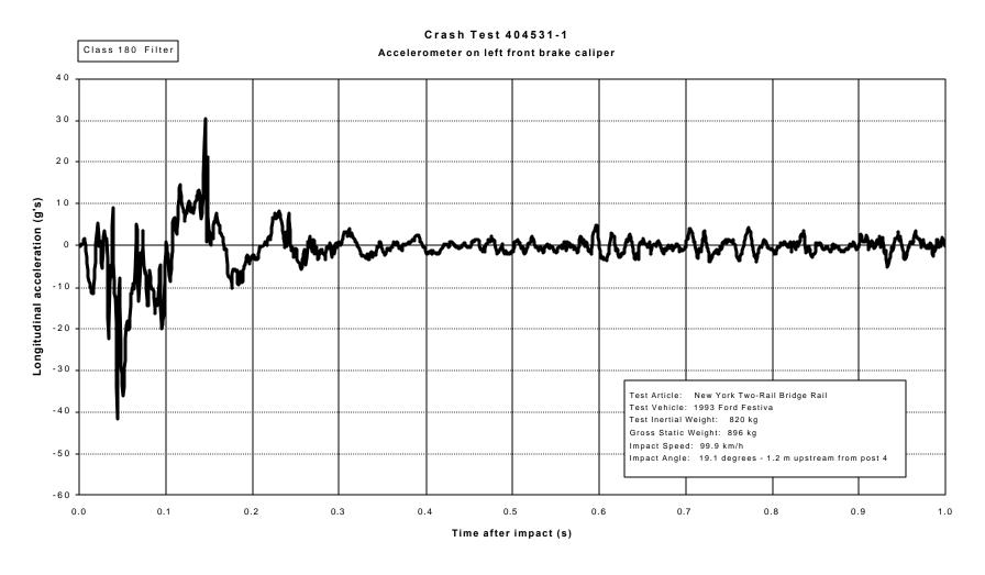
Figure 22. Vehicle longitudinal accelerometer trace for test 404531-1 (accelerometer located on left front brake caliper).
