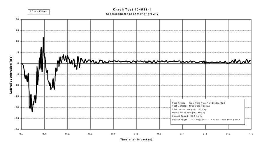
Figure 16. Vehicle lateral accelerometer trace for test 404531-1 (accelerometer located at center of gravity).
