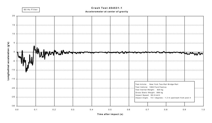
Figure 15. Vehicle longitudinal accelerometer trace for test 404531-1 (accelerometer located at center of gravity).
