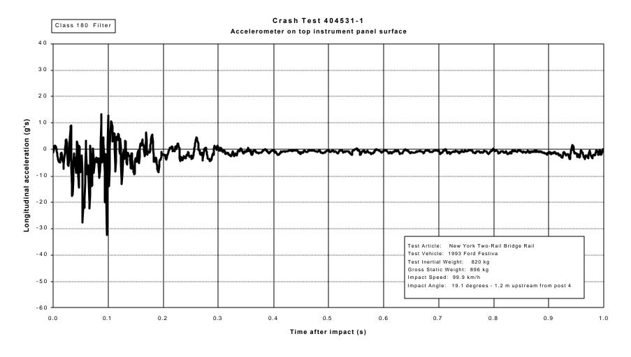
Figure 20. Vehicle longitudinal accelerometer trace for test 404531-1 (accelerometer located on top surface of instrument panel).
