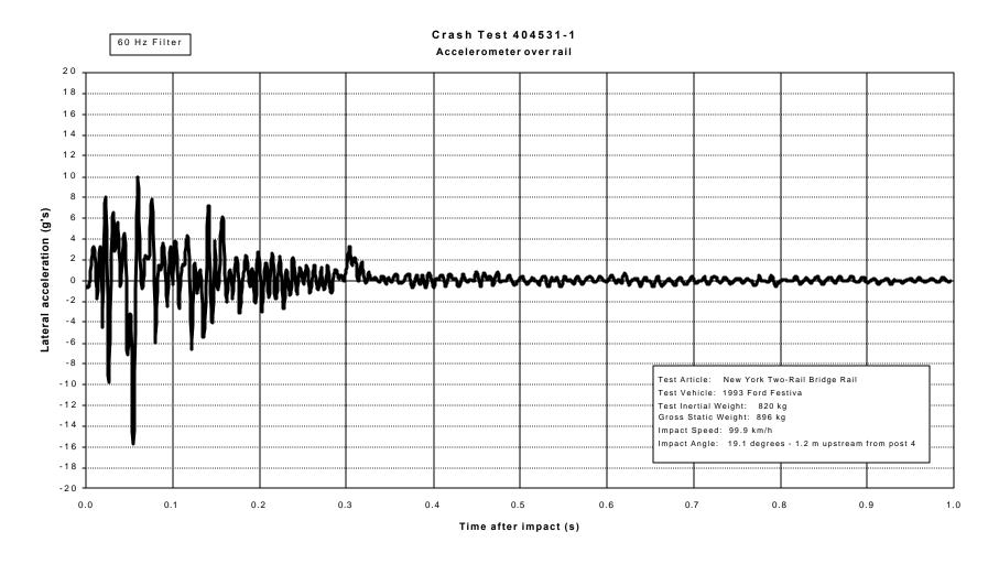
Figure 26. Bridge railing lateral accelerometer trace for test 404531-1 (accelerometer located over bridge railing at post 4).
