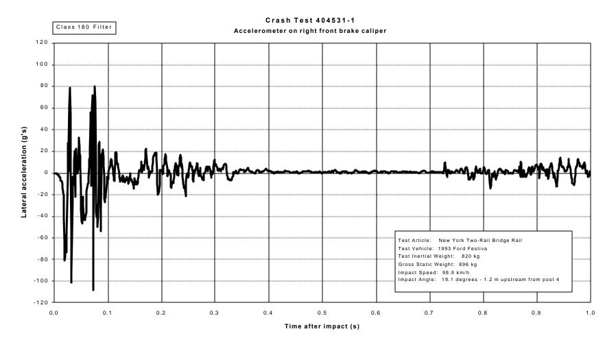
Figure 21. Vehicle lateral accelerometer trace for test 404531-1 (accelerometer located on right front brake caliper).
