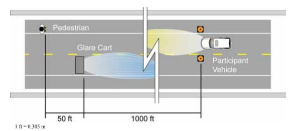
Figure 9. Diagram. Plan view of the participant vehicle at the start point for the disability glare portion with right pedestrian.
