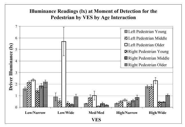
Figure 14. Bar graph. Mean illuminance readings (lx) at moment of detection for the Pedestrian by VES by Age interaction.
