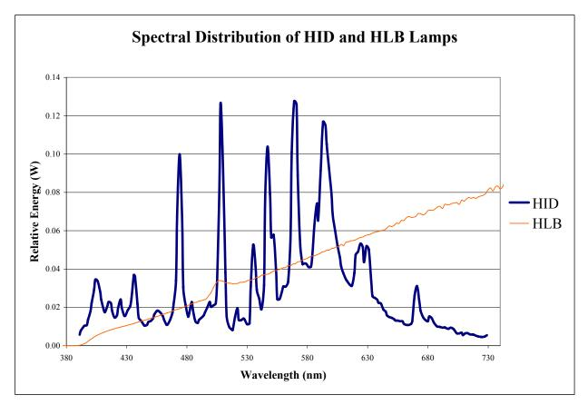
Figure 1. Line graph. Spectral power distribution of typical HID and halogen headlamps.
