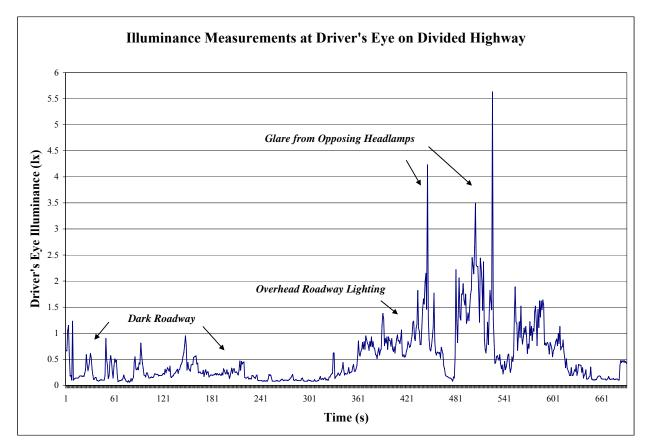
Figure 2. Line graph. Illuminance readings taken on a divided highway at night with and without overhead lighting and glare.
