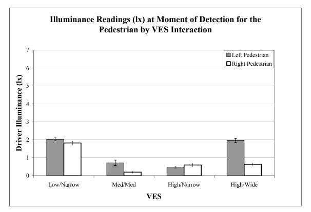
Figure 28. Bar graph. Mean illuminance readings (lx) at moment of detection for the Pedestrian by VES interaction without the low/wide VES.
