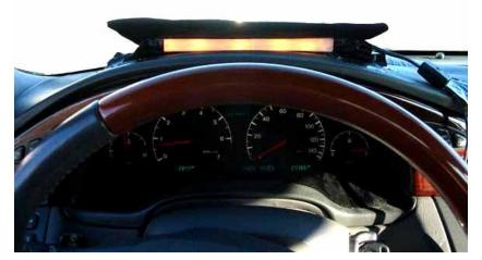
Figure 3. Photo. Light source used to control driver light adaptation level.
