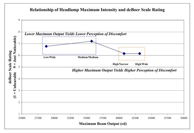
Figure 21. Line graph. The relationship between headlamp intensity and perceived glare.
