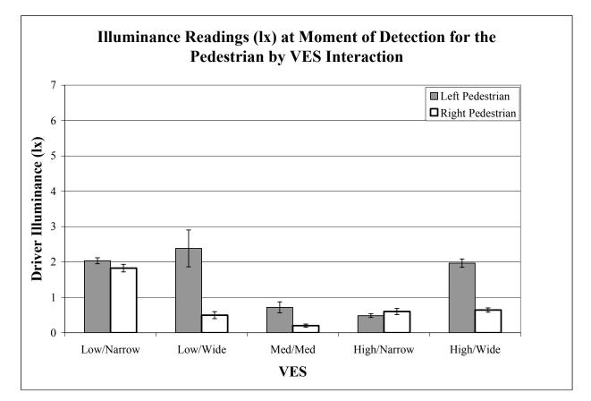
Figure 17. Bar graph. Mean illuminance readings (lx) at moment of detection for the Pedestrian by VES interaction.
