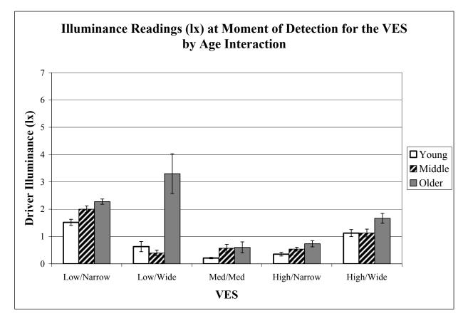
Figure 15. Bar graph. Mean illuminance readings (lx) at moment of detection for the VES by Age interaction.
