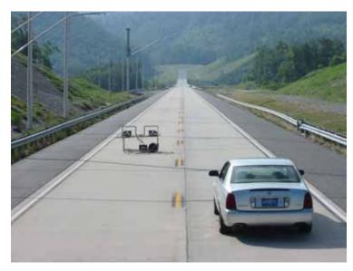
Figure 6. Photo. Glare cart and experimental vehicle on the Smart Road.
