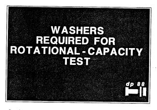
Washers are required for the R-C tests even though they may not be required for job-site installation. Where washers are not required for job-site installation, lot identification (both manufacturer and R-C) is not required. Washer coating should be the same as in the bolt and nut. All R-C tests are to be performed by the contractor/fabricator and should be witnessed by the DOT inspector.
