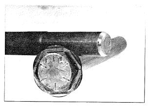
Next, the length of shank to be threaded is extruded to the thread pitch diameter (as shown on the upper bolt). The bolt then moves to the trimming station where a trimming die shears material from the circumference to form the hex shape (the bottom bolt).
