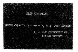
The installed bolt tension applies a clamping force to the plates in the connection. The plates will not slip relative to one another until the friction capacity is exceeded. The sum of the bolt tensions in the connection times the slip coefficient of the plate surfaces in contact (the faying surfaces), equals the slip load of the connection. Proper bolt tension is required for the connection to attain the design slip capacity.
