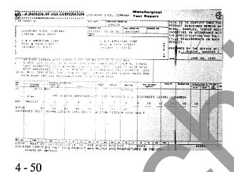
The Mill Test Report is furnished by the mill supplier. It contains records of mill heat number and chemical test results.
