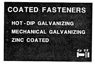
The A325 specification specifically refers to two processes for zinc coated fasteners, hot-dip and mechanically galvanized. Other methods of applying the zinc coatings are available.
