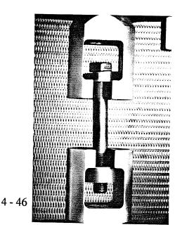
Wedge tension tests demonstrate bolt strength, ductility, and integrity of the head/shank junction. The tapered wedge adds significantly to the severity of the test.
