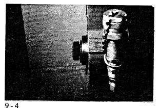
The performance of the DTIs should be checked in the field before the start of bolting. A tension measuring device is used along with a special adaptor at the bolt head. This adaptor replaces the normal piece used to prevent bolt head rotation.
