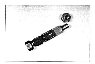
Nut threads are checked with a go/no-go gage.
