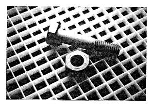
The fastener is then blasted to a "white metal" specification using a fine grit.
