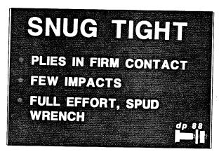
Bolts shall be installed in all holes of the connection and brought to a "snug tight" condition. Snug tight is defined as the tightness that exists when the plies of the joint are in firm contact. This may be attained by a few impacts of an impact wrench or the full effort of a man using an ordinary spud wrench.
