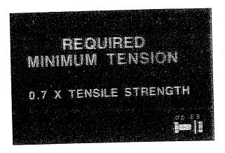
High-strength bolts used in bridge construction are required to be installed to an initial pretension equal to or greater than 0.7 tines their tensile strength. Note that the requirement is bolt tension, not a particular torque value. Torque may be used only if the requirements for calibrated wrench installation are followed.
