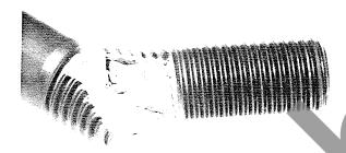
Wedge tension test failure must occur in the body or threaded section of the bolt. It may not occur at the head/shank junction, in spite of local bending due to the tapered wedge.
