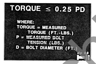
• 6 - Torque cannot exceed value calculated from this formula. P value used in this calculation is the "turn test tension" from table D4.1g of FHWA memo.
