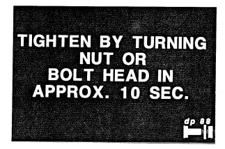
Tightening may be done by turning the bolt while the nut is prevented from rotating when it is impractical to turn the nut. Impact wrenches, if used, shall be of adequate capacity and sufficiently supplied with air to perform the required tightening of each bolt in approximately 10 seconds.
