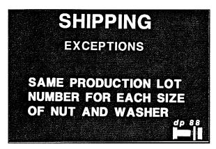
Each container is marked with rotational-capacity lot number and adequately identified.
