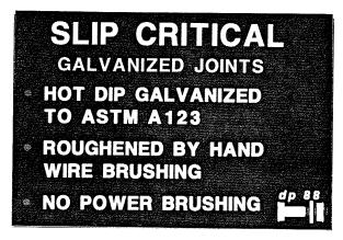
Faying surfaces specified to be galvanized shall be hot dip galvanized in accordance with ASTM Specification A123, and shall subsequently be roughened by means of hand wire brushing. Power wire brushing is not permitted.
