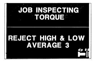
The job inspecting torque shall be taken as the average of three values thus determined after rejecting the high and low values.
