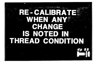
Wrenches shall be recalibrated when significant difference is noted in the surface condition of the bolt threads, nuts or washers. Recalibration is also required when fasteners are installed which may have been cleaned and/or relubricated.
