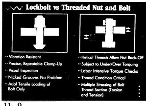
Many comparisons have been made between swage lock fasteners and threaded bolt/nut systems. There are significant differences in the forces applied and the action of their application to fastener components.
