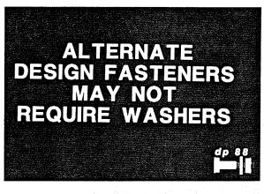
Alternate design fasteners with a geometry which provides a bearing circle on the head or nut with a diameter equal to or greater than the diameter of hardened washers meeting the requirements ASTM F436 satisfy the requirements for washers.
