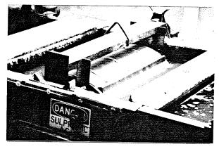
Parts are first cleaned in a sulfuric acid bath. They are then loaded into the barrel.
