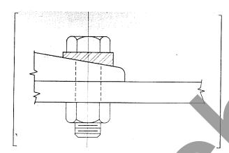
Where the outer face of the bolted parts has a slope greater than 1:20 with respect to a plane normal to the bolt axis, a hardened beveled washer shall be used to compensate for the lack of parallelism.
