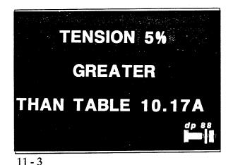
The test assembly shall include flat hardened washers, if required in the actual connection, arranged as in the actual connections to be tensioned. The calibration test shall demonstrate that each bolt develops a tension not less than 5 percent greater than the tension required by Table #. A. Manufacturer's installation procedure as required by Article #.326 shall be followed for installation of bolts in the calibration device and in all connections.
