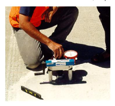
Figure 2. Commercially Available Tensile Bond Strength Test Device
