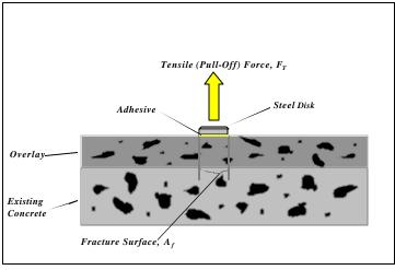
Figure 1. Schematic of Pull-Off Test Principle
