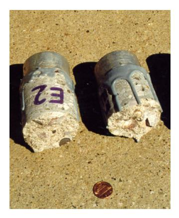
Figure 3. View of Fracture Surface of Tensile Cores
