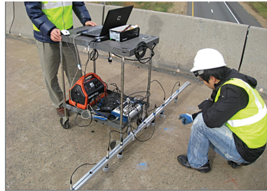
Figure 3. The contactless impact-echo scanning system.
