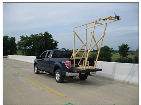
Figure 14. Three-dimensional optical bridge evaluation system.
