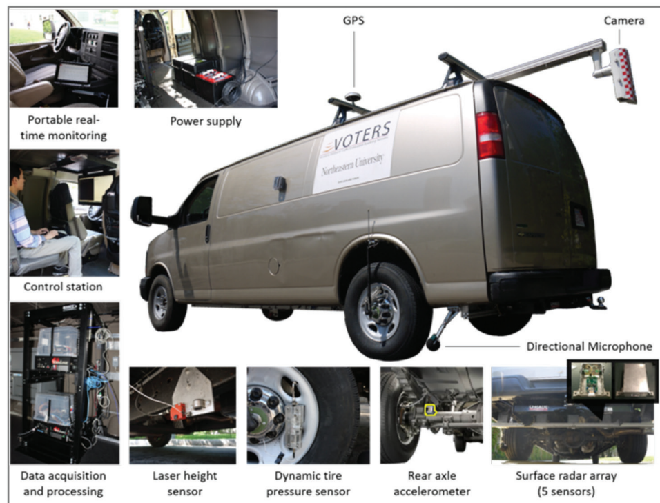
Figure 1. The versatile onboard traffic-embedded roaming sensors (VOTERS) test van.
