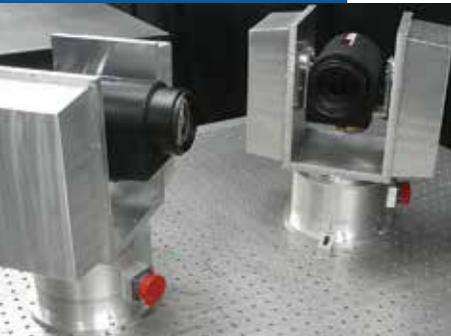
Cameras that can cooperate using precise and fast electronic pan, tilt, and zoom gimbals for event detection.
