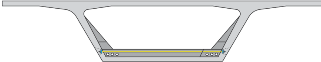
Figure 1.27 - Transverse Post-Tensioning in Deviator Ribs
