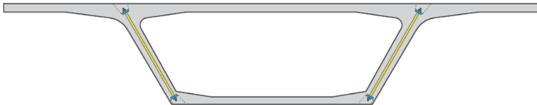
Figure 1.28 - Vertical Post-Tensioning in Webs
