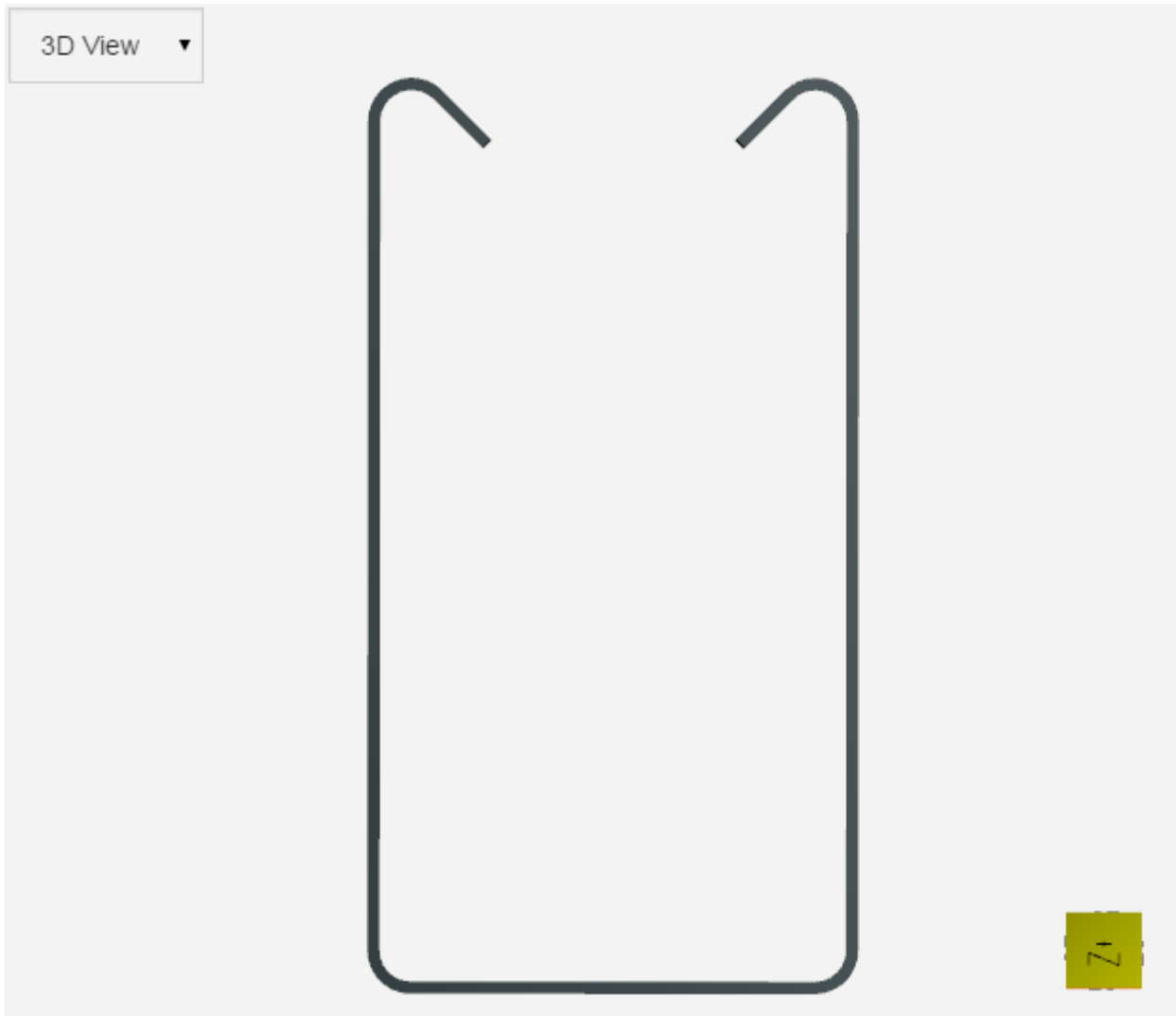
Figure 57 - Reinforcing Stirrup Bar Bend
