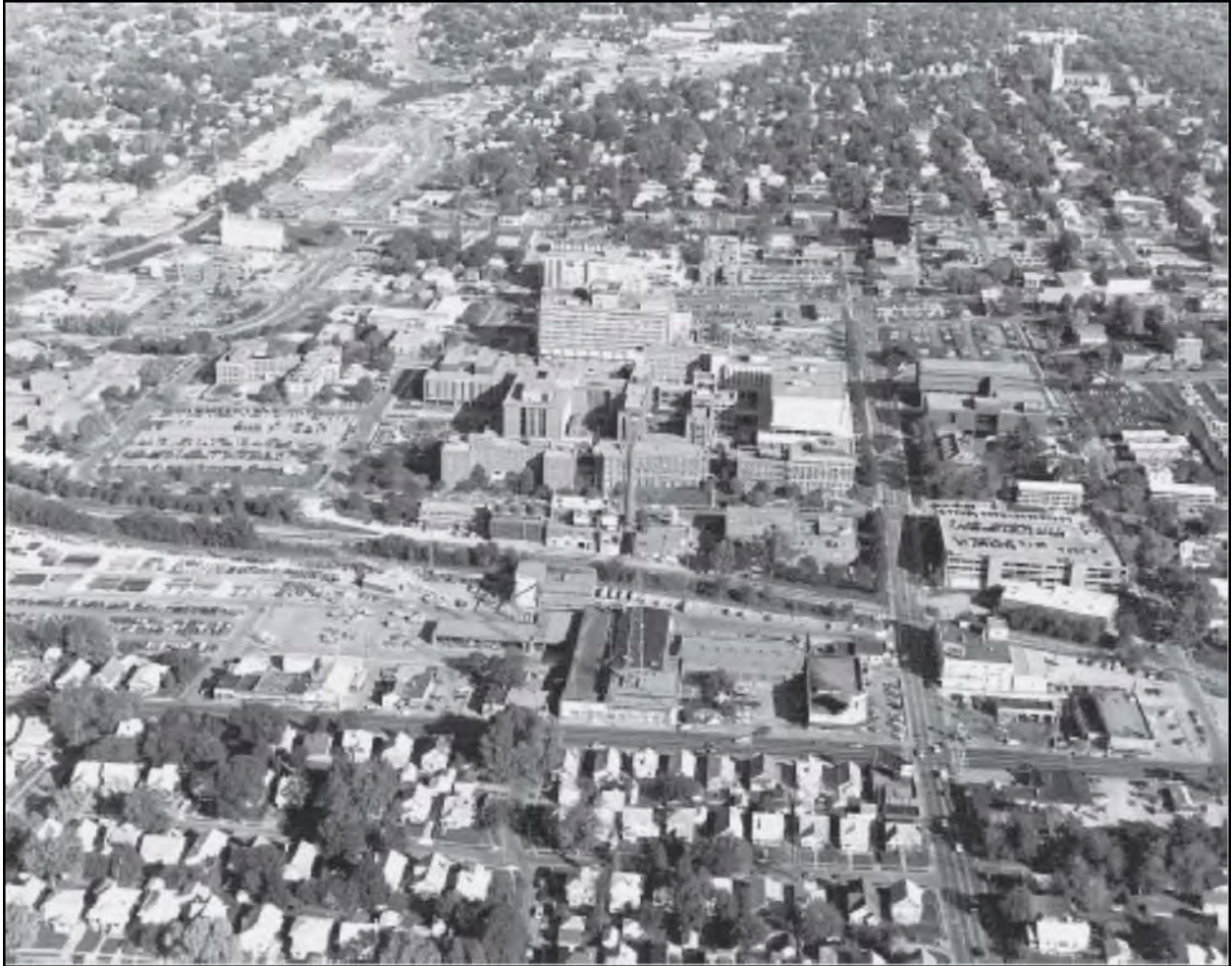
Figure 7-8 Exposure B - Urban Area with Numerous Closely Spaced Obstructions With Size of Single Family Dwellings or Larger (with permission from ASCE)
