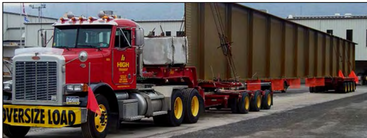
Figure 3-1 Bridge Plate Girder Loaded for Transport to Project Site
