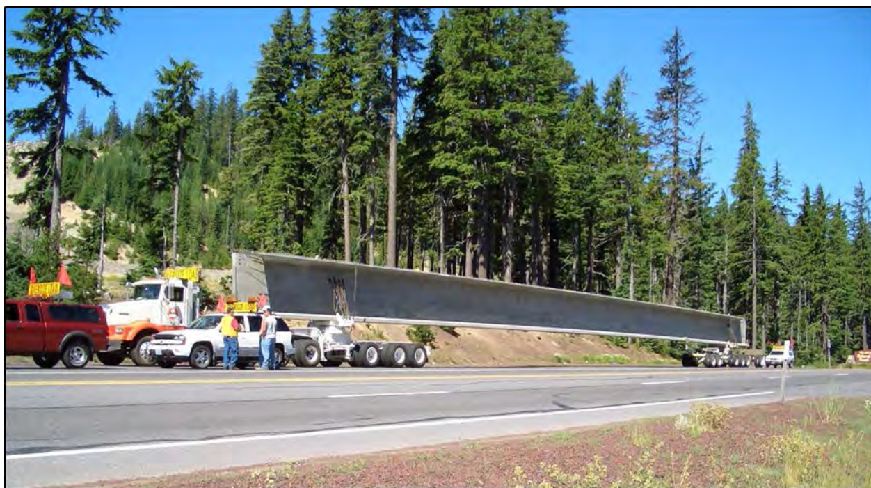
Figure 3-2 Concrete Girder in Transport with Escort Vehicles
