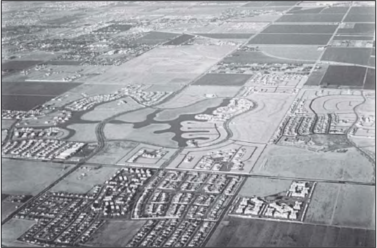
Figure 7-10 Exposure C - Open Terrain with Scattered Obstructions (with permission from ASCE)
