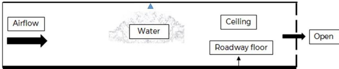
**Figure 3-30: Model schematic to examine water drop drift.**
