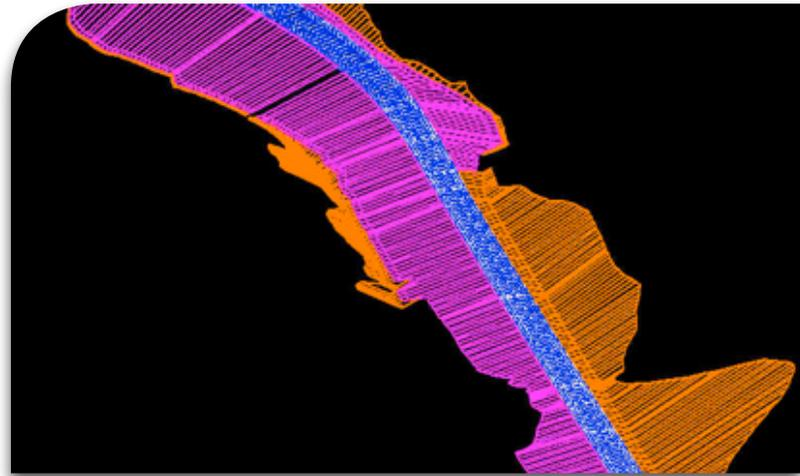
KYTC will develop and use 3D models for the proposed top surface and sub grade. The ultimate purpose of this process is to refine the way designers create the construction model so that it is more useful for contractors. The goals of this pilot project, as seen by KYTC, are to: 1) determine the best modeling practices for design, so better models can be provided to contractors in the future; and 2) set new policy to require better 3D models from design.
