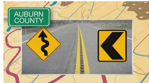
The county received funding and implemented low-cost strategies, such as warning signs, chevron signing, and raised pavement markers. The county even added non-traditional "curve ahead" pavement markings, including directional arrows as a
