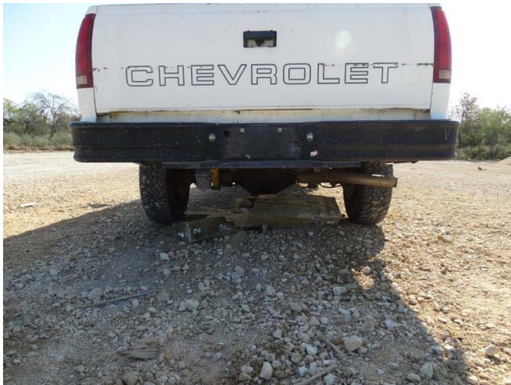
Figure 3.46: Post Test Vehicle – Accumulated Posts Located Under the Vehicle
