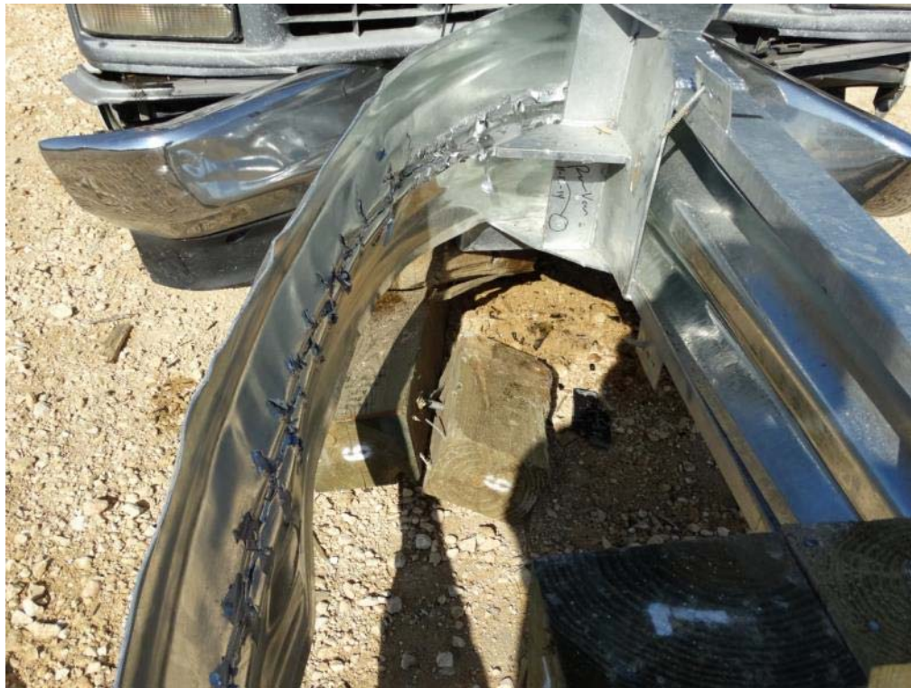
Figure 3.16: Post Test – Back Side of Extruder Head
