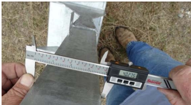
Figure 2.2: Measurement of Channel Width of Head
