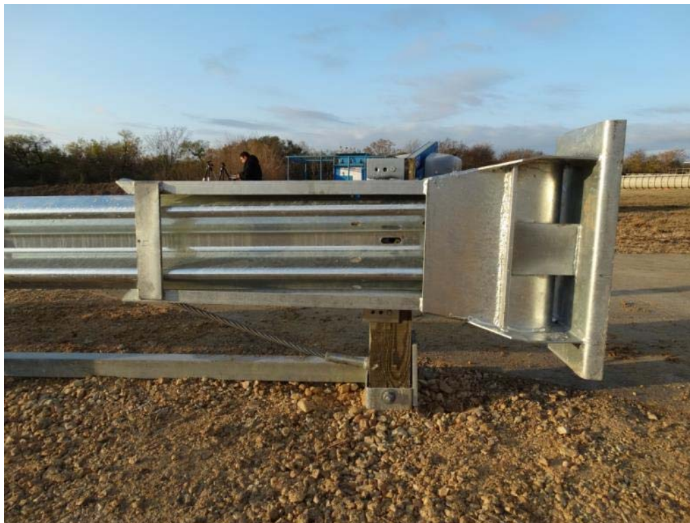
Figure 2.15: ET Plus Head and Post 1 – Traffic Side
