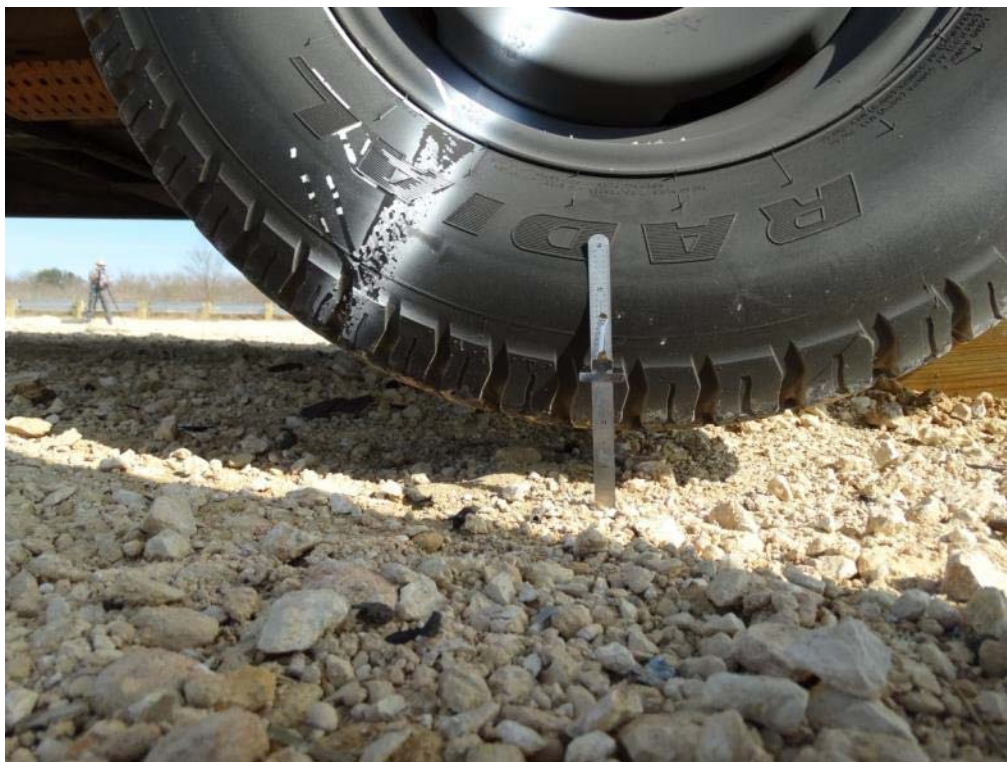
Figure 3.48: Post Test Vehicle – Accumulated Posts Lifted Vehicle
