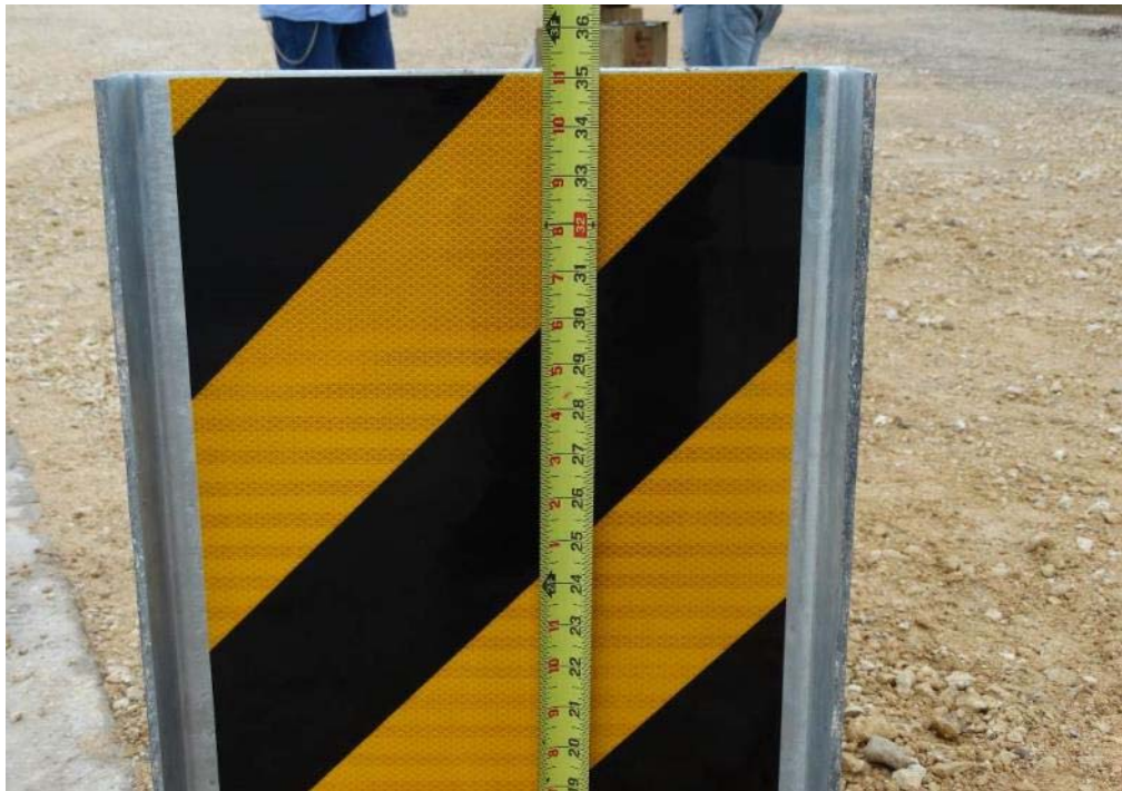
Figure 2.5: ET Plus Head Height Above Ground – Top
