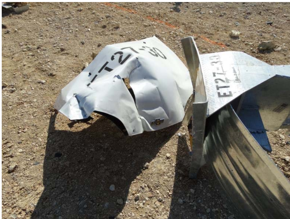
Figure 3.35: Damaged Test Vehicle – Front Hood
