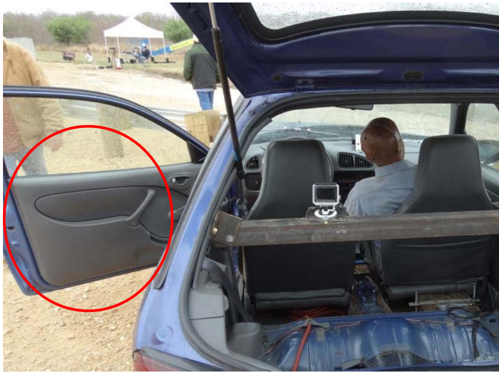
Figure 3.39: Damaged Test Vehicle – Door Panel Intact behind Exterior Tear
