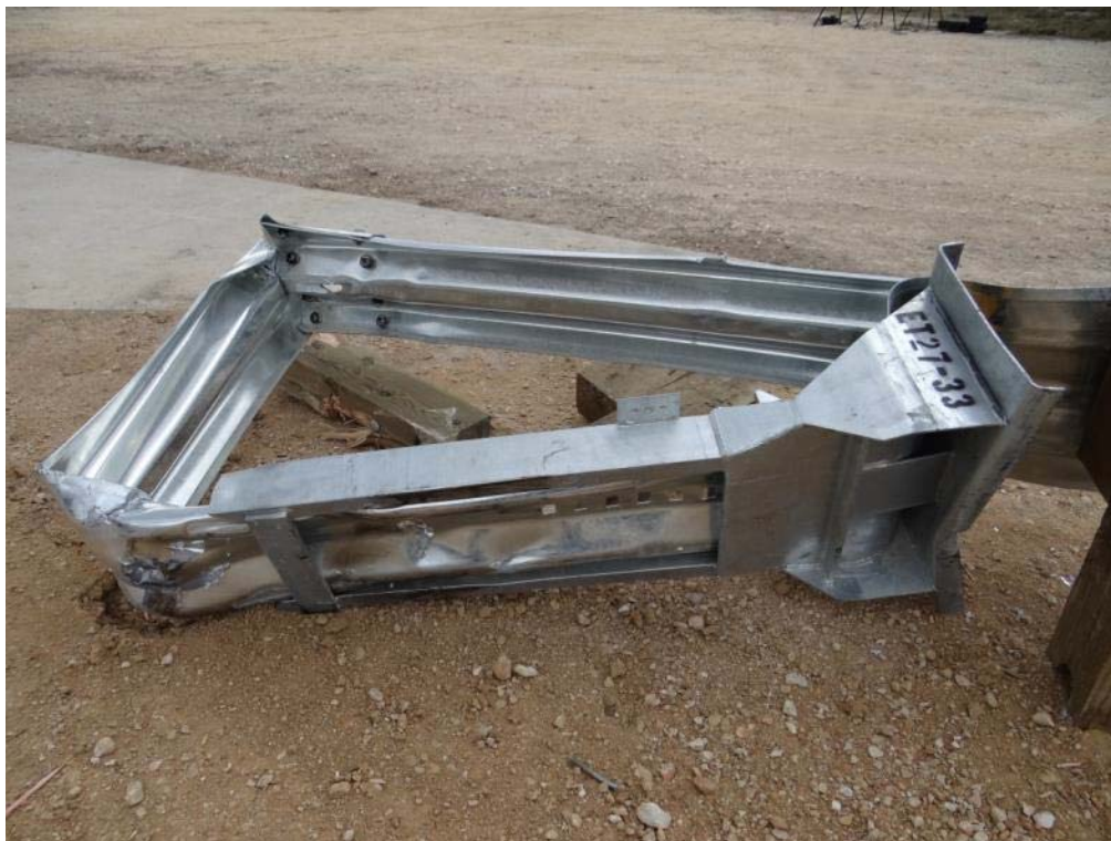
Figure 3.20: Post Test – Gated Guardrail
