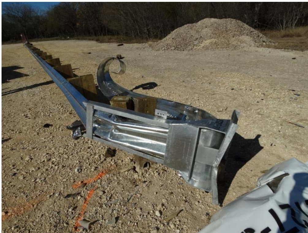
Figure 3.24: Post Test – Traffic Side View of Extruder Head
