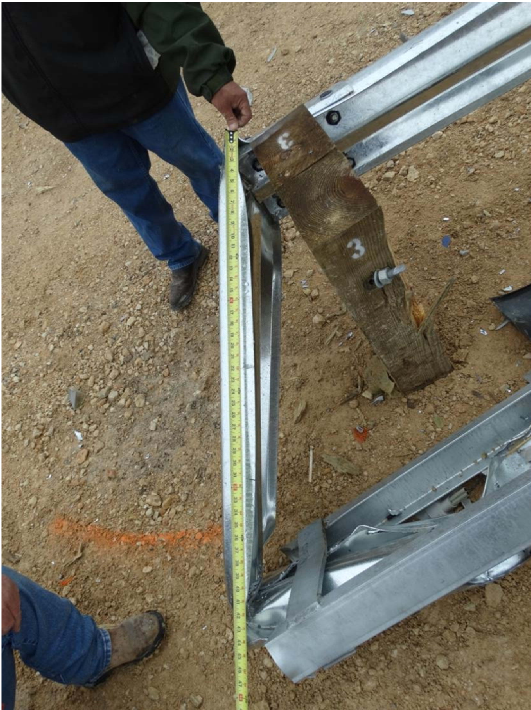
Figure 3.22: Post Test – Gated Guardrail
