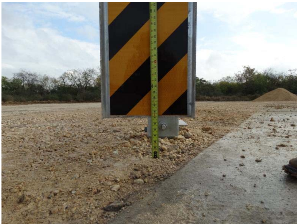
Figure 2.6: ET Plus Head Height Above Ground – Bottom
