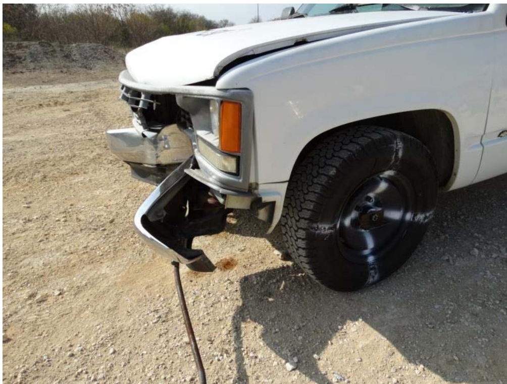
Figure 3.50: Post Test Vehicle – Left Side after Removal from Guardrail
