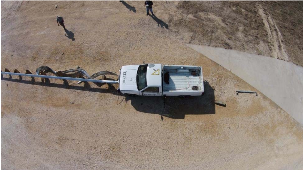
Figure 3.6: Post-Impact Condition of the Test Article and Vehicle
