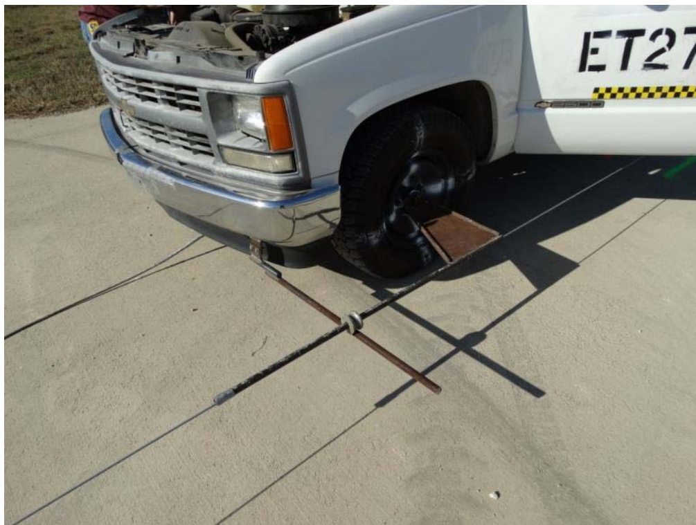
Figure 2.26: Test Vehicle Steering Guidance Assembly
