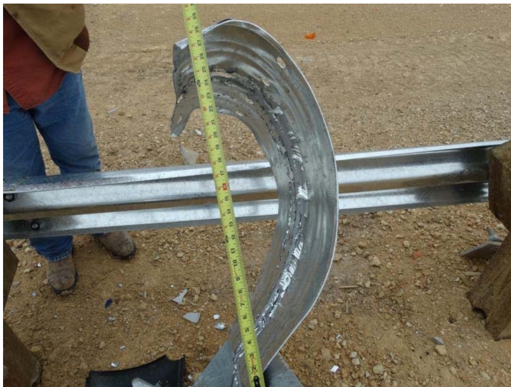
Figure 3.17: Post Test – Extruded Guardrail Tail
