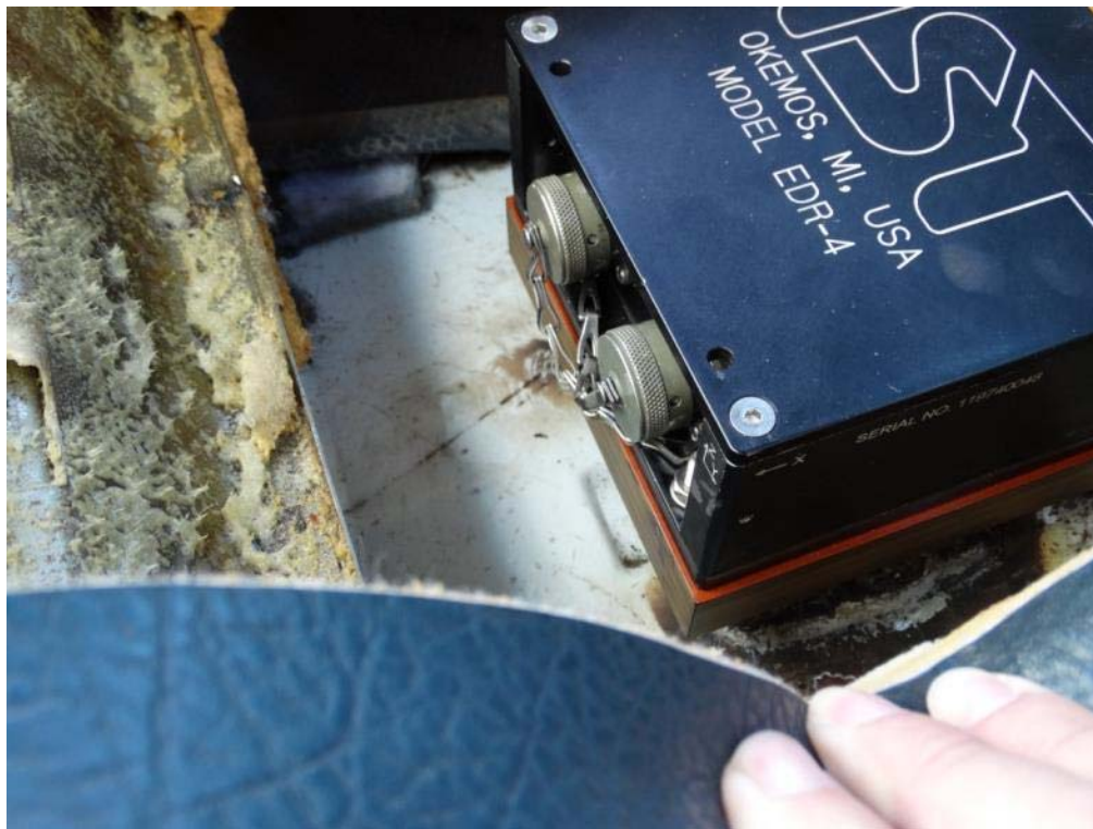
Figure 2.28: Close-up of EDR Mounted in Vehicle
