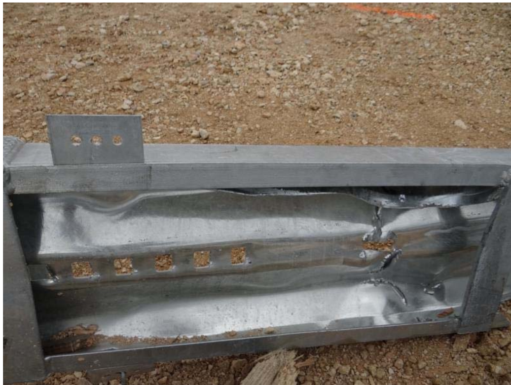
Figure 3.35: Post Test – ET Plus Head Guide Channel, Non-Traffic Side
