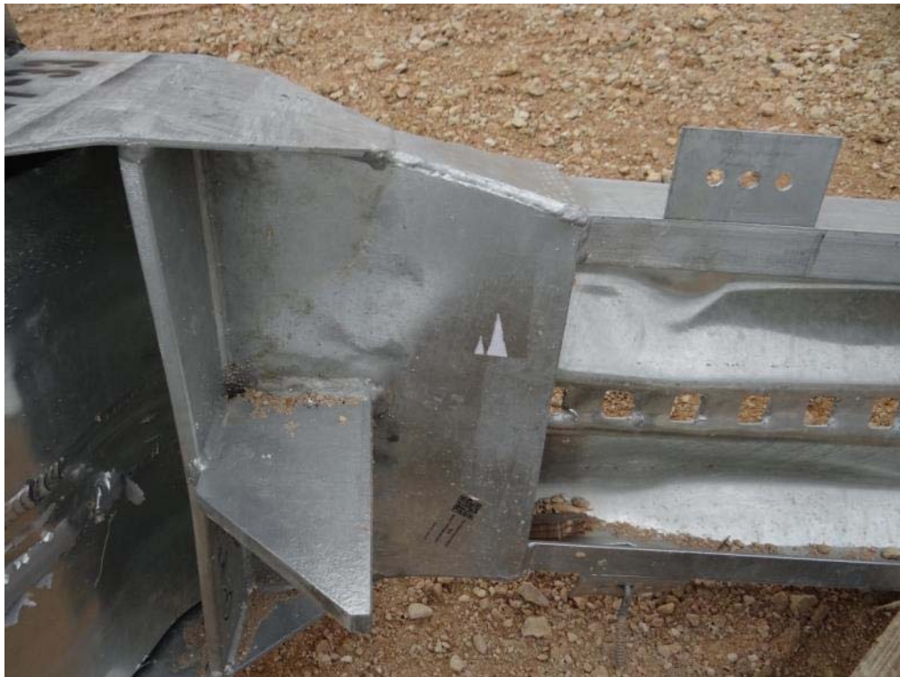
Figure 3.34: Post Test – ET Plus Head, Non-Traffic Side
