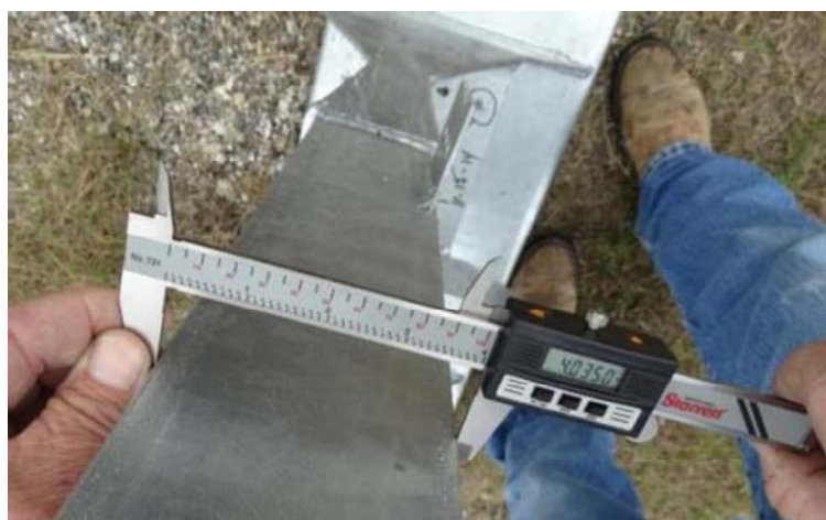
Figure 2.2: Measurement of Channel Width of Head
