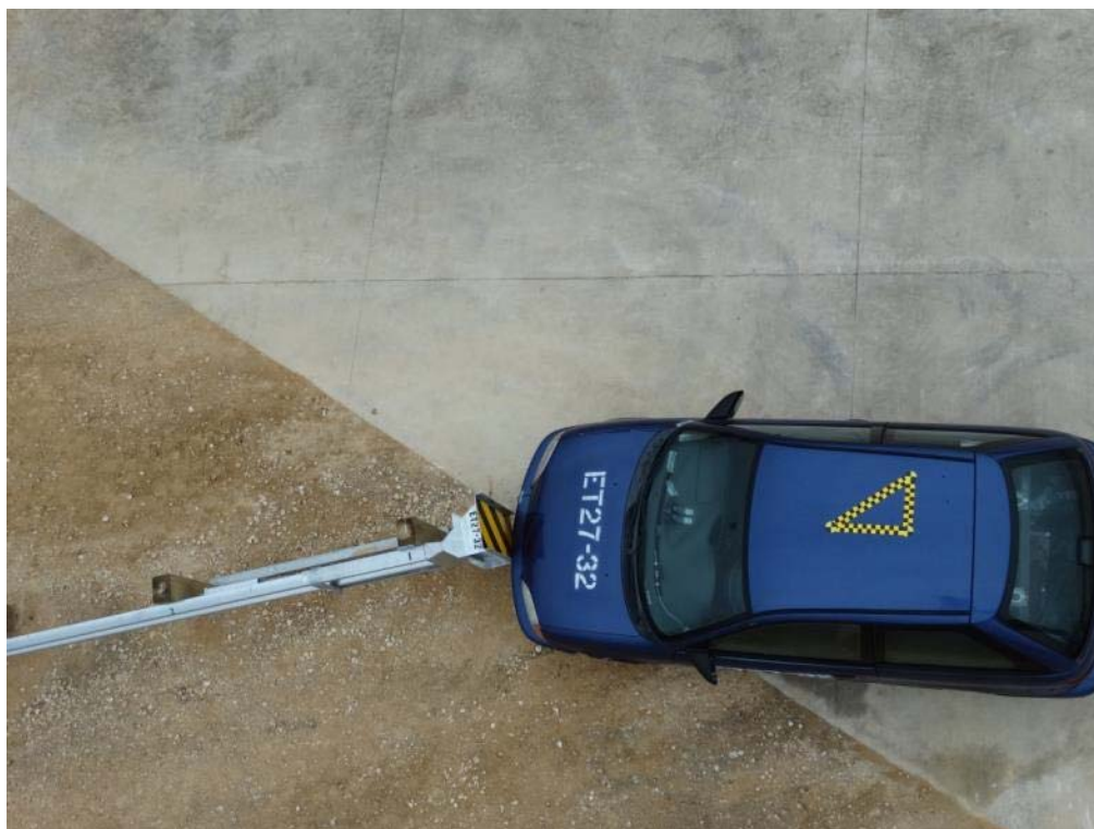
Figure 2.22: Test Vehicle Impact Trajectory – Overhead View
