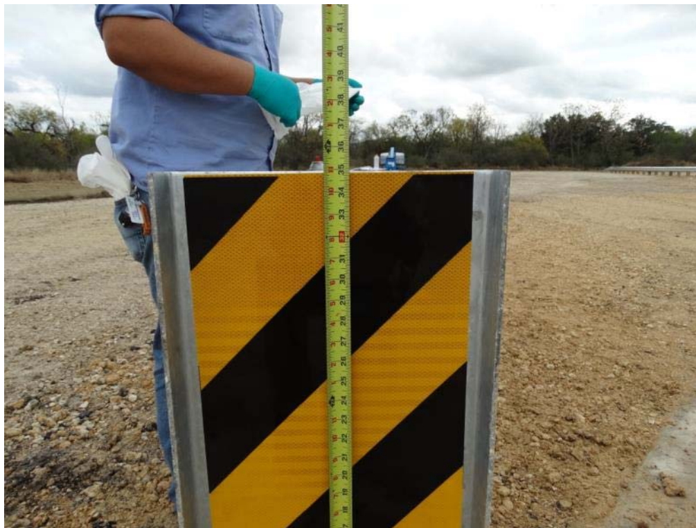
Figure 2.5: ET Plus Head Height Above Ground – Top
