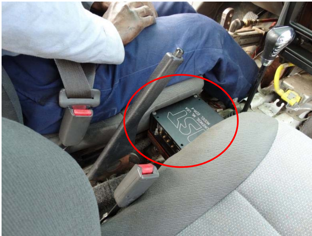
Figure 2.26: EDR Mounted in Test Vehicle for Test ET27-30
