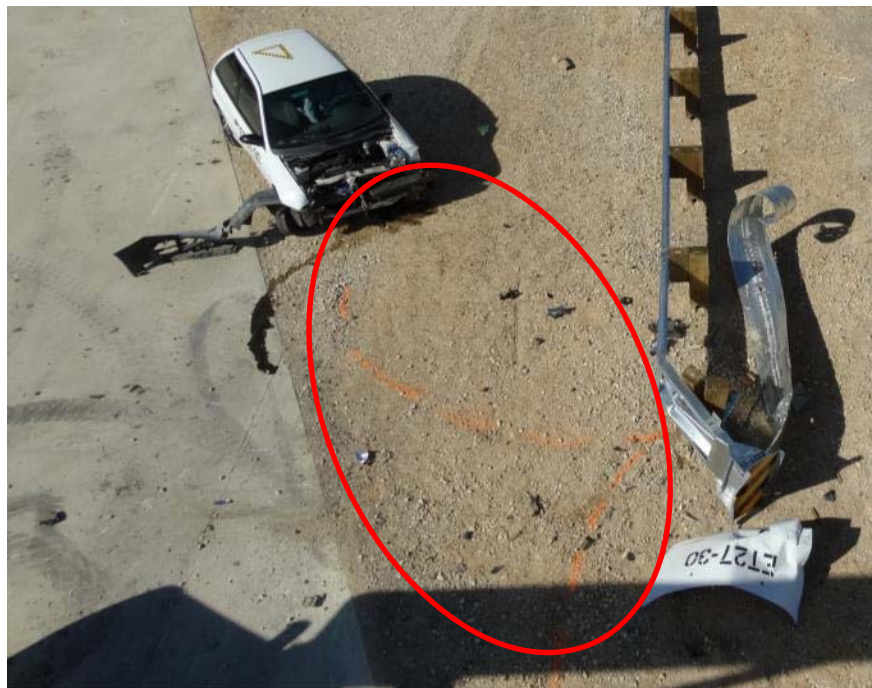
Figure 3.30: Test Vehicle Path of Left Front Tire (Orange Paint)
