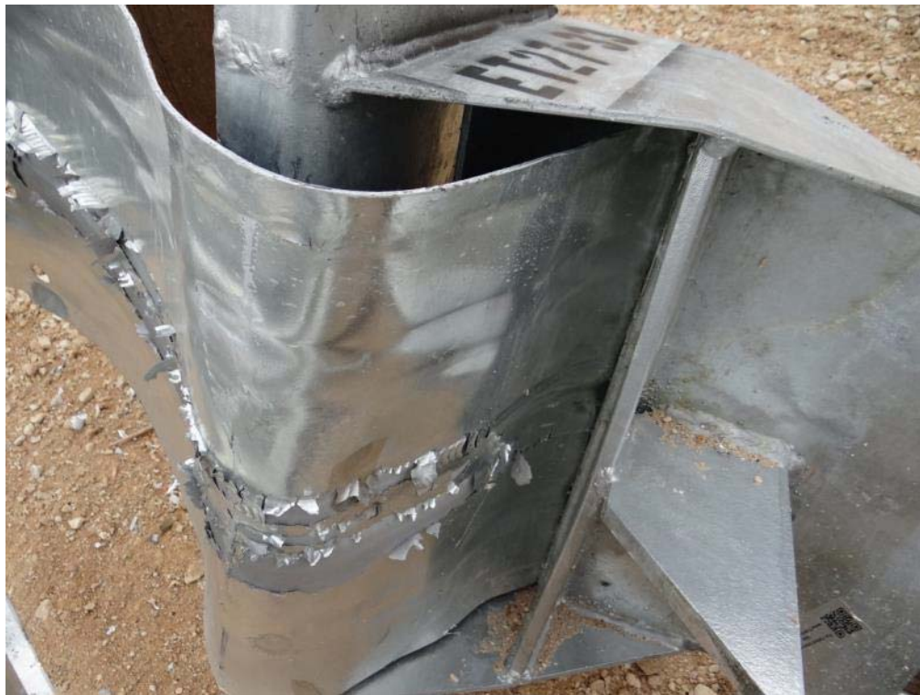
Figure 3.29: Post Test – Extruded W beam at Exit Chute
