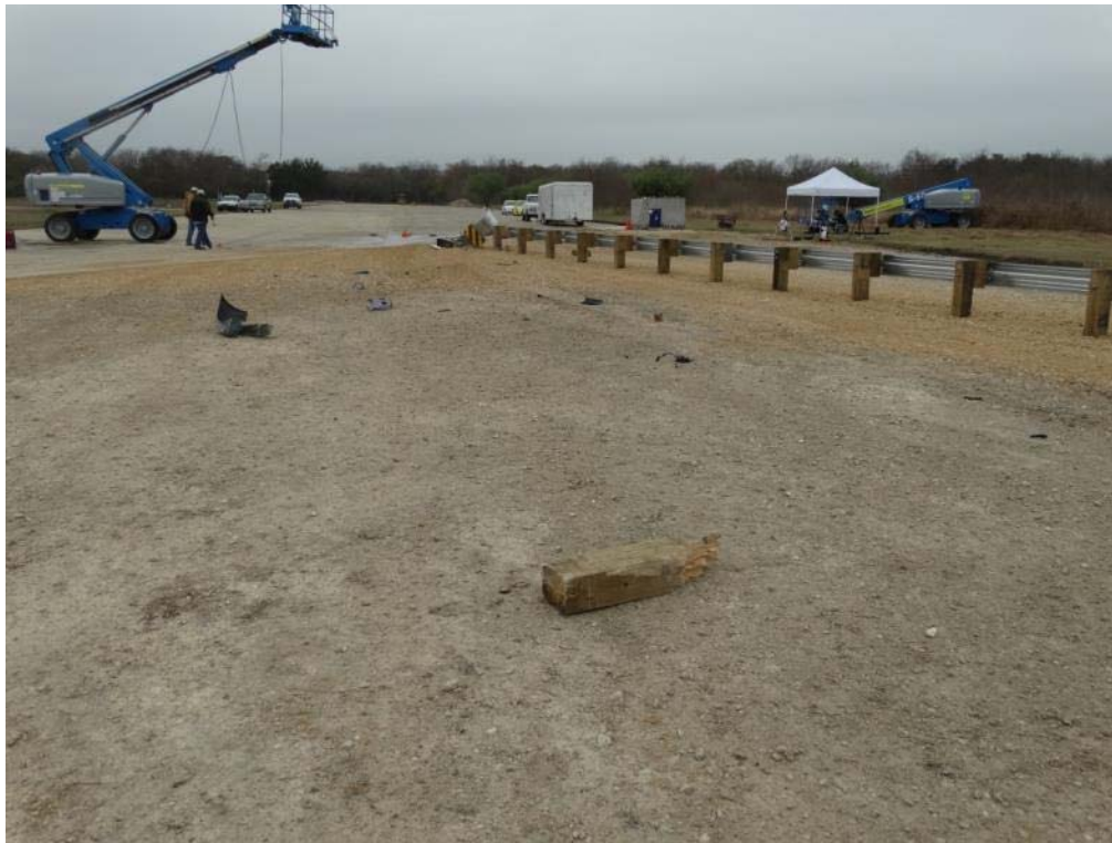
Figure 3.23: Post Test – Debris Field on Non-Traffic Side
