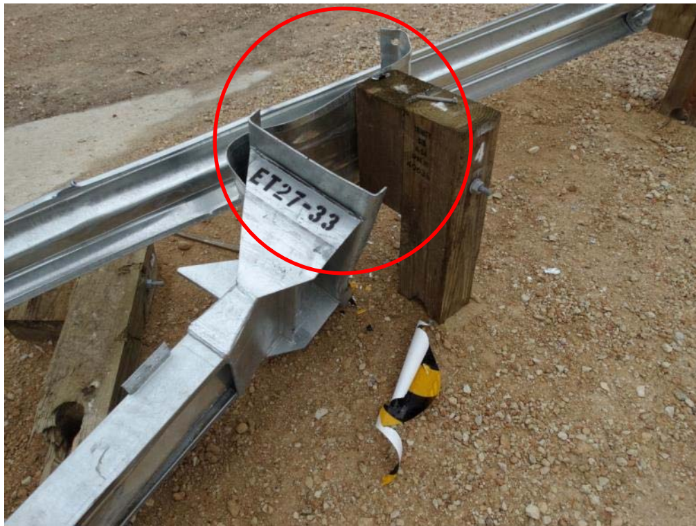
Figure 3.23: Post Test – Extruded W beam
