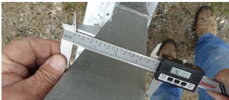
Figure 2.2: Measurement of Channel Width of Head
