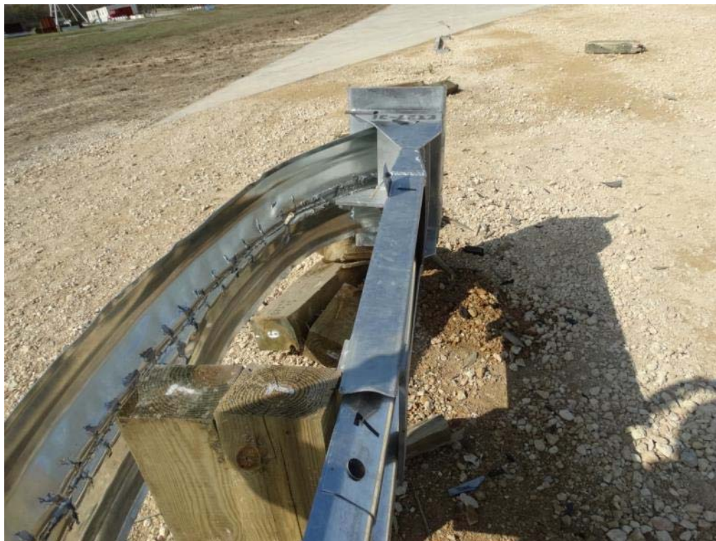
Figure 3.35: Post-Impact Test Article after Vehicle Removed – Rear View
