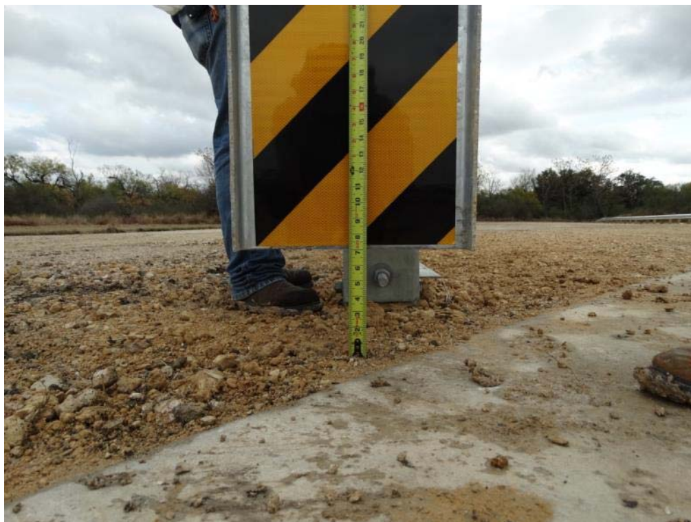
Figure 2.6: ET Plus Head Height Above Ground – Bottom
