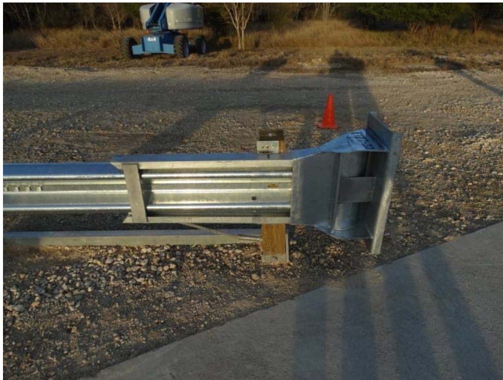
Figure 2.13: ET Plus Head and Post 1 – Traffic Side
