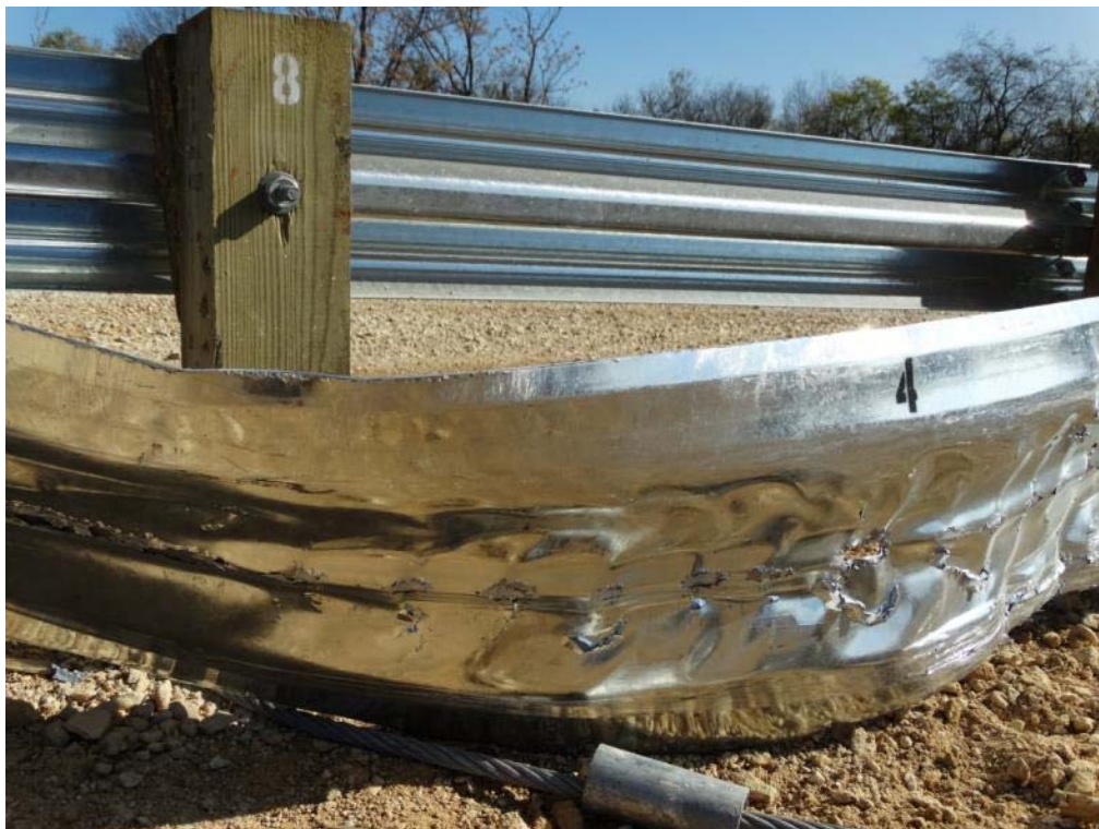
Figure 3.21: Post Test – Extruded Guardrail
