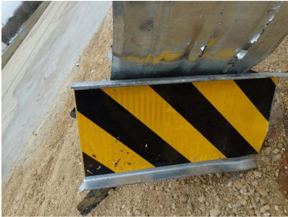
Figure 3.27: Post Test Terminal Extruder Head Impact Plate
