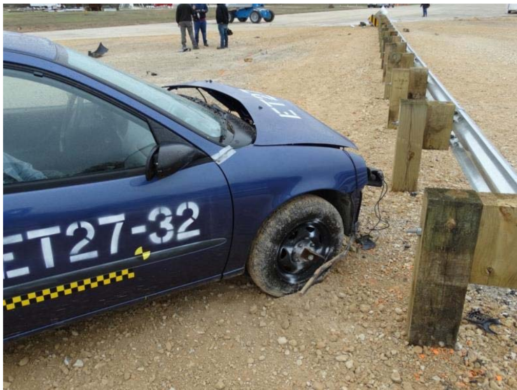
Figure 3.36: Damaged Test Vehicle – Right Side
