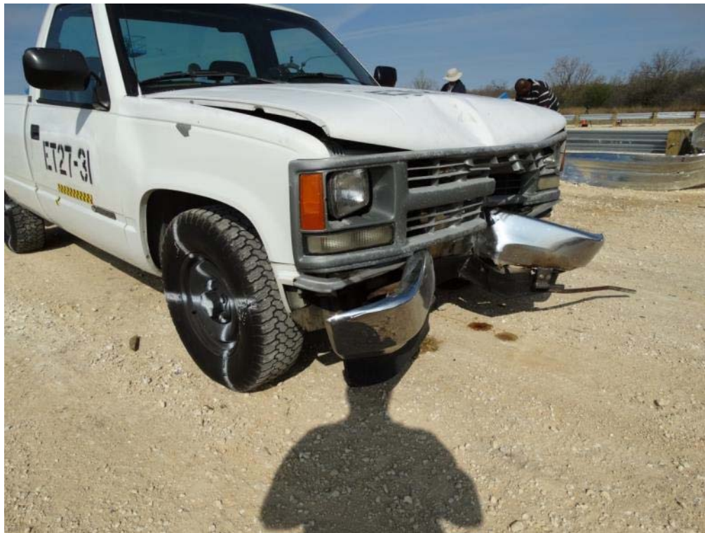
Figure 3.51: Post Test Vehicle – Right Side after Removal from Guardrail
