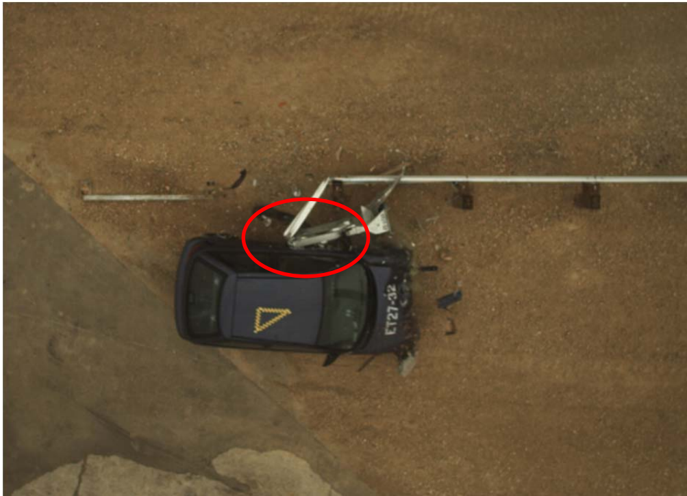
Figure 3.37: Guide Channel at Driver Side Door During Test
