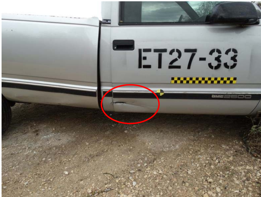
Figure 3.51: Damage to Passenger Door Caused by Steering Cable Rod
