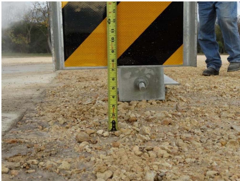
Figure 2.6: ET Plus Head Height Above Ground – Bottom
