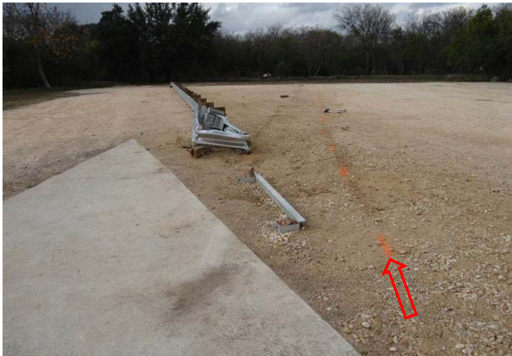
Figure 3.40: Post-Impact Path of Right Tire (Orange Paint)
