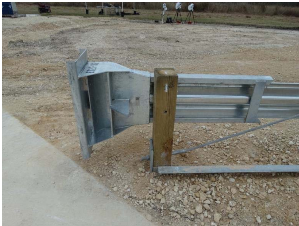
Figure 2.14: ET Plus Head and Post 1 – Non-Traffic Side
