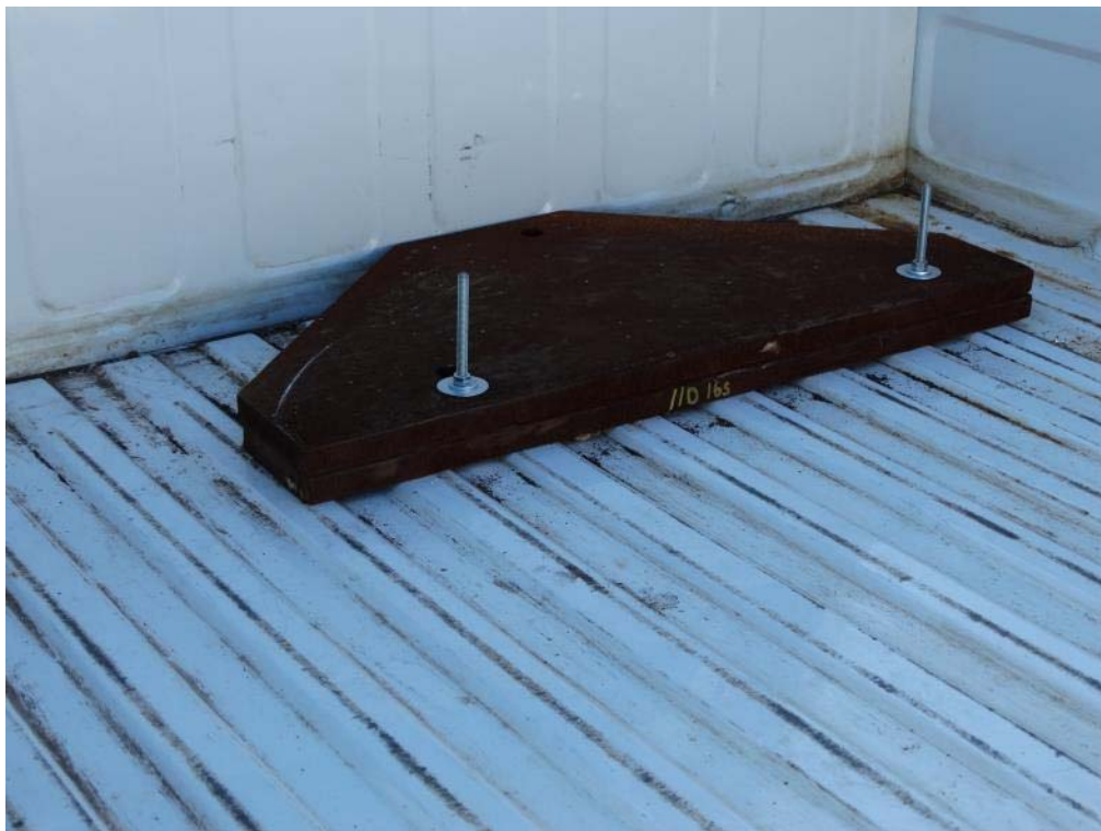
Figure 2.25: Test Vehicle Ballast
