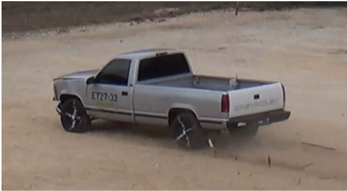
Figure 3.45: Left Side of Vehicle Following ET Plus Impact
