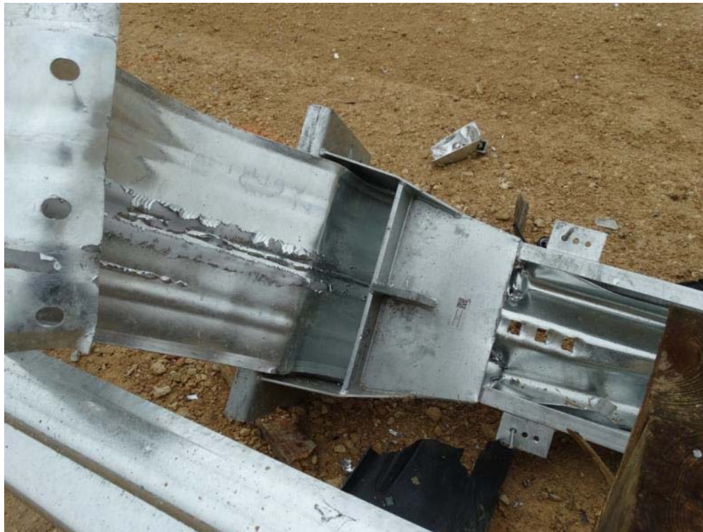
Figure 3.16: Post Test – Extruded Tail of W-Beam
