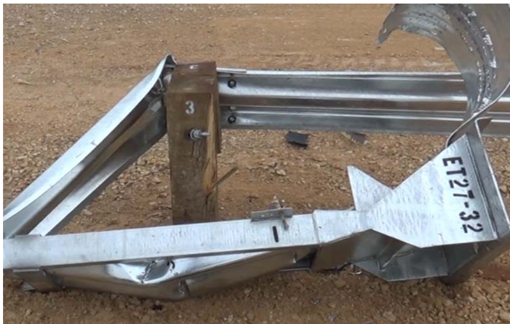
Figure 3.21: Post Test – Top View of Extruder Head
