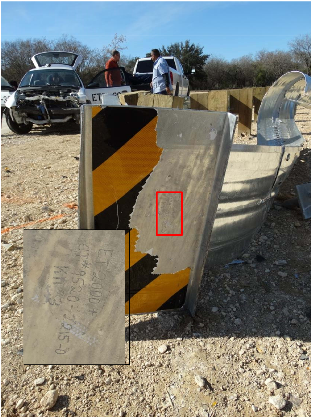
Figure 3.28: Post Test Verification of Extruder Head 3
