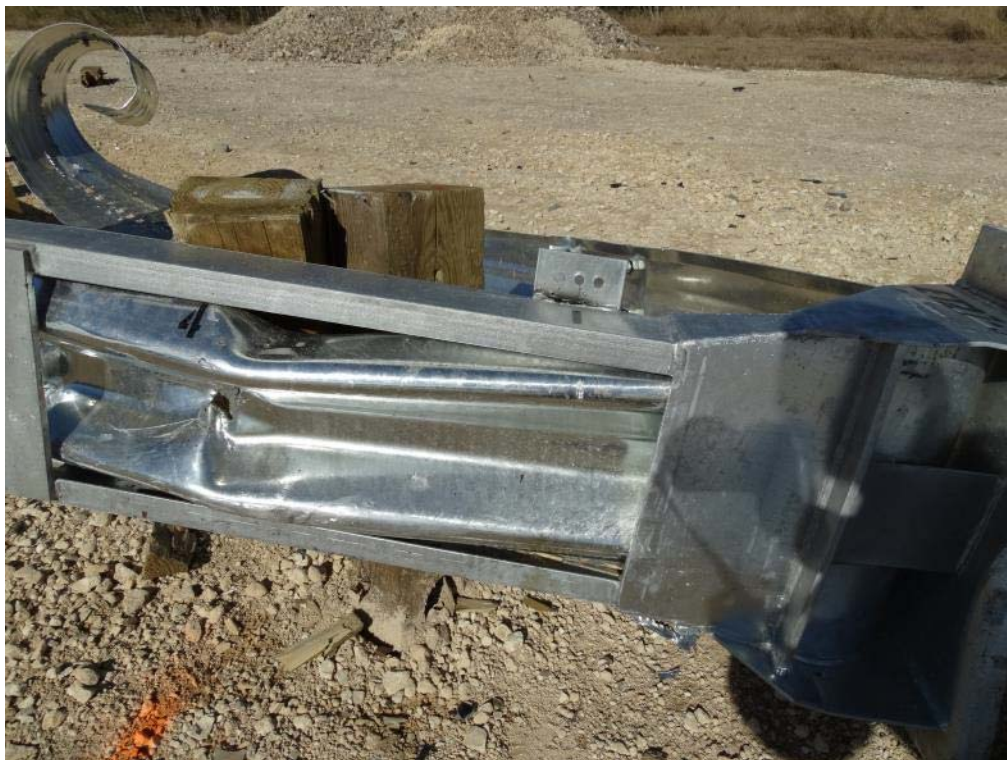
Figure 3.14: Post Test – Side View of Extruder Head
