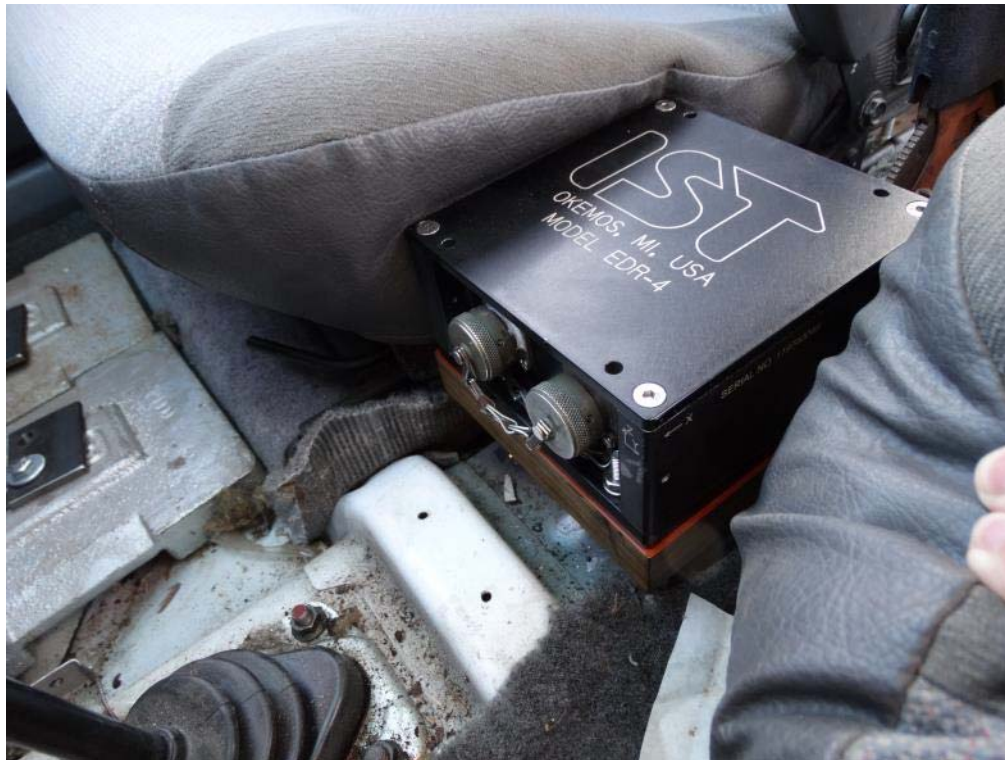
Figure 2.27: Close-up of EDR Mounted in Vehicle
