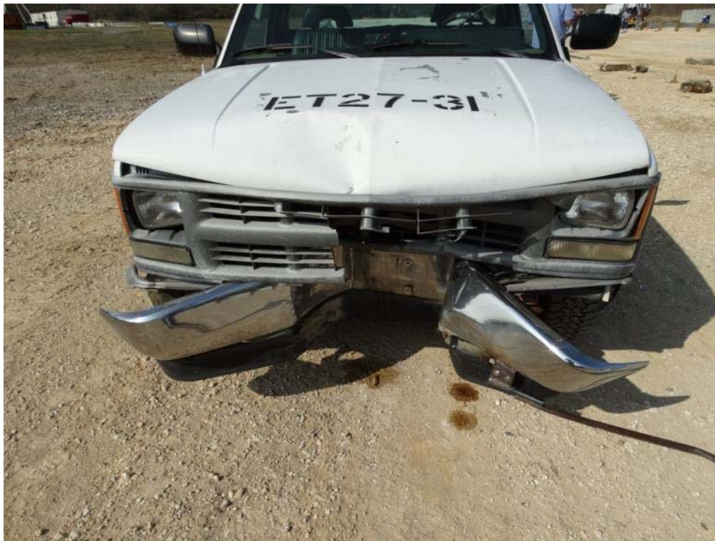
Figure 3.49: Post Test Vehicle – Front View after Removal from Guardrail
