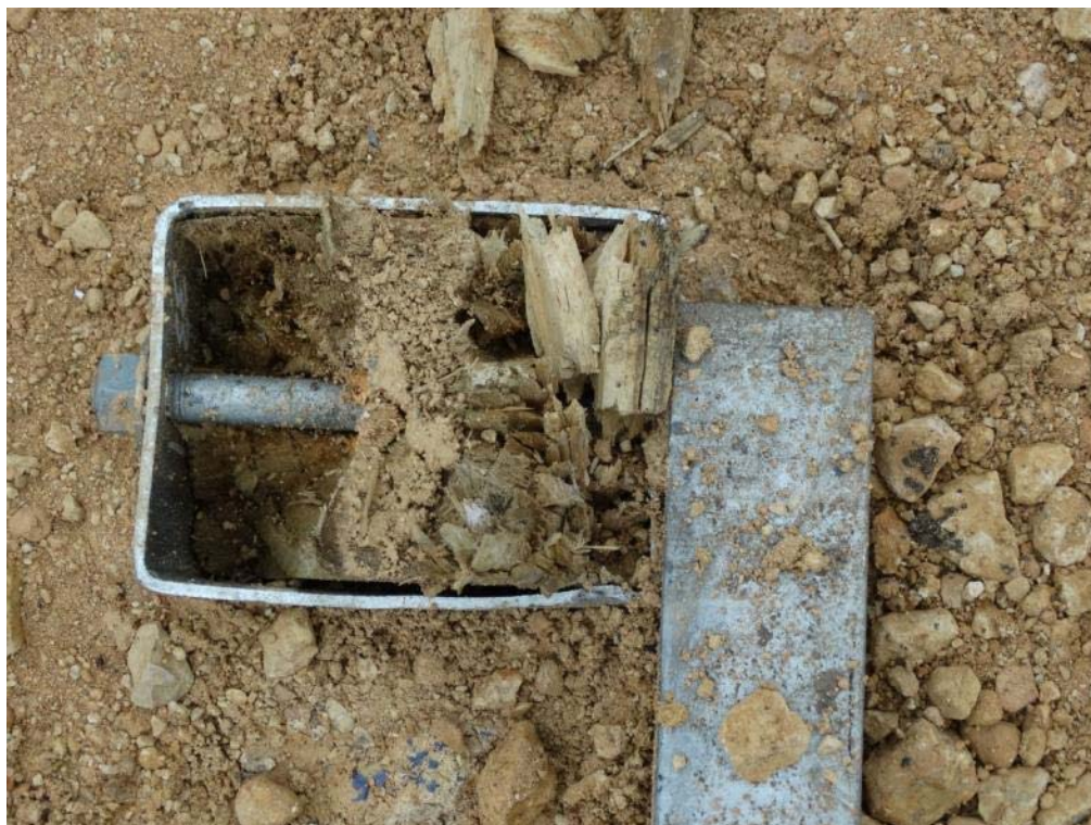
Figure 3.9: Post Test – Foundation Sleeve at Post 2
