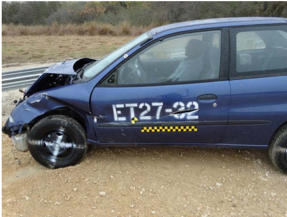
Figure 3.35: Damaged Test Vehicle – Left Side
