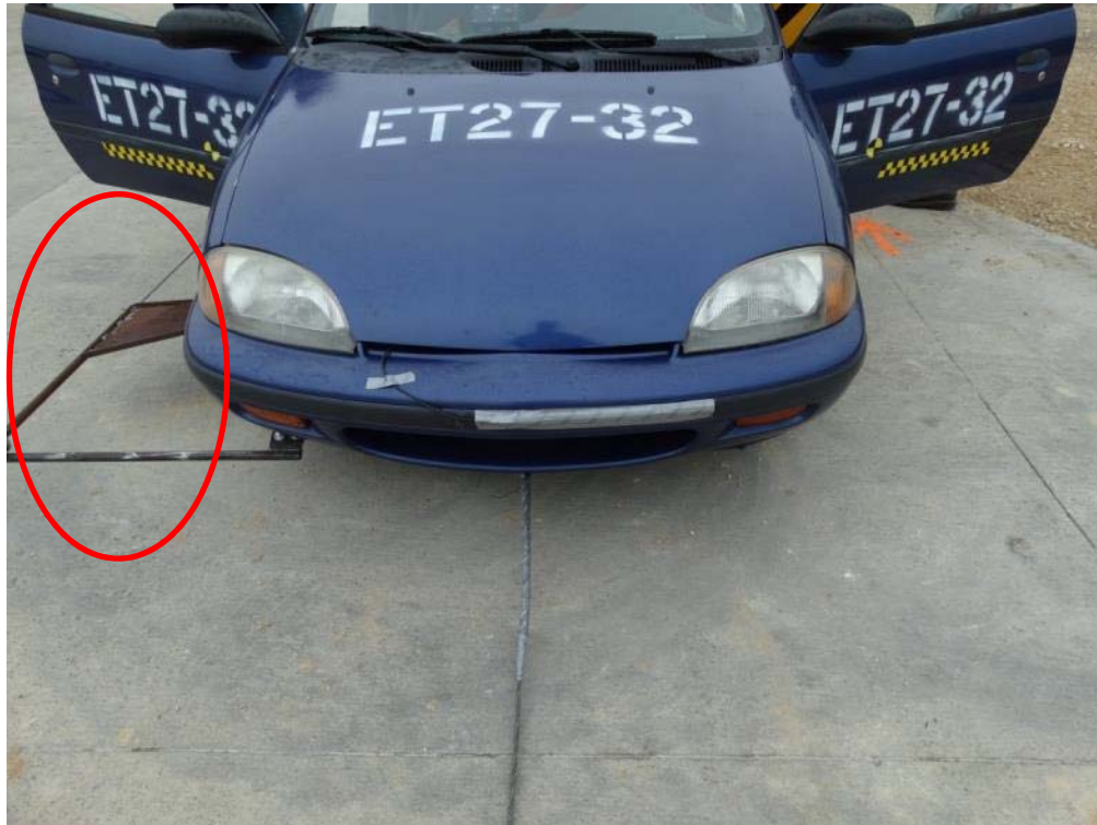
Figure 2.24: Test Vehicle Steering Guidance Assembly
