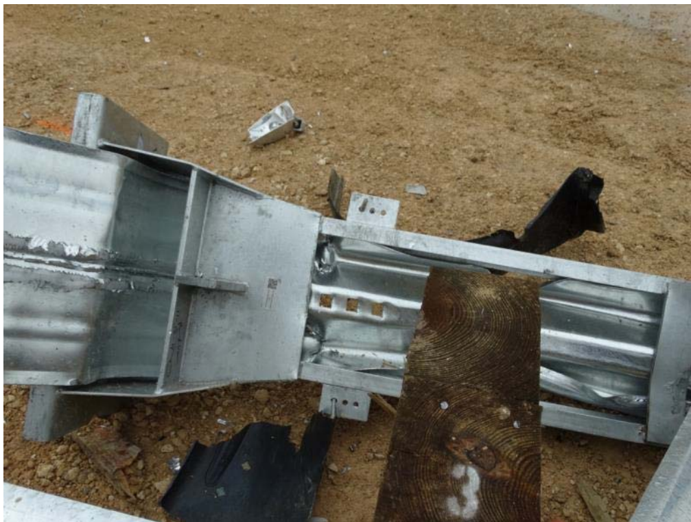
Figure 3.28: Post Test – Non-Traffic Side of Extruder Head
