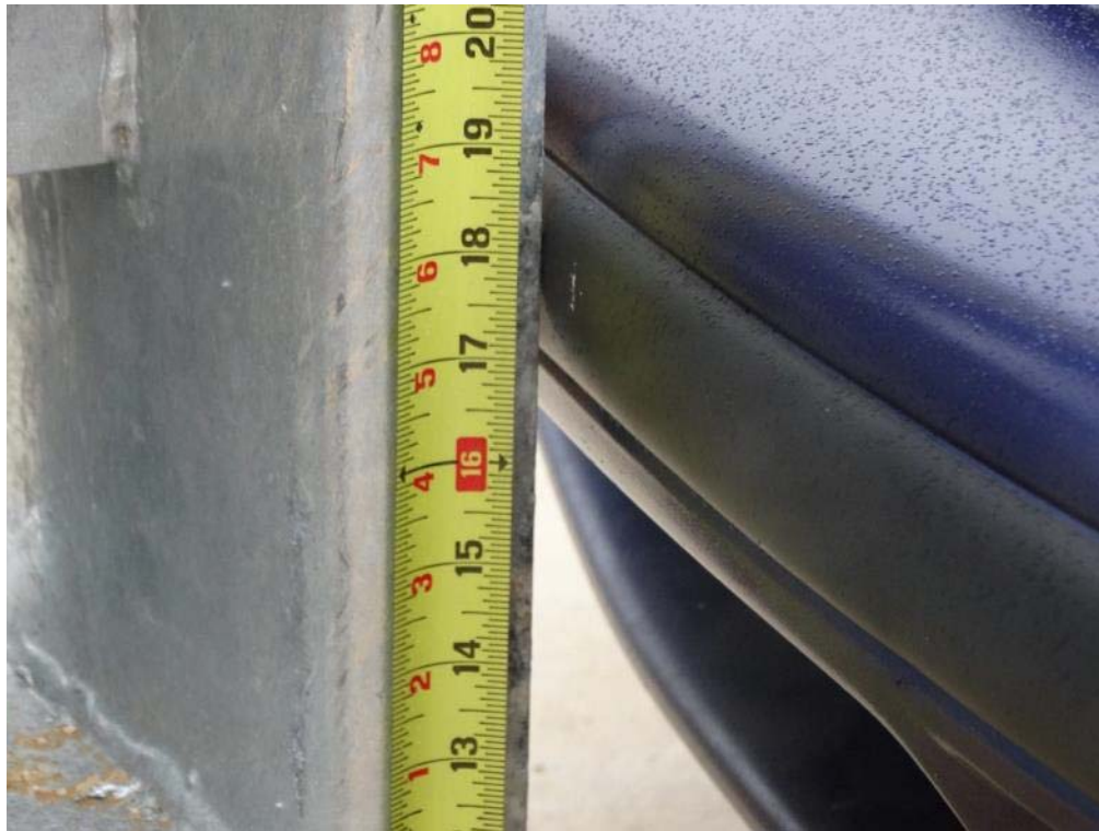
Figure 2.20: Test Vehicle Bumper Height
