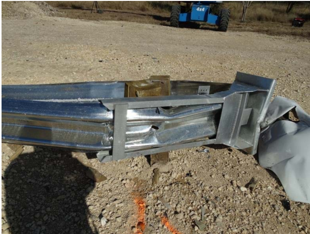
Figure 3.27: Extruder Head Post Test – Traffic Side
