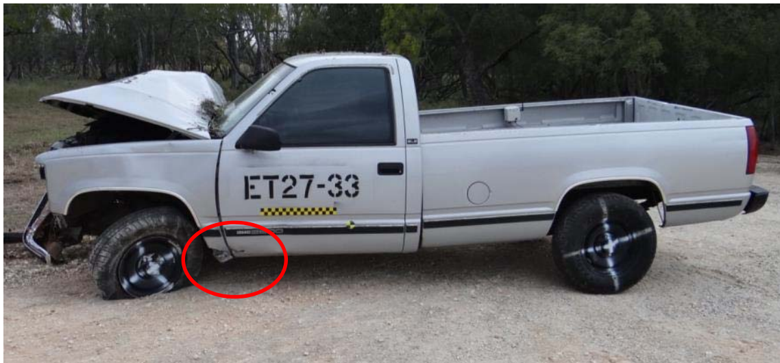
Figure 3.46: Left Side Damage (Note: Hood Damage/Bent Frame Due to Impact with Tree)
