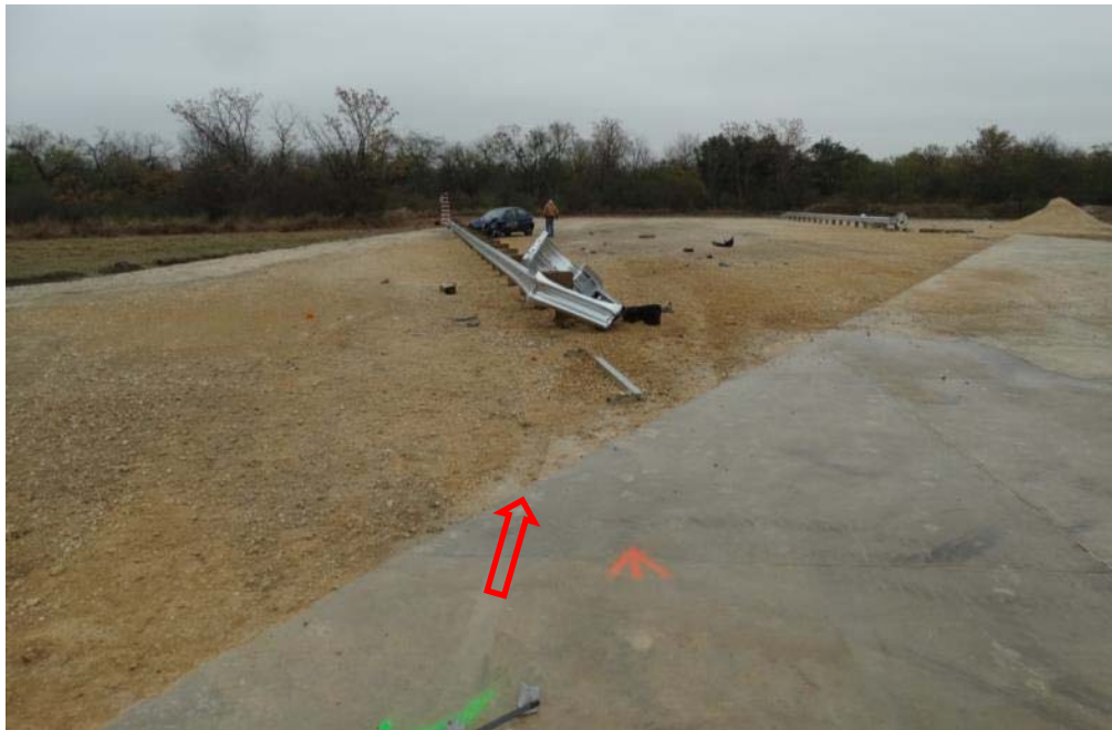
Figure 3.32: Test Vehicle Path of Left Front Tire
