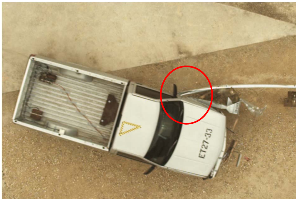
Figure 3.48: Left Side Damage Caused by W beam
