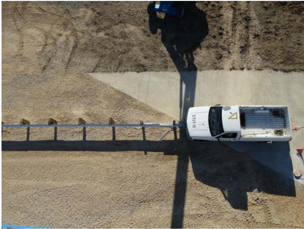
Figure 2.24: Test Vehicle Impact Trajectory – Overhead View
