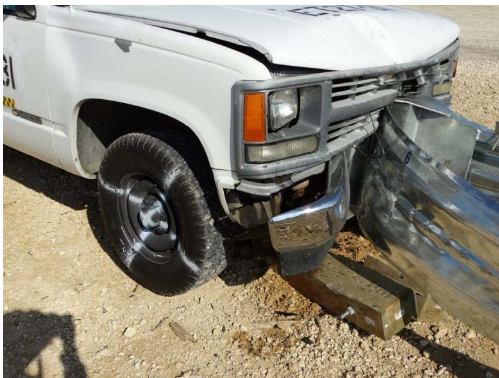
Figure 3.42: Damaged Test Vehicle – Front View Close-up
