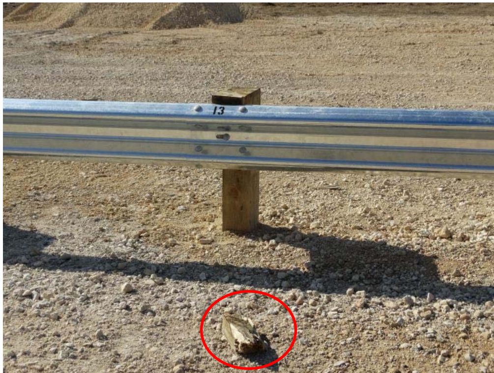
Figure 3.32: Post Test – Line Post 13 and Traffic-Side Debris
