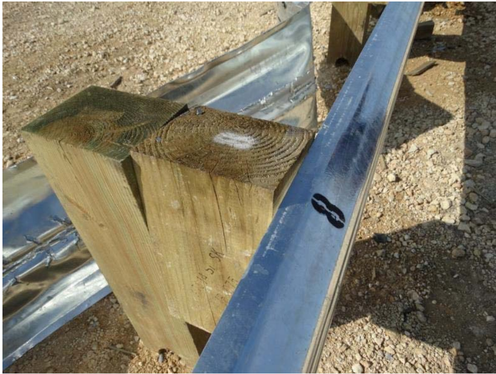
Figure 3.22: Post Test – Post 8 Blockout Twisted
