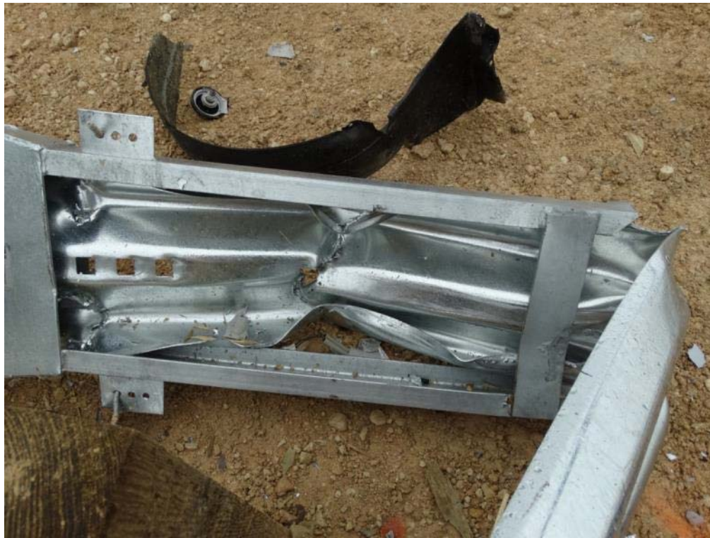
Figure 3.20: Post Test – Non-Traffic Side of Extruder Head
