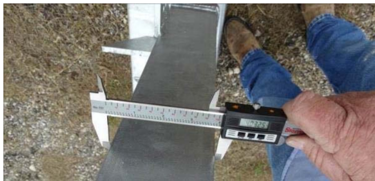
Figure 2.2: Measurement of Channel Width of Head
