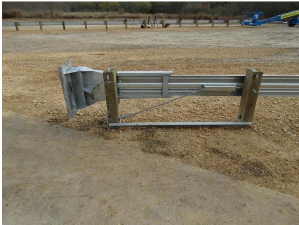
Figure 2.17: End Terminal Head with Posts 1 & 2 and Strut
