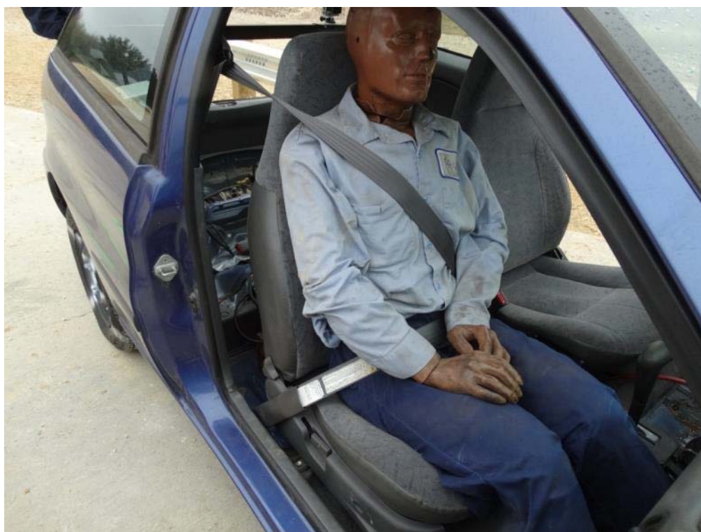
Figure 2.23: Test Dummy Positioned in Passenger Seat
