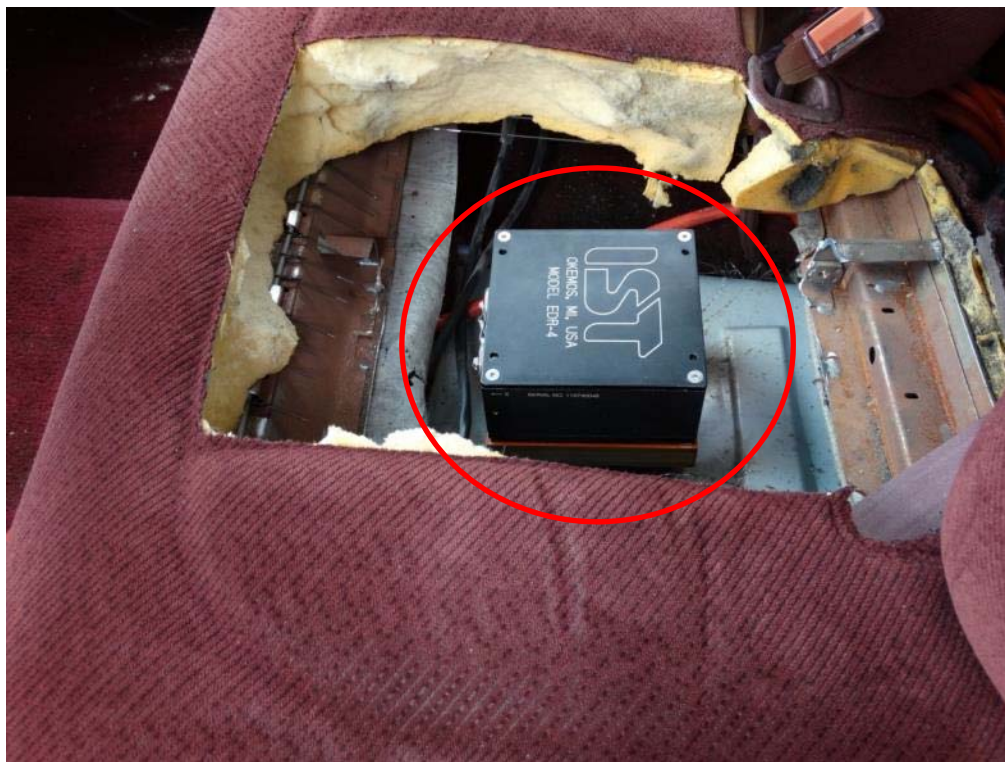
Figure 2.26: EDR Mounted in Test Vehicle for Test ET27-33
