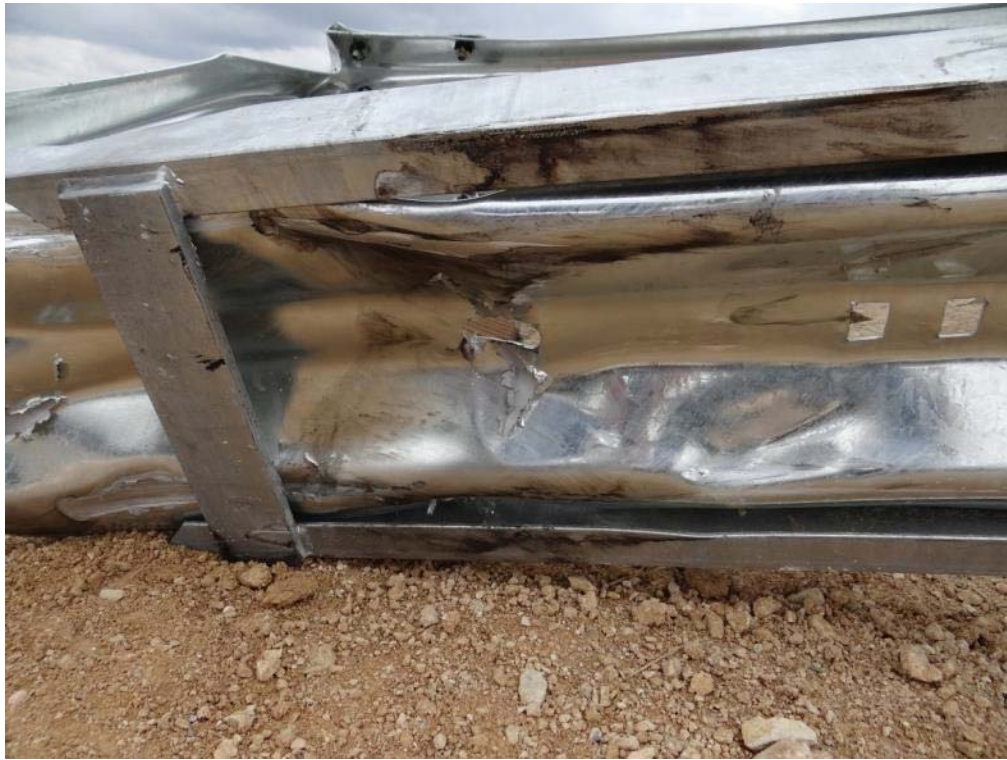
Figure 3.33: Post Test – ET Plus Head Guide Chute Entrance, Traffic Side
