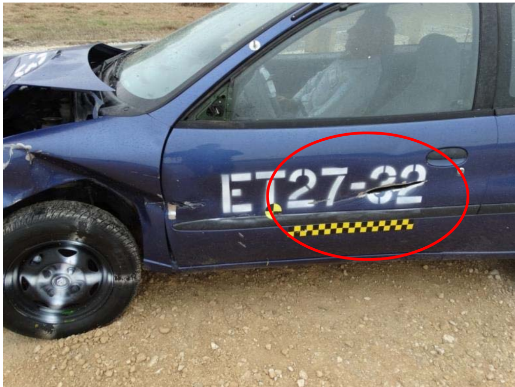
Figure 3.38: Damaged Test Vehicle – Tear in Door Skin
