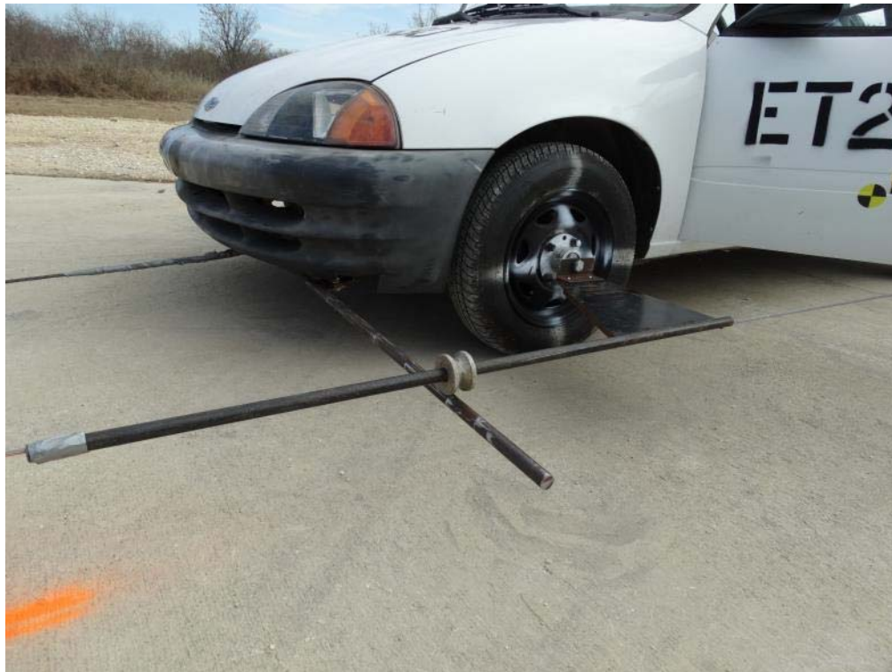
Figure 2.25: Test Vehicle Steering Guidance Assembly
