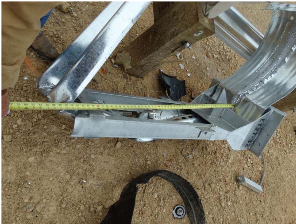
Figure 3.19: Post Test – Gating Between Posts 2 and 3
