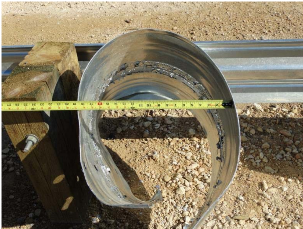
Figure 3.25: Post Test – Extruded Guardrail Coil
