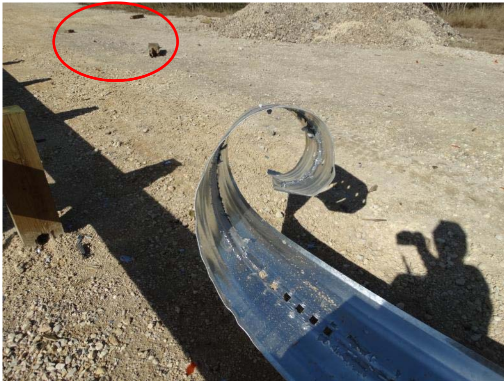
Figure 3.23: Post Test – Extruded Guardrail Coil and Post Debris
