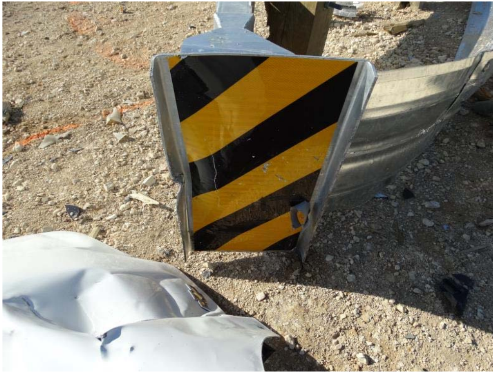
Figure 3.11: Post Test – End View of Extruder Head Impact Plate
