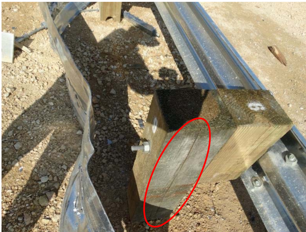
Figure 3.15: Post Test – Post 9 Cracked
