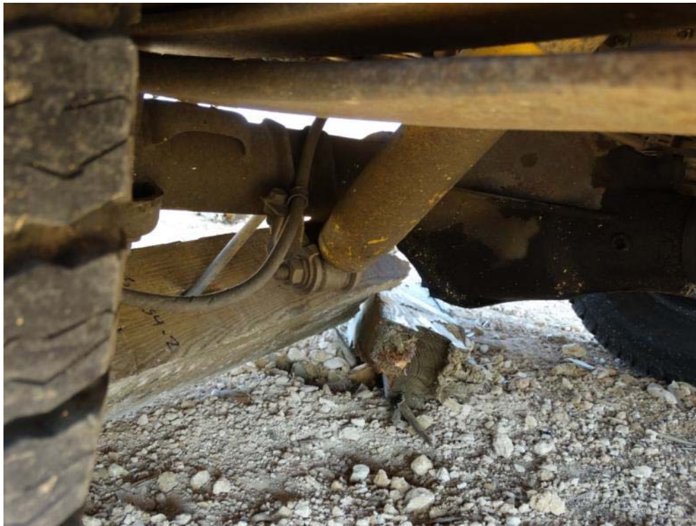
Figure 3.47: Post Test Vehicle – Accumulated Posts Located Under the Vehicle
