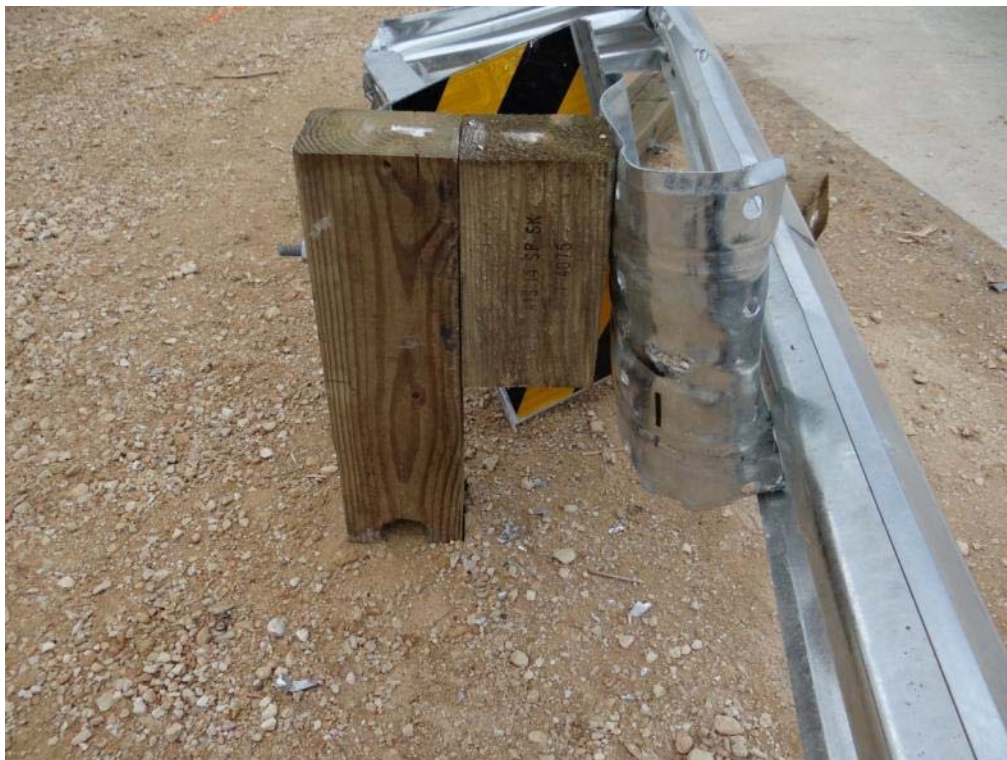
Figure 3.28: Post Test – Extruded Tail of W beam
