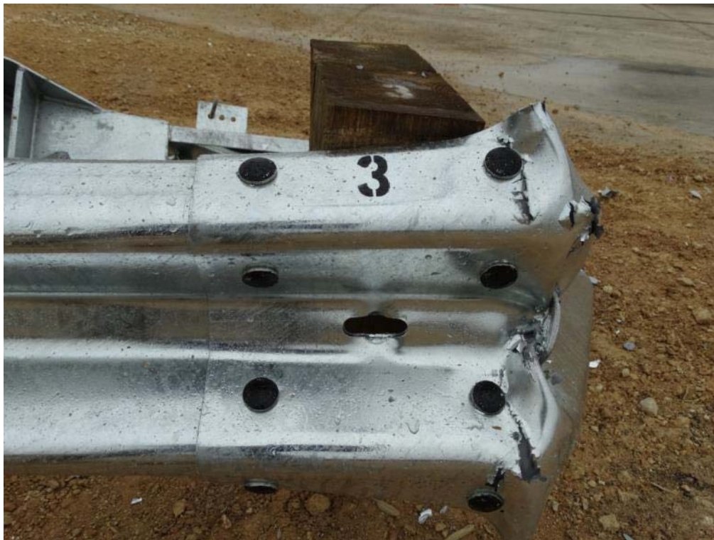
Figure 3.13: Post Test – Gated Guardrail, View from Traffic Side
