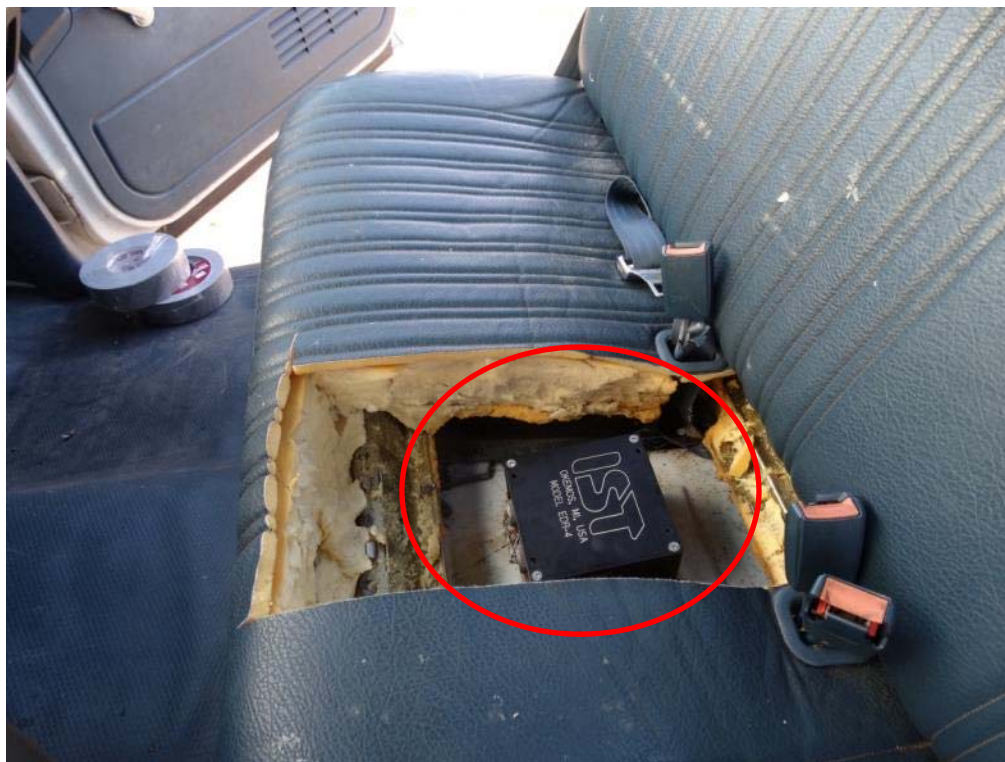
Figure 2.27: EDR Mounted in Test Vehicle for Test ET27-31
