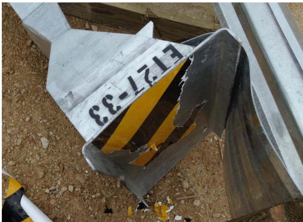
Figure 3.30: Post Test – ET Plus Head Impact Plate
