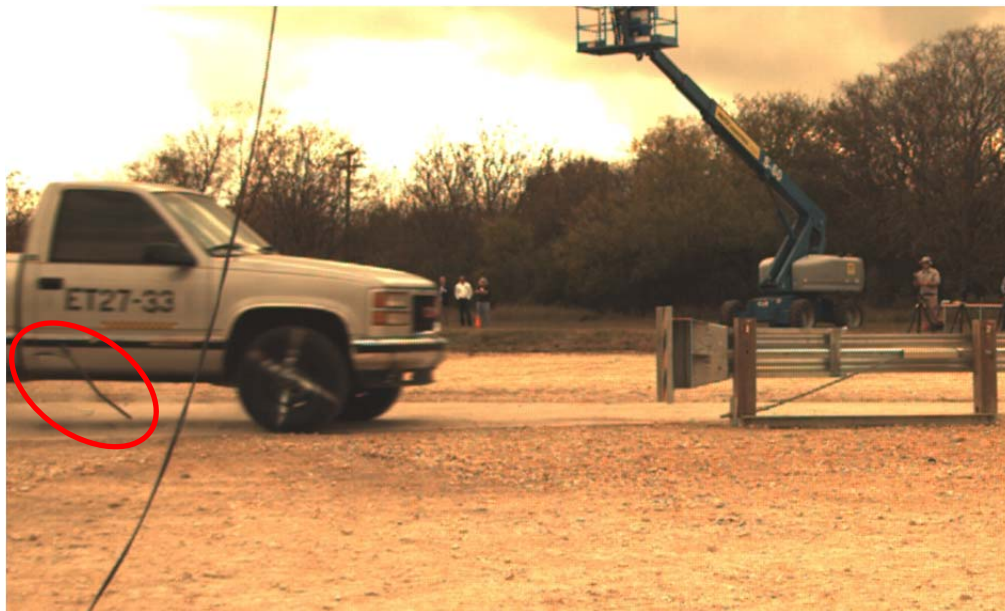
Figure 3.52: Steering Cable Support Rod Creating Damage to Passenger Door Prior to Impact Event
