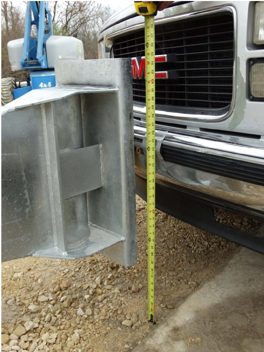
Figure 2.20: Test Vehicle Bumper Height
