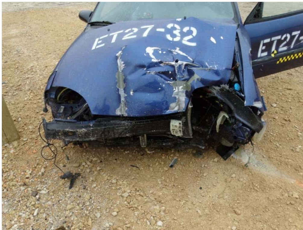
Figure 3.33: Damaged Test Vehicle – Front View
