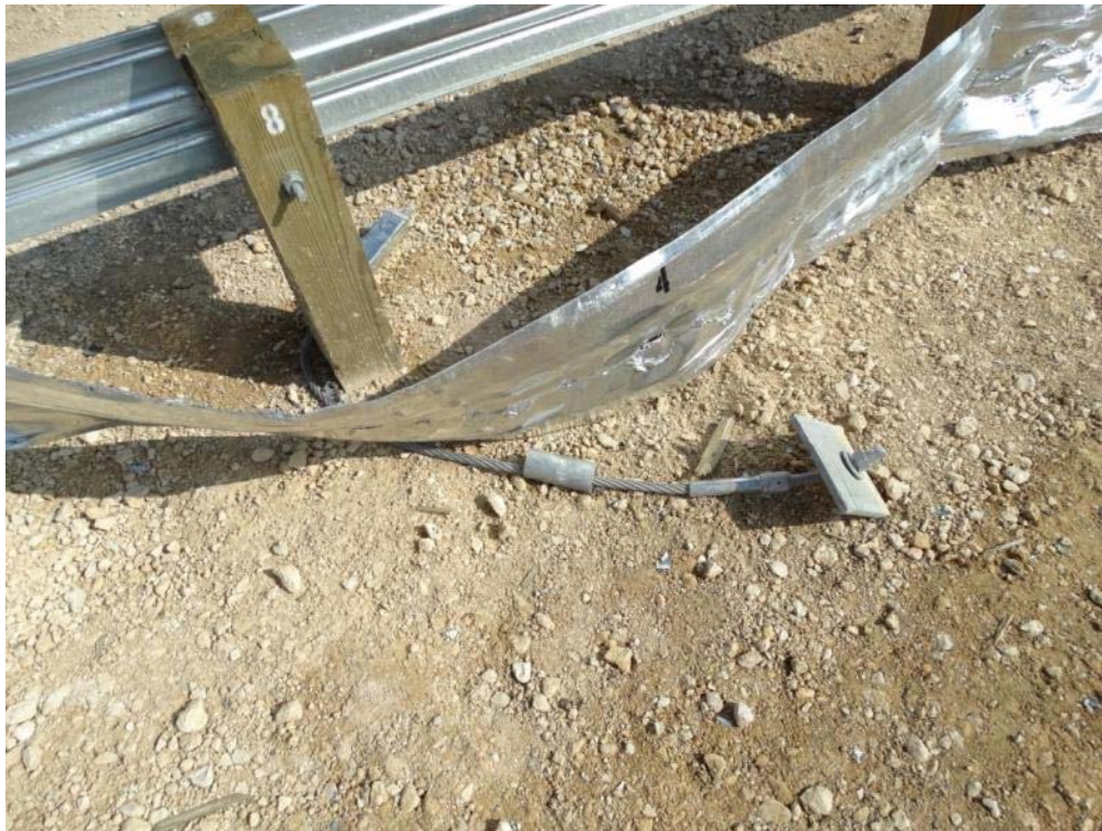
Figure 3.23: Post Test Location of Anchor Cable
