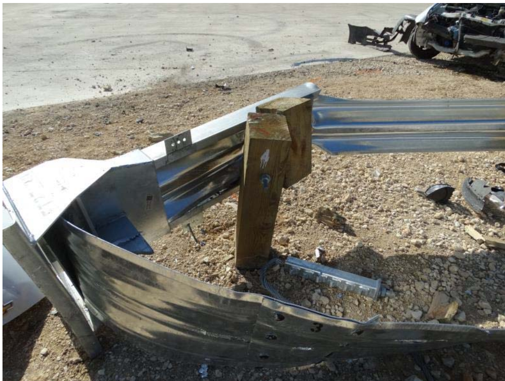
Figure 3.16: Post Test – Non-Traffic Side of Post 4
