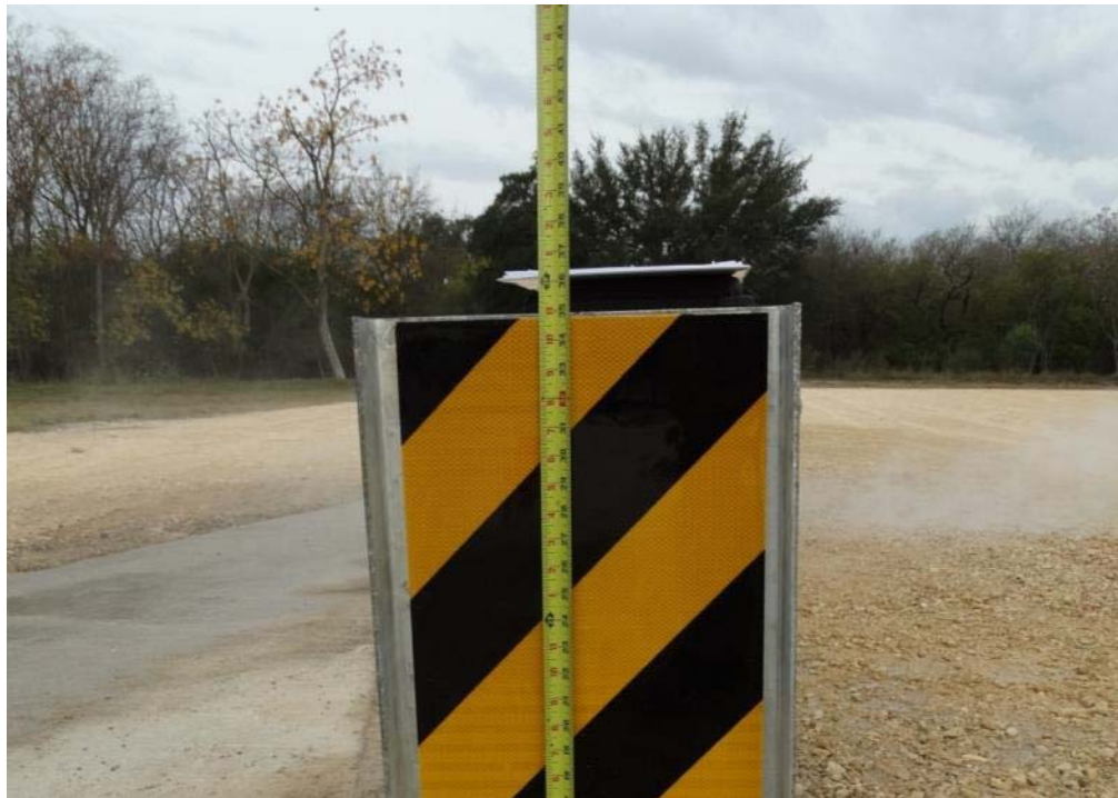
Figure 2.5: ET Plus Head Height Above Ground – Top
