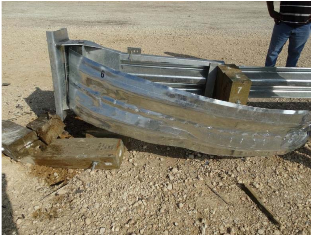
Figure 3.36: Post-Impact Test Article after Vehicle Removed – Non-Traffic Side View
