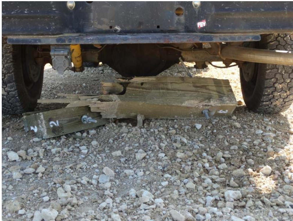
Figure 3.12: Post Test – Posts 2 and 3 Under Vehicle, Close-up
