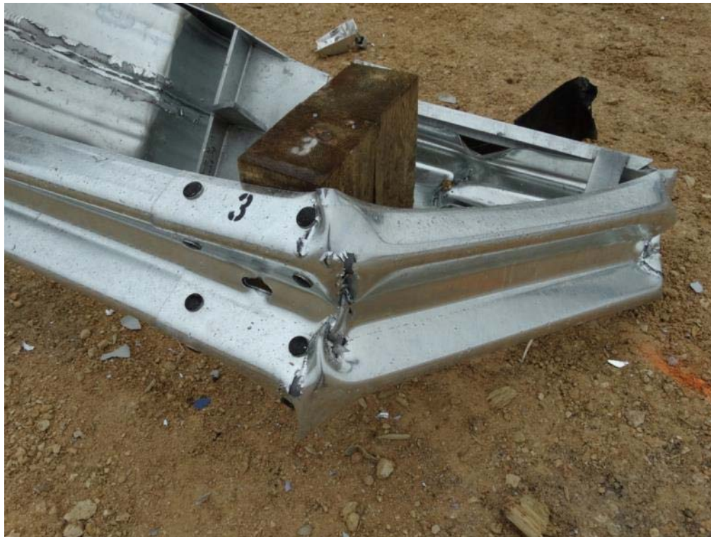
Figure 3.14: Post Test – Gated Guardrail
