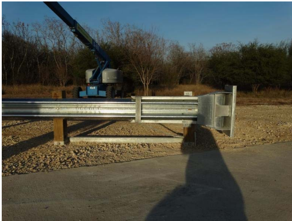
Figure 2.15: End Terminal Head with Posts 1 & 2 and Strut
