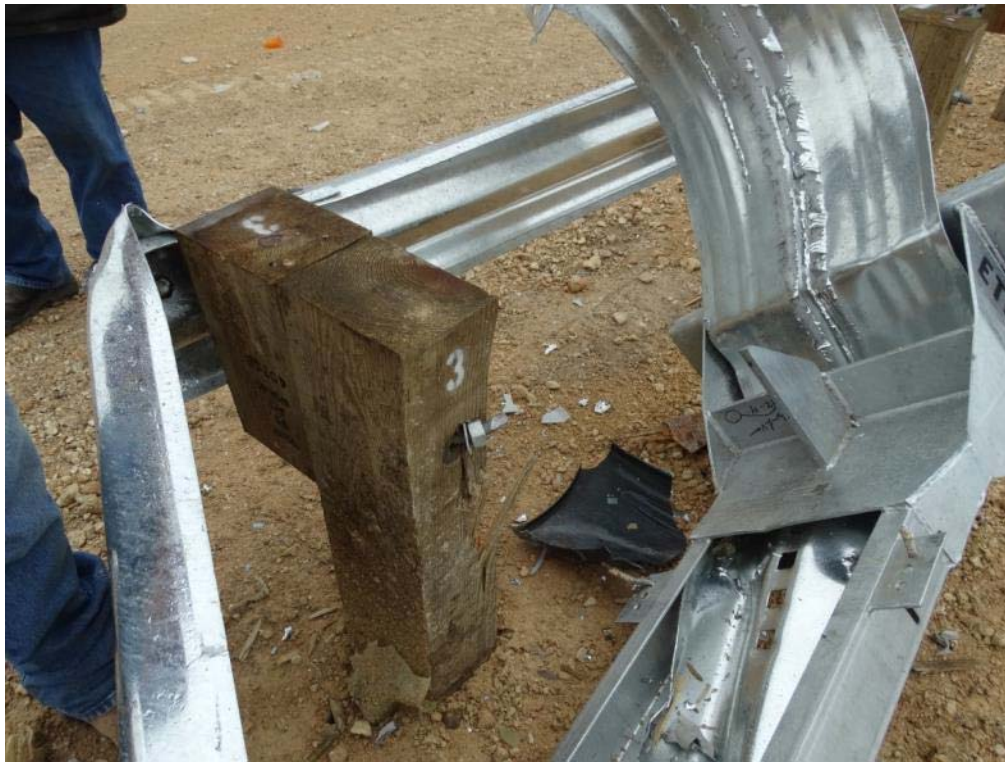
Figure 3.18: Post Test – Extruded Guardrail
