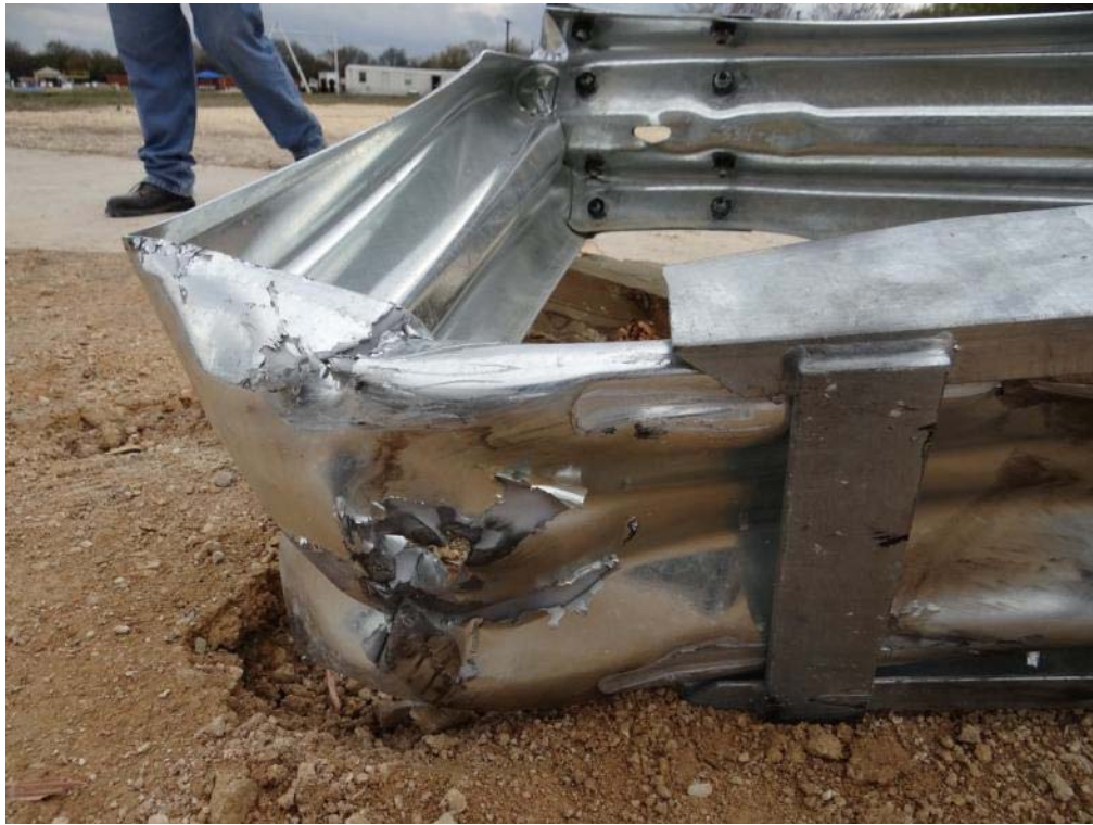
Figure 3.27: Post Test – Side View of Guide Chute Entrance
