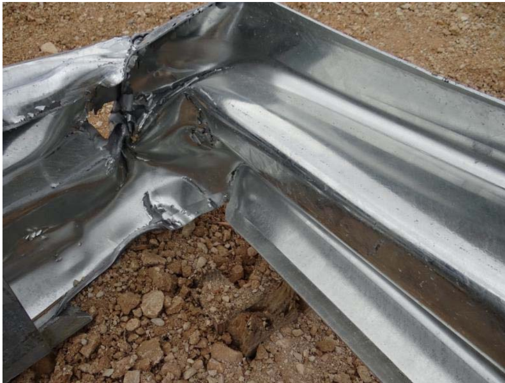
Figure 3.25: Post Test – Gating Past Extruder Head
