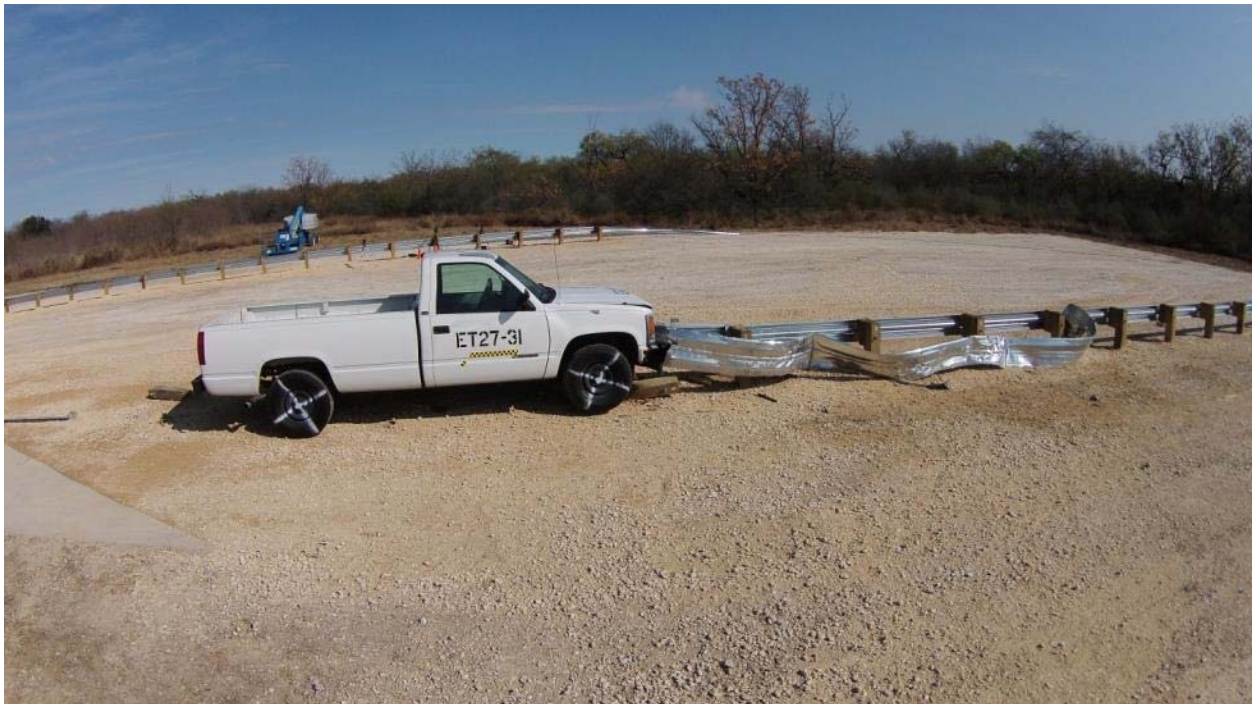
Figure 3.7: Post-Impact Condition of the Test Article and Vehicle
