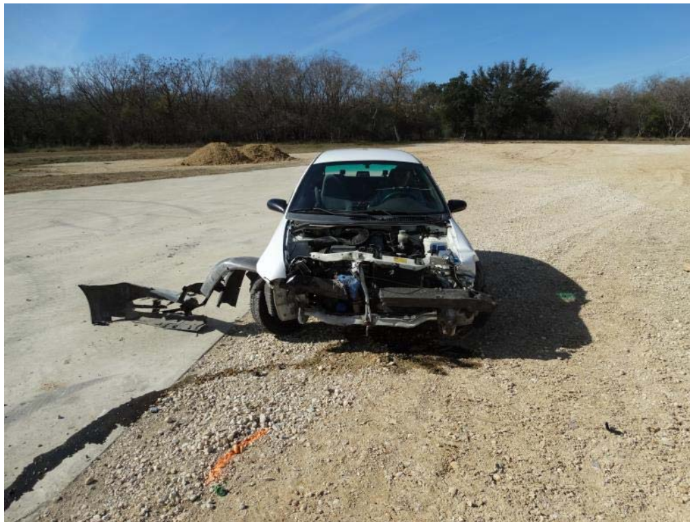
Figure 3.31: Damaged Test Vehicle – Front View
