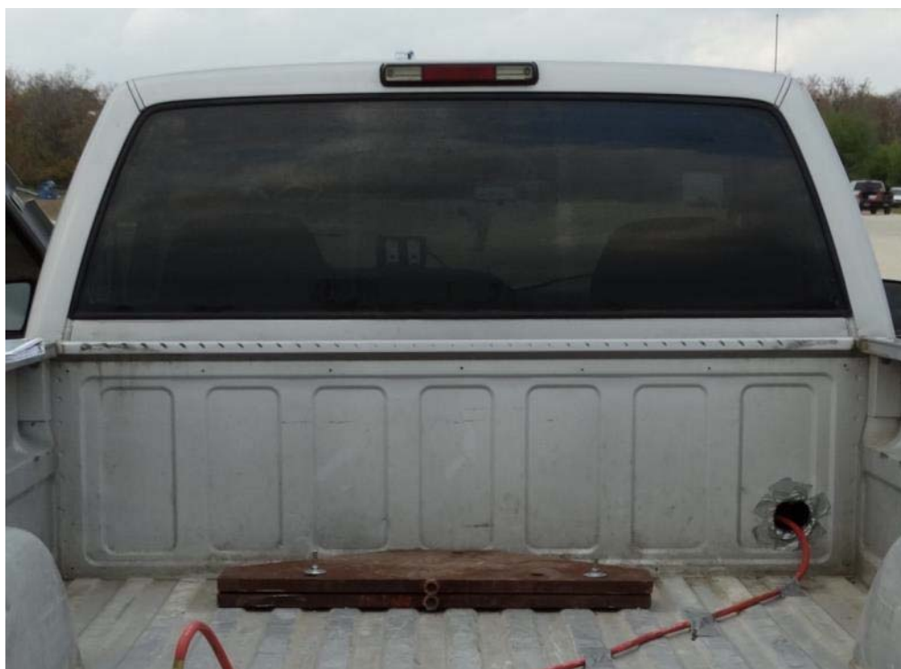
Figure 2.24: Test Vehicle Ballast
