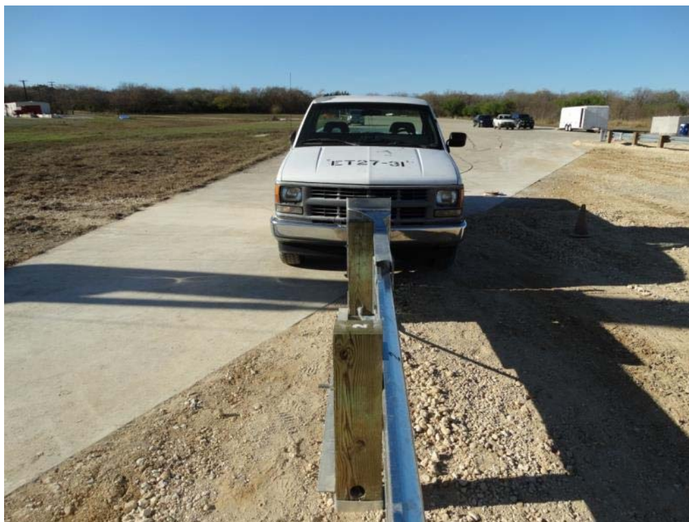
Figure 2.23: Test Vehicle Impact Trajectory
