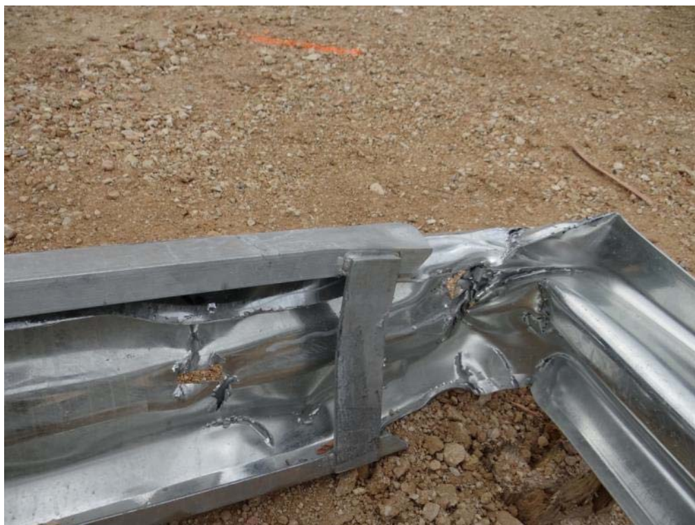
Figure 3.36: Post Test – ET Plus Head Guide Chute Entrance, Non-Traffic Side
