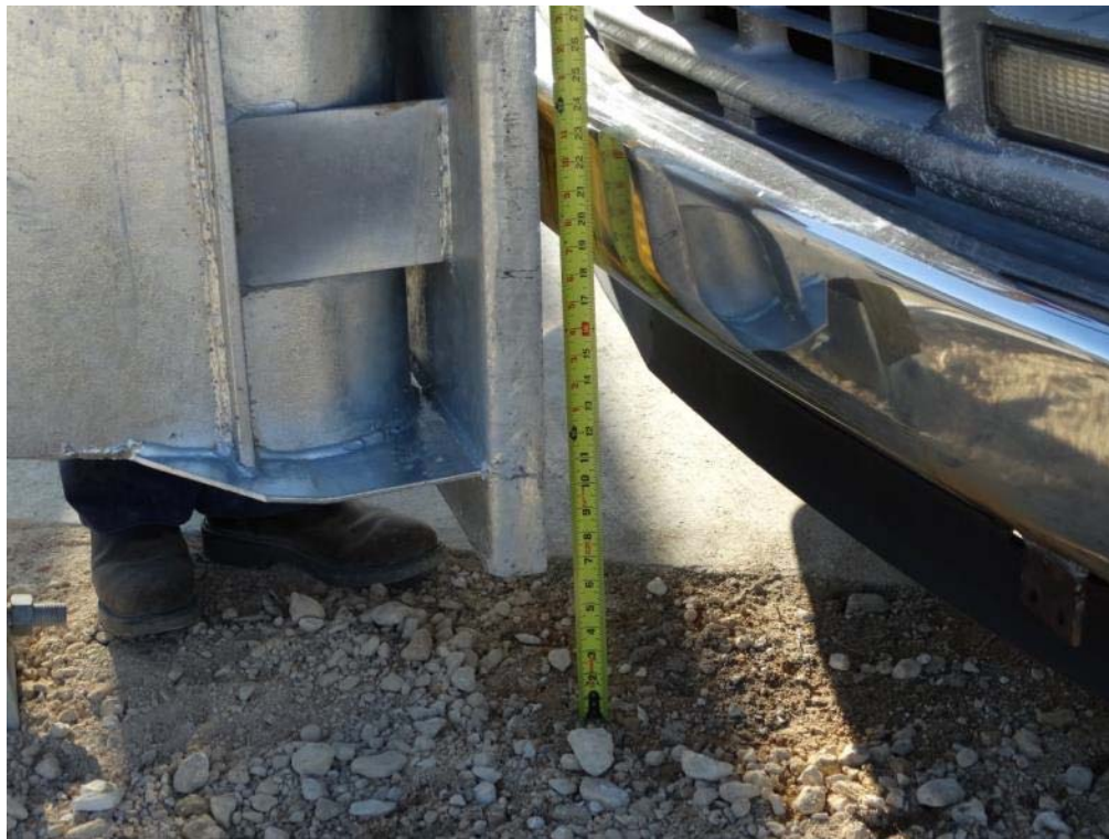
Figure 2.22: Test Vehicle Bumper Height
