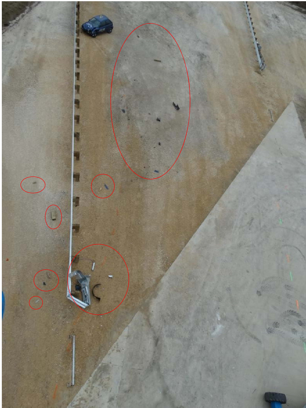
Figure 3.29: Post-Impact Debris Field
