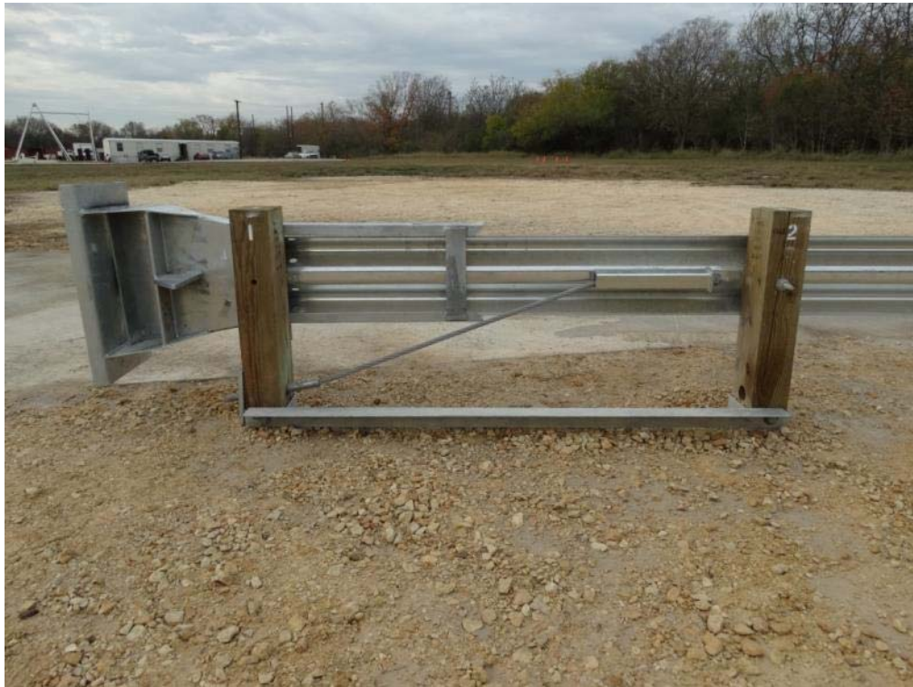
Figure 2.15: End Terminal Head with Posts 1 & 2 and Strut
