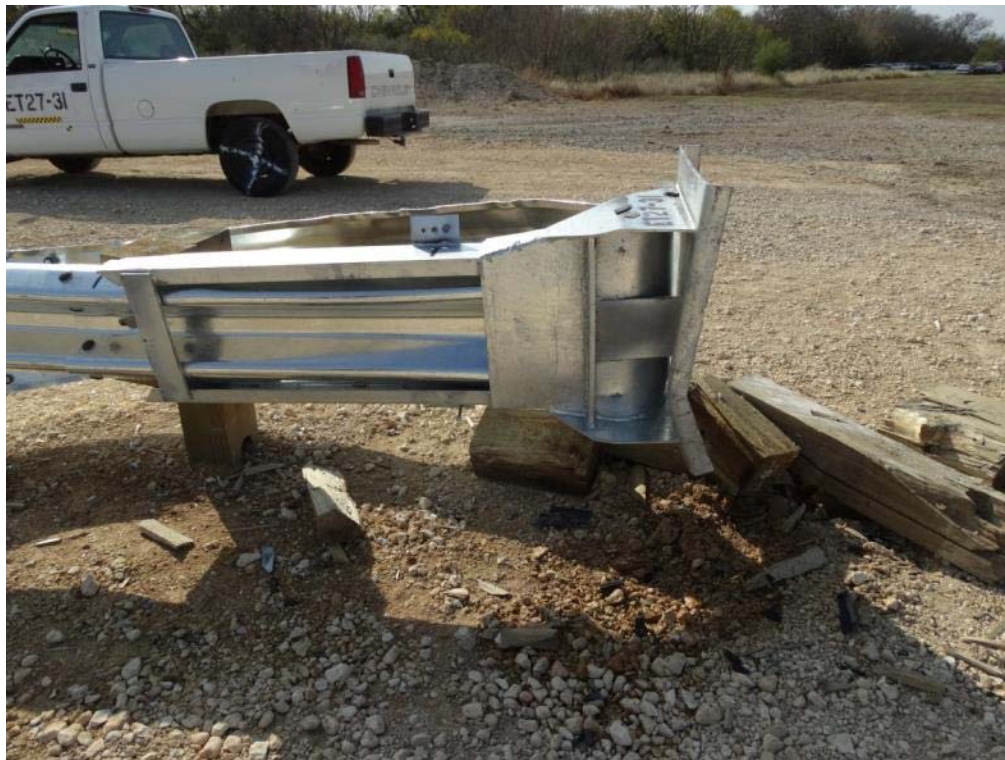
Figure 3.34: Post-Impact Test Article after Vehicle Removed – Traffic Side View
