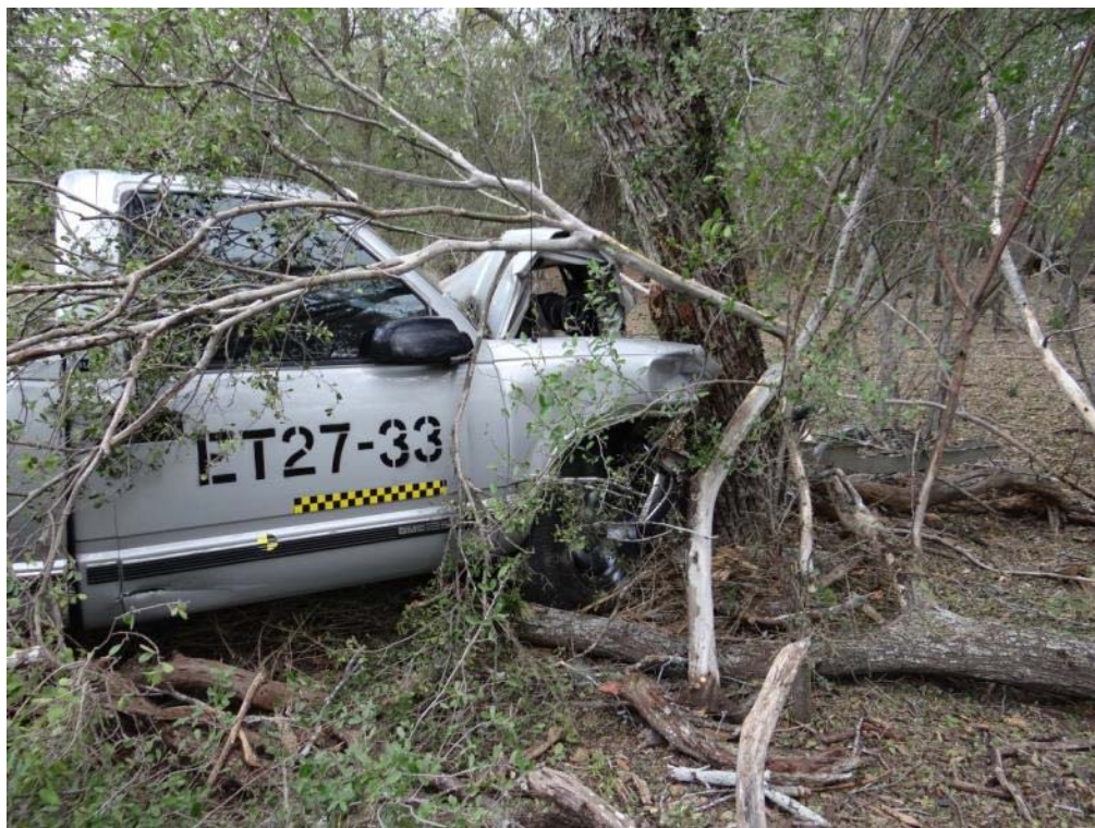
Figure 3.43: Test Vehicle Impacted Tree
