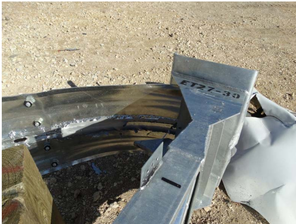
Figure 3.17: Post Test – Extruded Guardrail at Extruder Head
