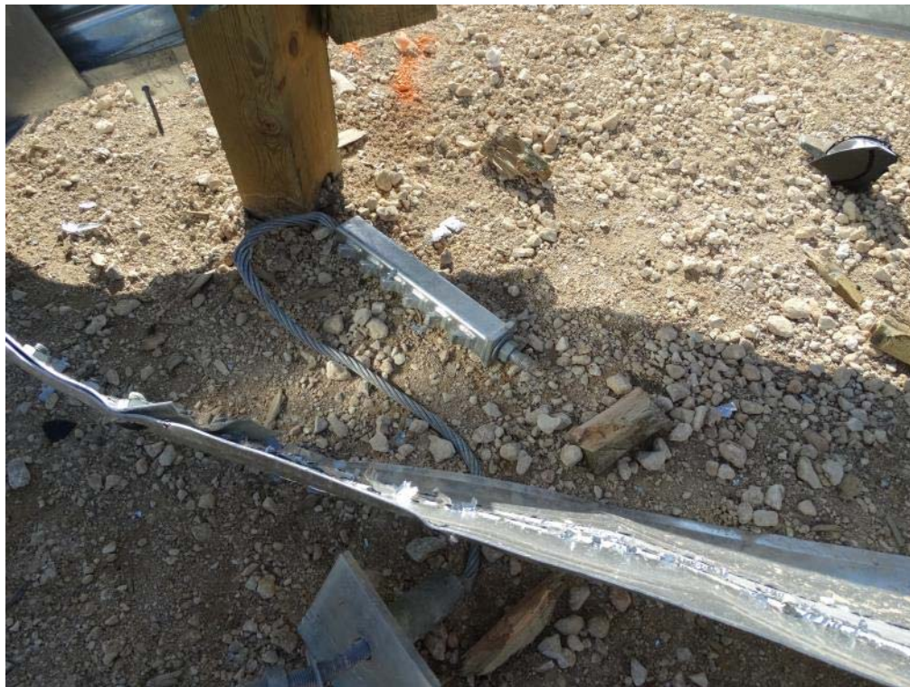
Figure 3.25: Post Test Location of Anchor Cable
