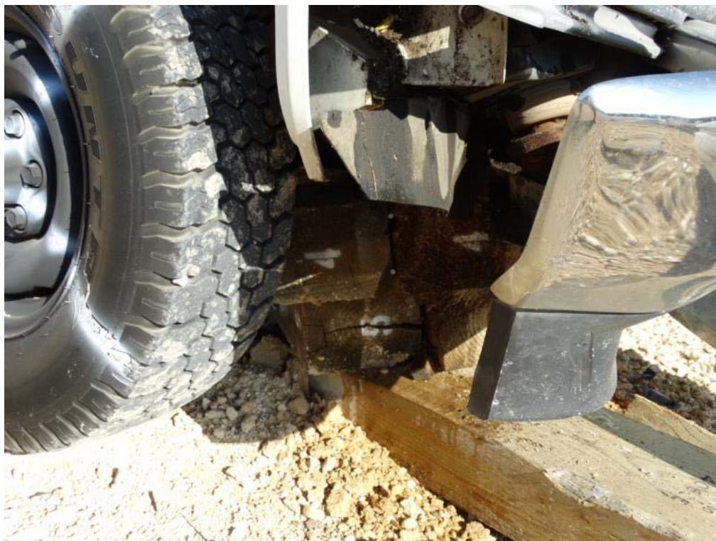
Figure 3.13: Post Test – Posts 4, 5 and 6 Stacked Under Vehicle
