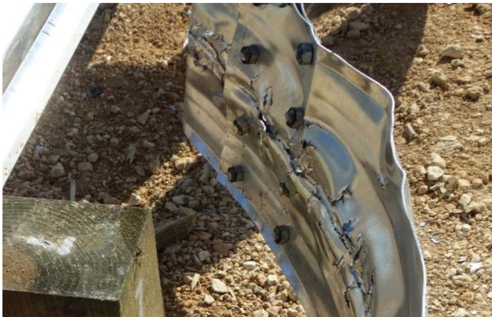
Figure 3.29: Post Test – Extruded Guardrail Splice from Post 5, Splice Nuts
