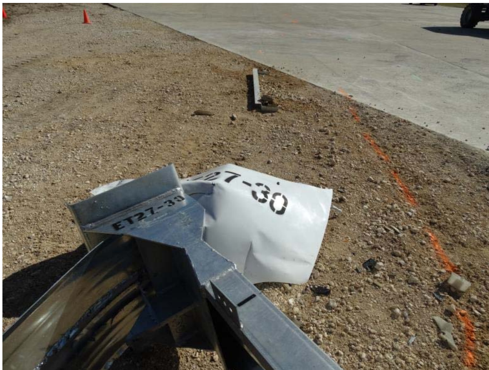
Figure 3.12: Post Test – Upstream View of Extruder Head
