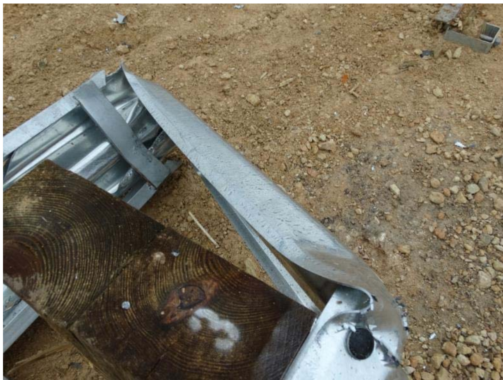
Figure 3.15: Post Test – Gated Guardrail
