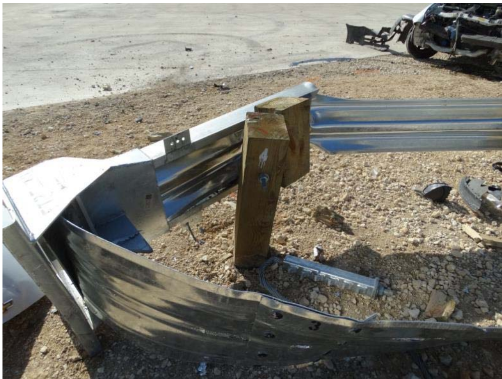
Figure 3.28: Extruder Head Post Test – Non-Traffic Side
