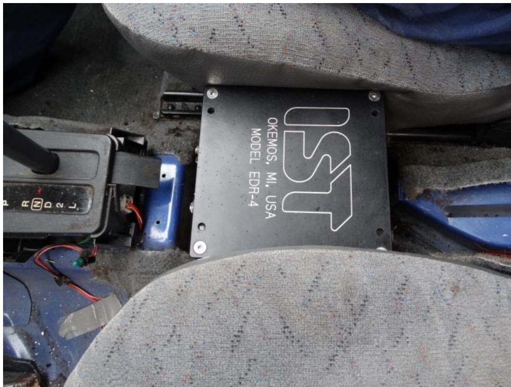
Figure 2.25: EDR Mounted in Test Vehicle for Test ET27-32
