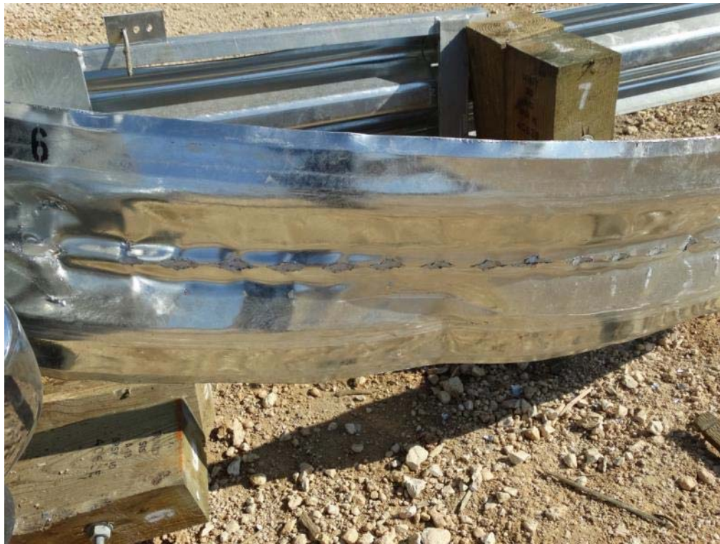
Figure 3.18: Post Test – Extruder Head at Post 7, Blockout Twisted
