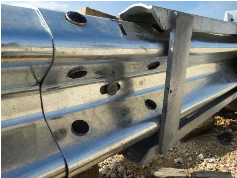
Figure 3.37: Post-Impact Test Article after Vehicle Removed –Guide Channel Entrance
