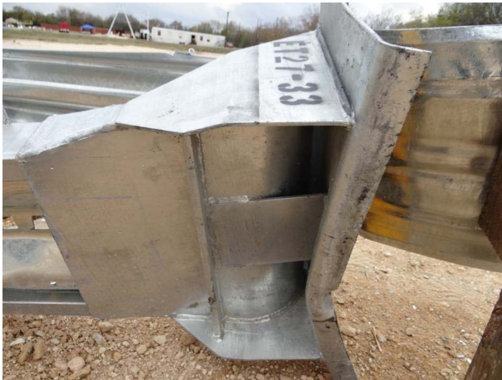
Figure 3.31: Post Test – ET Plus Head, Traffic Side
