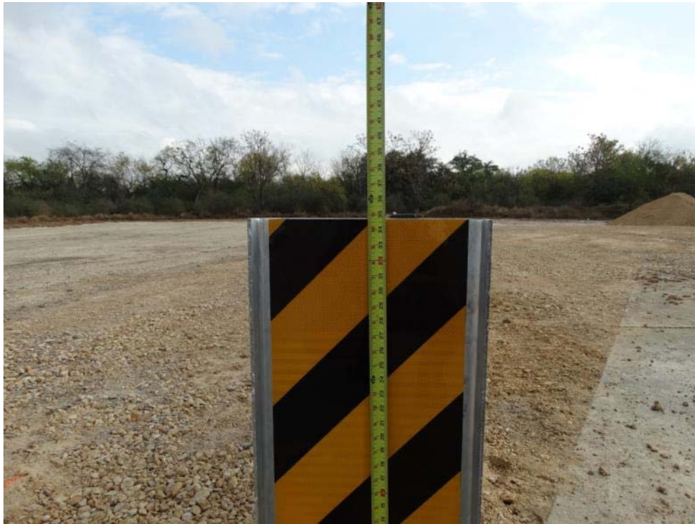
Figure 2.5: ET Plus Head Height Above Ground – Top
