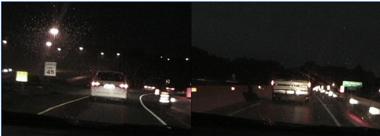
Figure 17. Photos. The AWP (left) and standard pavement marking (right) work zones on eastbound US-32/33/50 at night.
