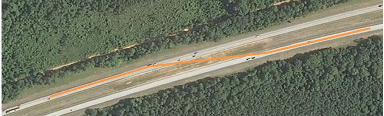
Figure 9. Photo. Aerial view of southern crossover. Southbound traffic shifts back to normal operation.
