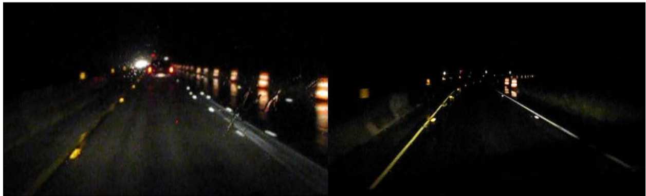
Figure 3. Photos. Wet weather comparison of standard pavement marking (left) and the AWP (right) pavement markings.
