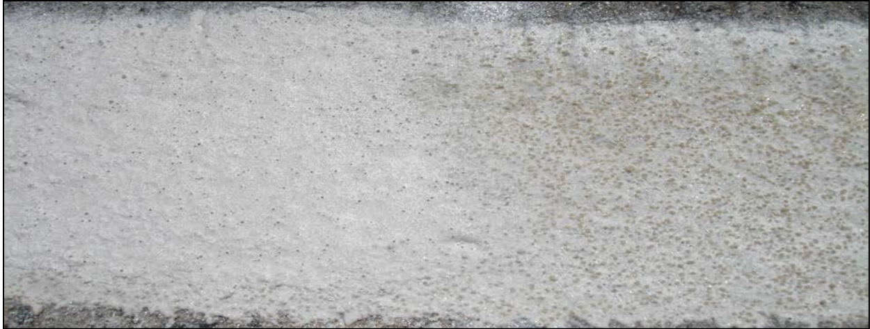
Figure 4. Photos. Comparison between standard pavement marking (left) and the AWP marking with microcrystalline ceramic beads (right).
