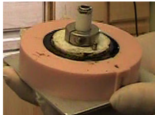
Step 11.2. Rotation completed. Post lines up with label "L" on mold.
