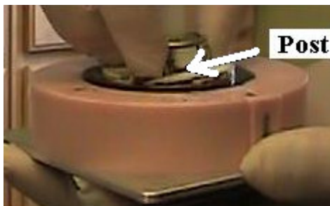
Step 11.2. Post is pushed back by index finger of right hand.
