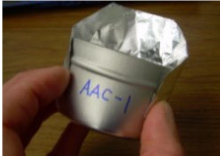
Steps 4.1 and 4.2. Line up foil on container seal.
