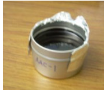
Step 4.3. Mold foil onto container for good seal.
