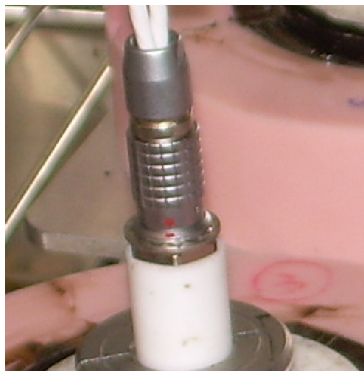
Step 12.2. Line up red dots on ring and wire harness.
