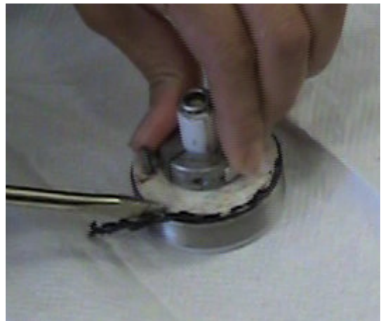
Step 15.5.1. Cleaning ring with paper towel. Step 15.5.2. Screwdriver to carefully remove binder from ABCD ring.
