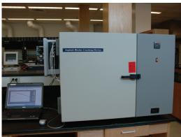
The ABCD system includes a computer to collect data and control the environmental chamber, which cools the asphalt binder samples at a controlled rate.
