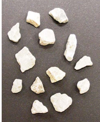
Figure 2.11. Light 4.75 mm (ASTM #4 sieve) aggregates used in Experiment 5.
