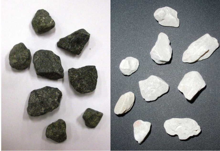
Figure 2.4. Dark and light 9.5 mm (0.375 in) aggregates used in Experiment 5.
