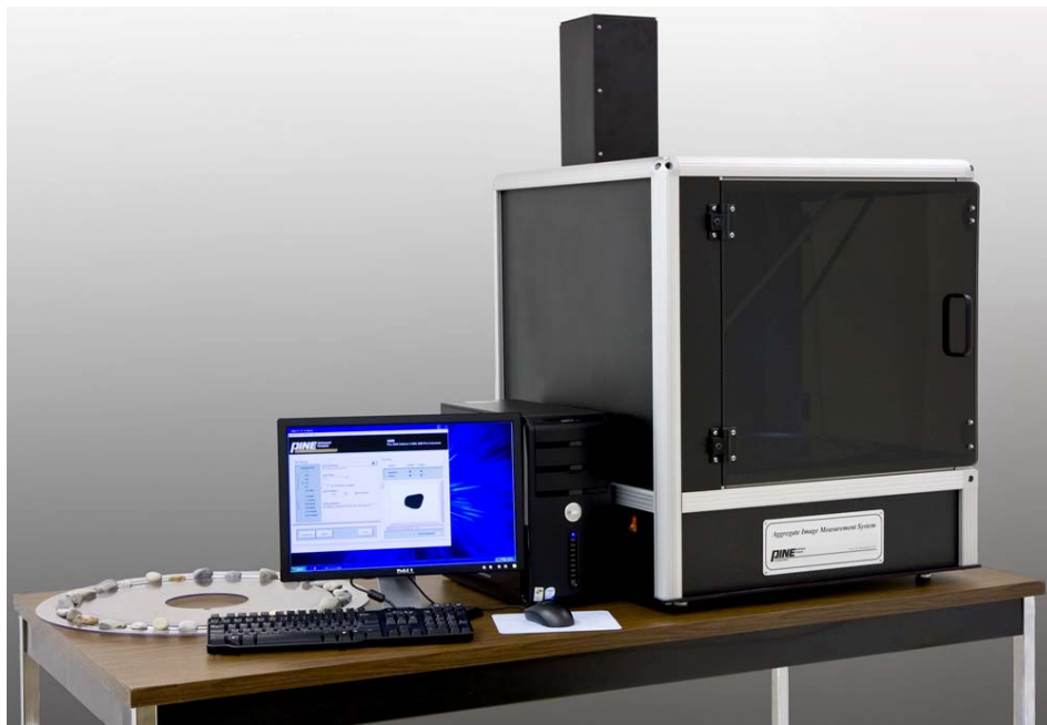
Figure 2. Photo. New Aggregate Imaging Measurement System equipment (AIMS2) (photo courtesy of Pine Instrument).
