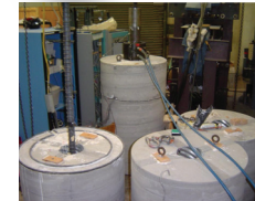
Large-Bar Pullout Tests
