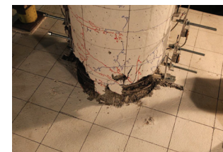
Spread Footing Specimen After Testing
