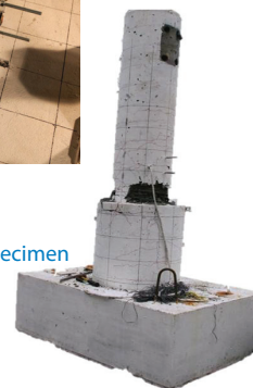
Spread Footing Specimen After Testing
