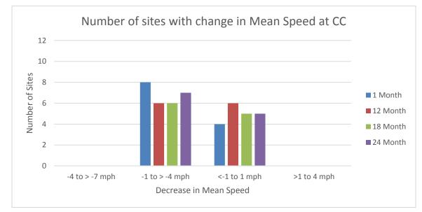
Figure 20. Graph. Number of sites with a change in mean speed for all vehicles of a certain magnitude at the center of curve (CC).
