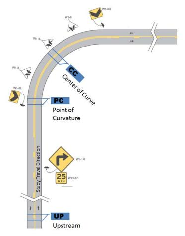
Figure 15. Diagram. Typical traffic counter placement.
