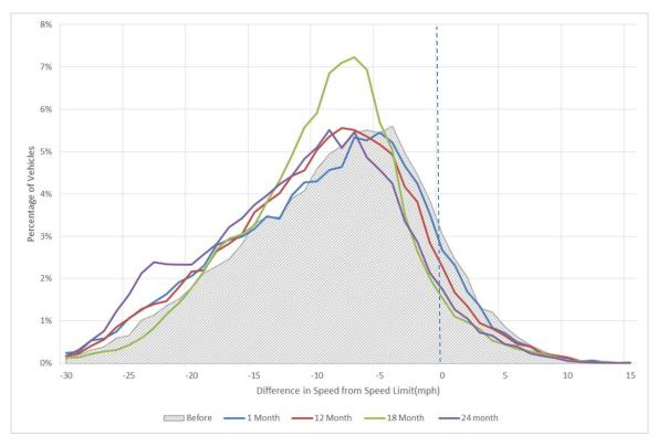
Figure EX.6. Percentage of vehicles with difference in speed from speed limit at center of curve (CC).
