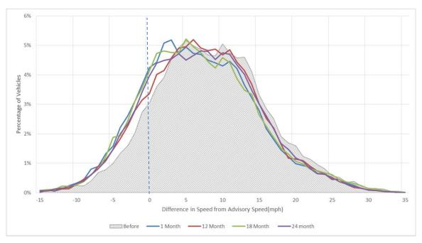
Figure 30. Graph. Percentage of vehicles with difference in speed from advisory speed at point of curvature (PC).
