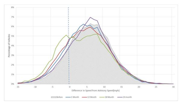
Figure 32. Graph. Percentage of vehicles with difference in speed from advisory speed at center of curve (CC).
