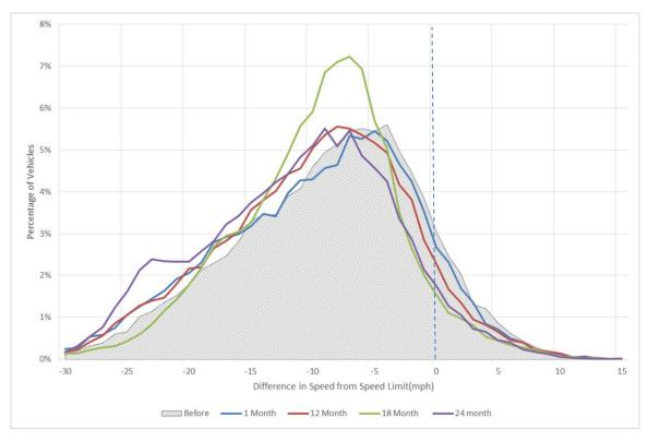
Figure 31. Graph. Percentage of vehicles with difference in speed from speed limit at center of curve (CC).
