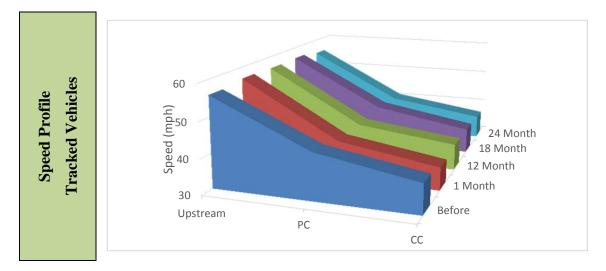
Figure 96. Graph. Speed profiles of tracked vehicles – Wisconsin Hwy 20.
