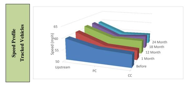
Figure 106. Graph. Speed profiles of tracked vehicles – Wisconsin Hwy 213.
