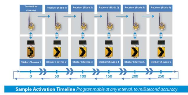
Figure 14. Photo. Example SDCWS activation sequence. (Source: TAPCO)
