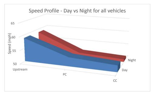
Figure 136. Graph. Day vs Night speed profile comparison for all vehicles – Wisconsin Hwy 213.
