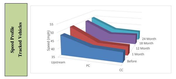
Figure 86. Graph. Speed profiles of tracked vehicles – Washington SR 9.
