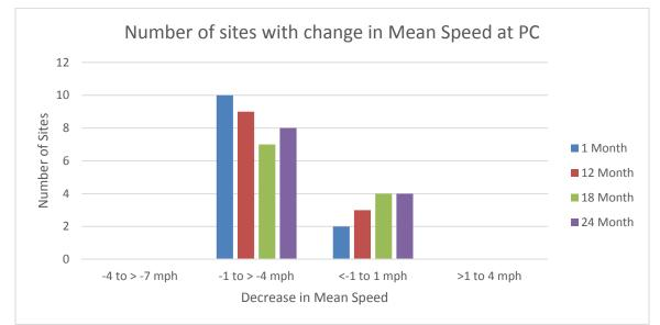
Figure 16. Graph. Number of sites with a change in mean speed for all vehicles of a certain magnitude at the point of curvature (PC).
