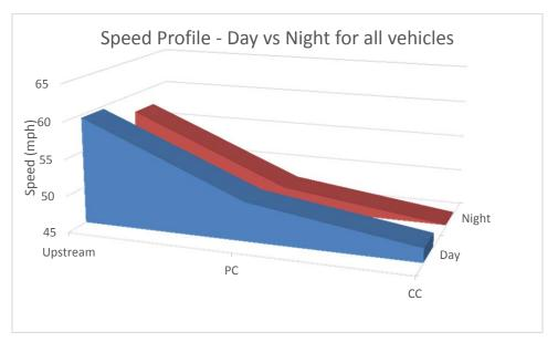
Figure 129. Graph. Day vs Night speed profile comparison for all vehicles – Iowa Hwy 144.
