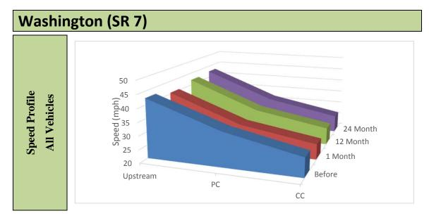
Figure 80. Graph . Speed profiles of all vehicles – Washington SR 7.
