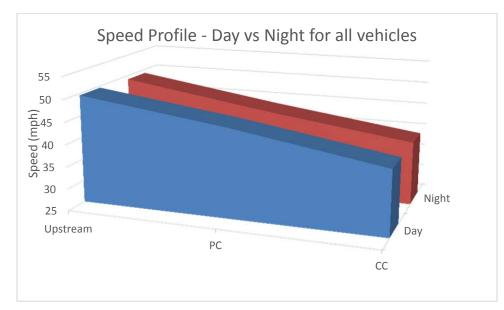
Figure 135. Graph. Day vs Night speed profile comparison for all vehicles – Wisconsin Hwy 67.
