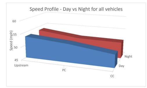
Figure 133. Graph. Day vs Night speed profile comparison for all vehicles – Washington SR 203.
