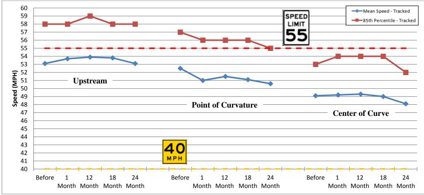
Figure 74. Graph. Impact on tracked vehicle speed - Missouri Hwy 221.
