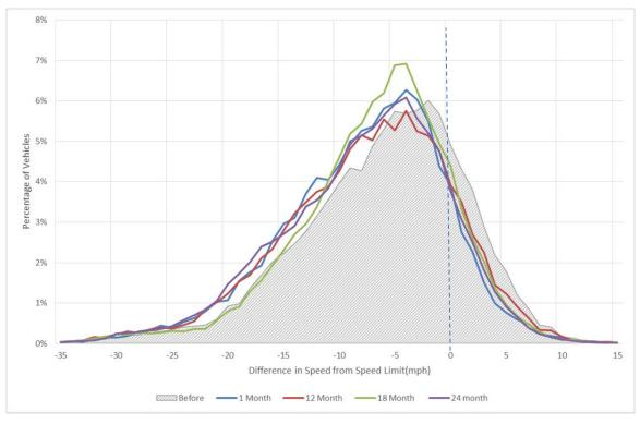
Figure EX.4. Percentage of vehicles with difference in speed from speed limit at point of curvature (PC).
