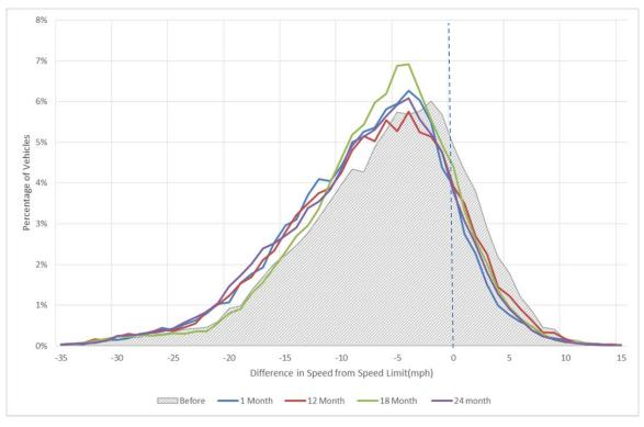
Figure 29. Graph. Percentage of vehicles with difference in speed from speed limit at point of curvature (PC).
