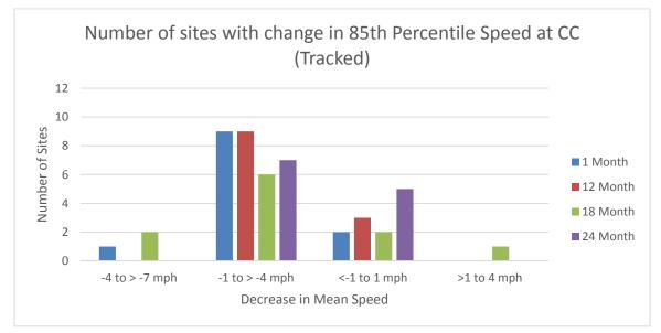
Figure 23. Graph. Number of sites with a change in 85<sup>th</sup> percentile speed for tracked vehicles of a certain magnitude at the center of curve (CC).
