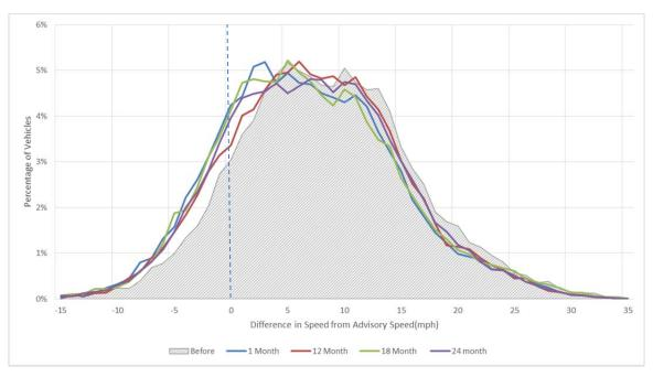
Figure EX.5. Percentage of vehicles with difference in speed from advisory speed at point of curvature (PC).
