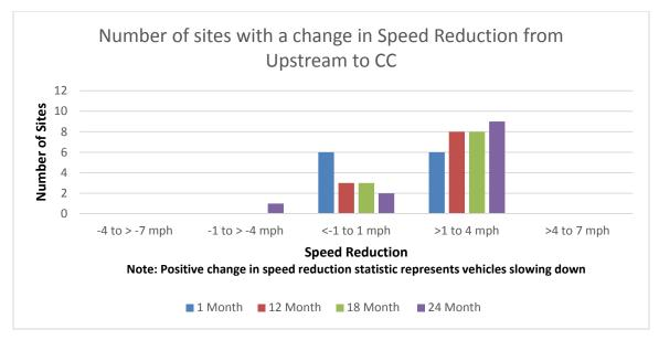
Figure 25. Graph. Number of sites with a change in speed reduction for tracked vehicles of a certain magnitude between the upstream and center of curve (CC).
