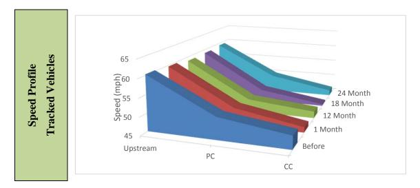
Figure 71. Graph. Speed profiles of tracked vehicles – Iowa Hwy 144.
