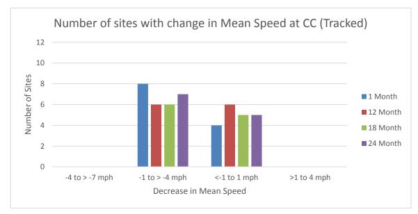
Figure 21. Graph. Number of sites with a change in mean speed for tracked vehicles of a certain magnitude at the center of curve (CC).
