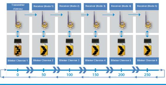
Sample Activation Timeline Programmable at any interval, to millisecond accuracy
