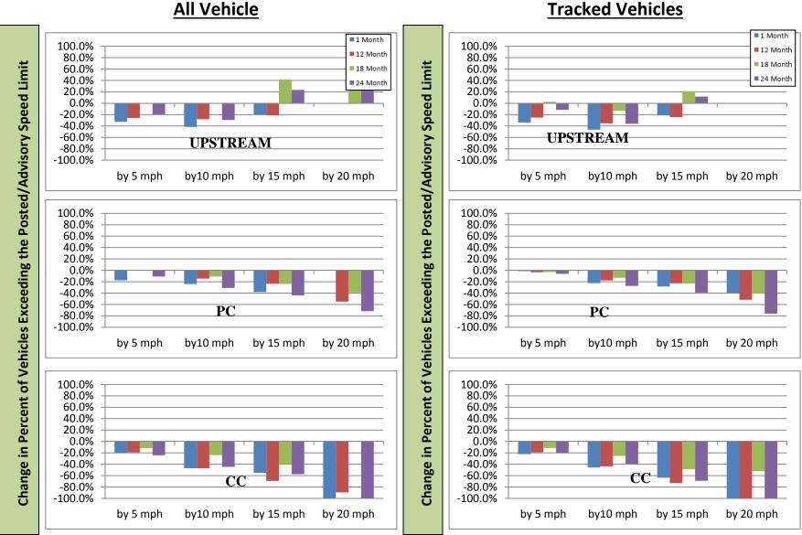
Figure 122. Graphs. Change in percentile (compared to before) of all vehicle speed - Texas FM 530.
