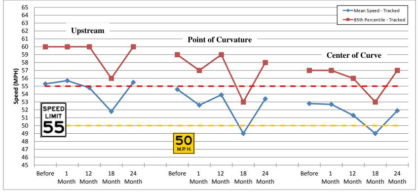
Figure 89. Graph. Impact on tracked vehicle speed - Washington SR 203.
