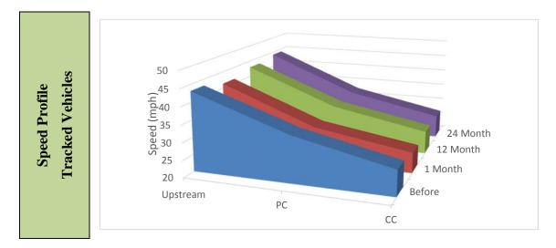
Figure 81. Graph . Speed profiles of tracked vehicles – Washington SR 7.
