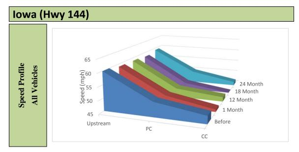
Figure 70. Graph. Speed profiles of all vehicles – Iowa Hwy 144.
