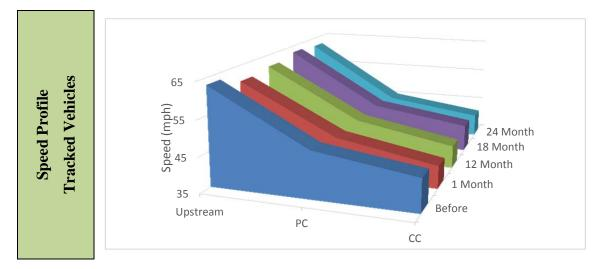
Figure 121. Graph. Speed profiles of tracked vehicles – Texas FM 530.
