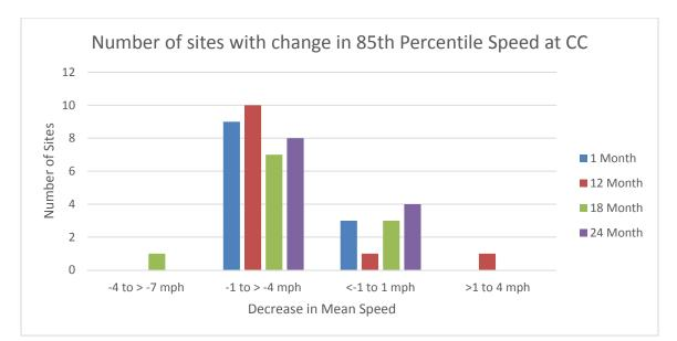
Figure 22. Graph. Number of sites with a change in 85<sup>th</sup> percentile speed for all vehicles of a certain magnitude at the center of curve (CC).
