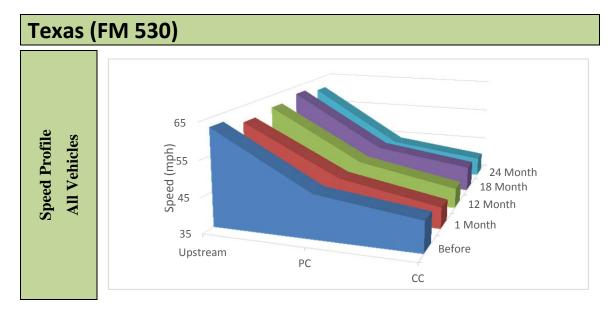
Figure 120. Graph. Speed profiles of tracked vehicles – Texas FM 530.
