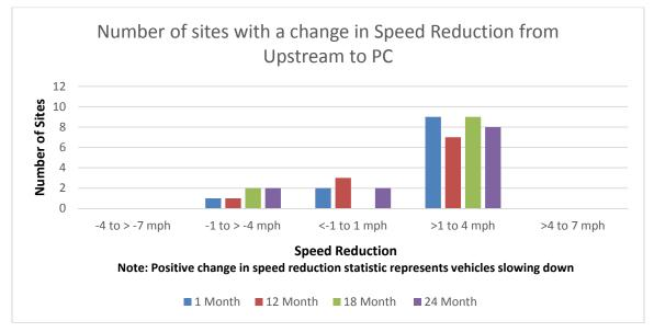
Figure 24. Graph. Number of sites with a change in speed reduction for tracked vehicles of a certain magnitude between the upstream and point of curvature (PC).
