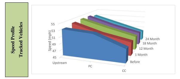
Figure 76. Graph Speed profiles of tracked vehicles – Missouri Hwy 221.
