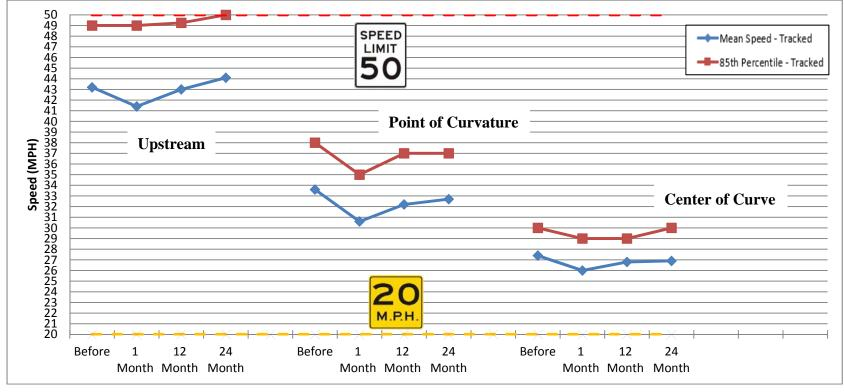
Figure 79. Graph. Impact on tracked vehicle speed - Washington SR 7.
