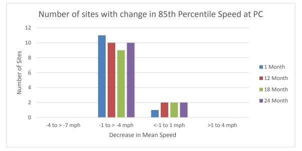
Figure 18. Graph. Number of sites with a change in 85<sup>th</sup> percentile speed for all vehicles of a certain magnitude at the point of curvature (PC).
