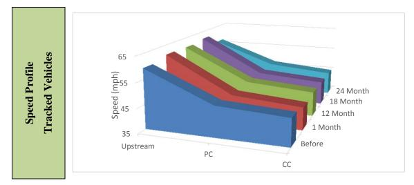
Figure 111. Graph. Speed profiles of tracked vehicles – Texas FM 109.
