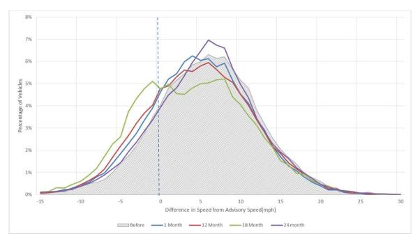
Figure EX7. Percentage of vehicles with difference in speed from advisory speed at center of curve (CC).
