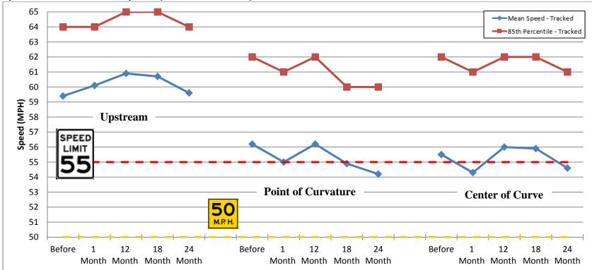
Figure 104. Graph. Impact on tracked vehicle speed - Wisconsin Hwy 213.
