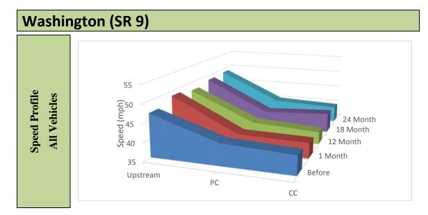
Figure 85. Graph. Speed profiles of all vehicles – Washington SR 9.
