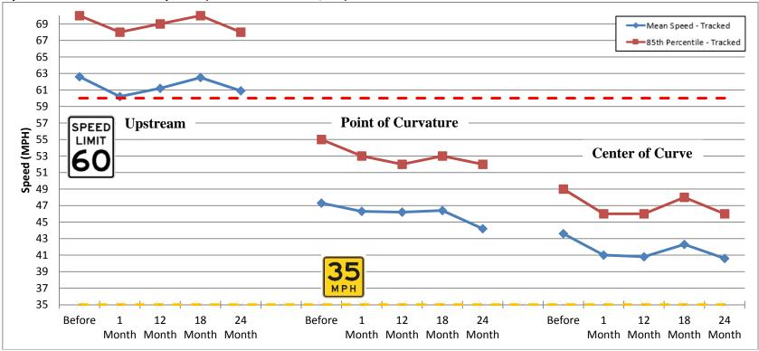
Figure 119. Graph. Impact on tracked vehicle speed - Texas FM 530.
