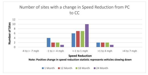
Figure 26. Graph. Number of sites with a change in speed reduction for tracked vehicles of a certain magnitude between the point of curvature (PC) and center of curve (CC).
