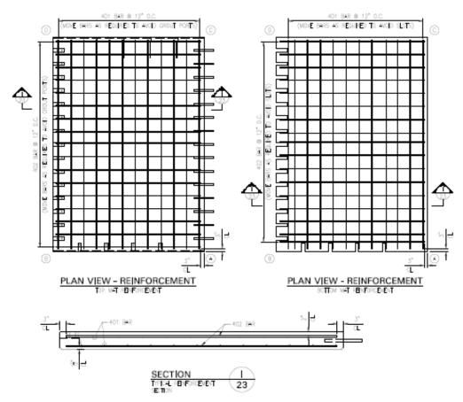
Figure 20. Diagram. Typical panel shop drawings (reinforcement details).
