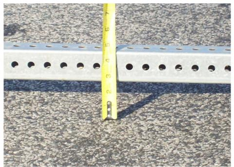
Figure 7. Photo. Rut depth measurement.
