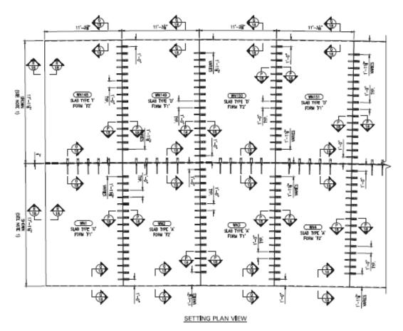
Figure 37. Diagram. Typical panel installation layout.
