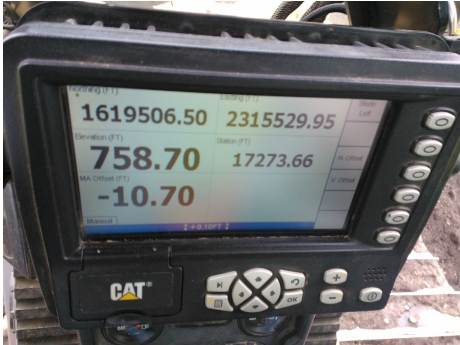
Figure 9. Photo. Screen showing the northing, easting, station, and offset parameters.
