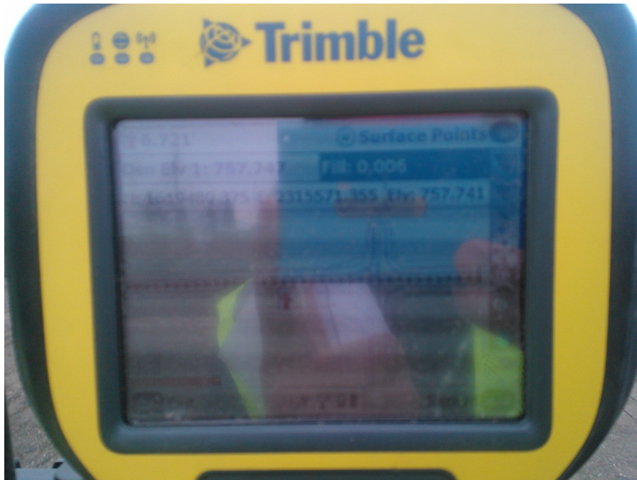
Figure 4. Photo. GPS survey rover screen indicating surface elevation and fill.
