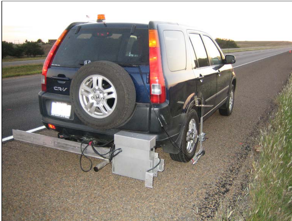
Figure 11. High-speed inertial profiler mounted behind the test vehicle.
