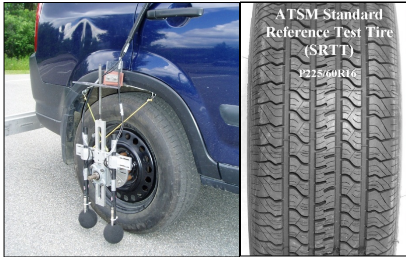
Figure 11. OBSI dual-probe system and the SRTT.
